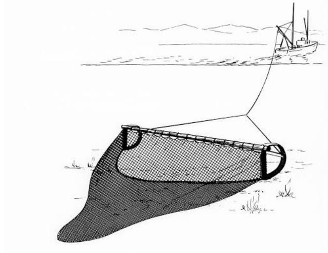
**Figure W-19. Schematic of a Beam Trawl** (Credit: FAO 2001)
