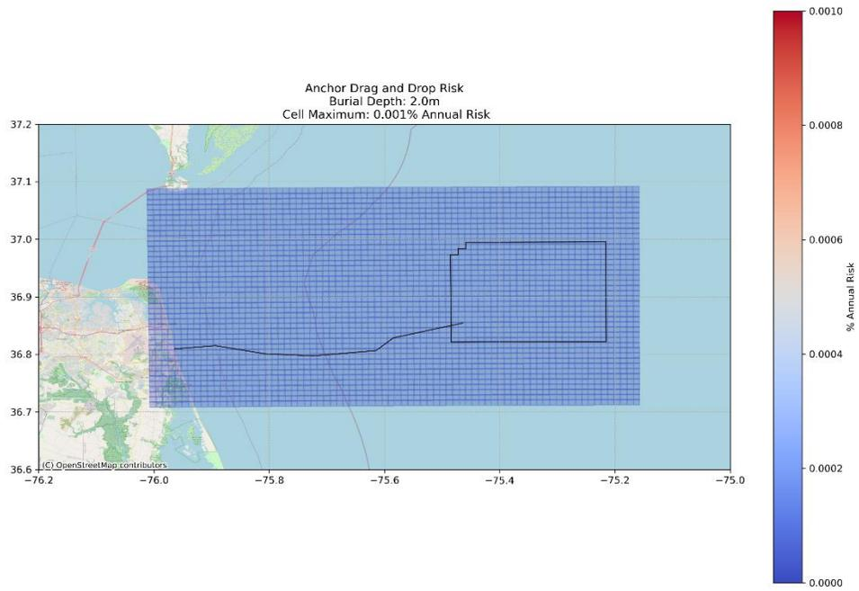
Figure W-59. Area Based Drag & Drop Anchoring Risk Chart, 6.6-ft (2.0-m) Burial Depth
