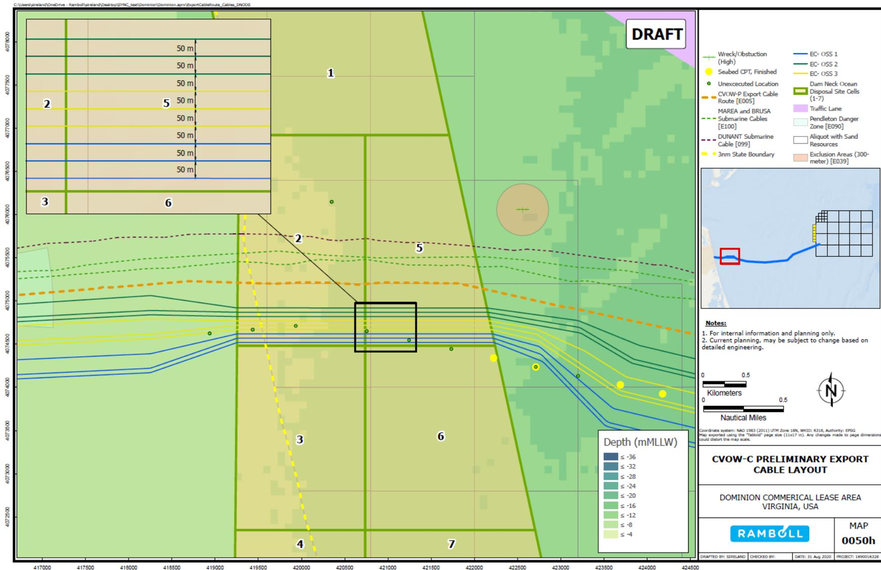
Figure W-31. Indicative Initial Layout of the Individual Export Cables where the Cables Cross the DNODS and Exhibit Decreased Spacing
