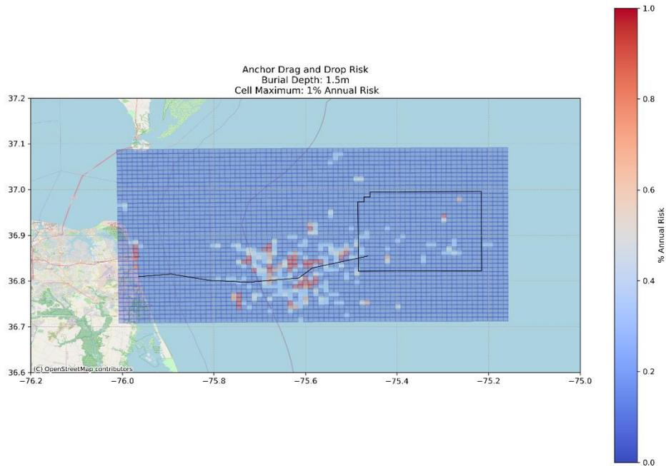
Figure W-58. Area Based Drag & Drop Anchoring Risk Chart, 5.0-ft (1.5-m) Burial Depth
