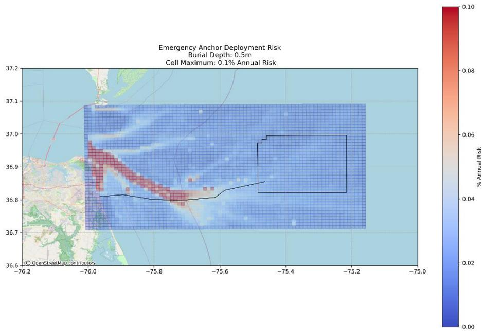
Figure W-51. Area Based Emergency Anchoring Risk Chart, 1.6-ft (0.5-m) Burial Depth
