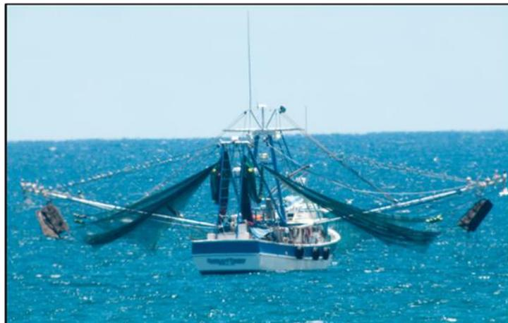
**Figure W-21. Double Rig Shrimp Trawl Vessel** (Photo Credit: Unknown)
