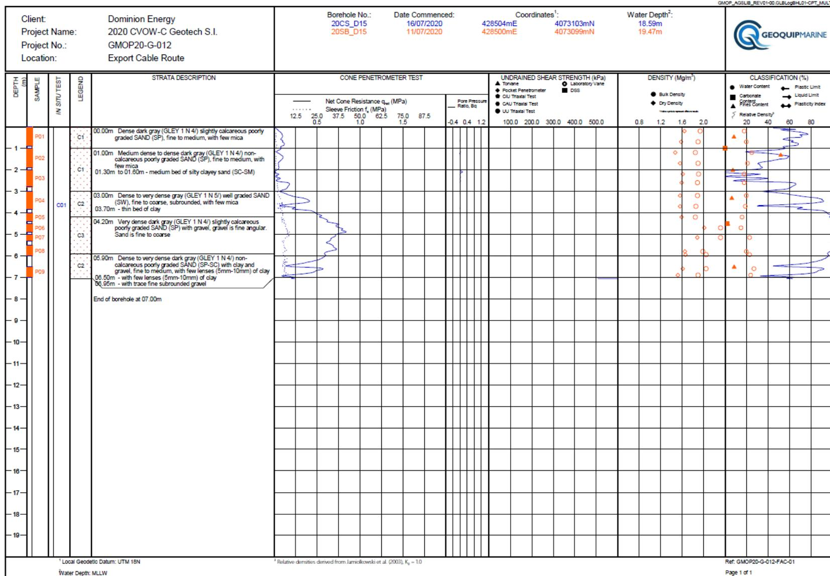
Figure W-11. CPT site 20CS\_D15 Shows Medium to Dense Sands in the Upper 1 to 2 m of the Seabed with some Finer Grained Materials Present
