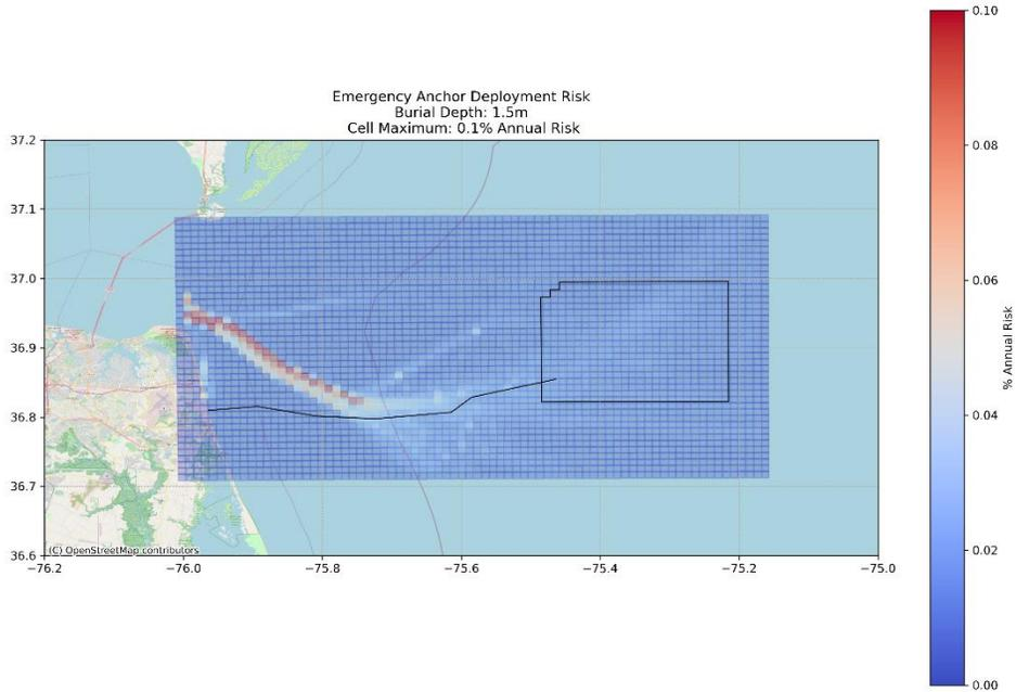
Figure W-53. Area Based Emergency Anchoring Risk Chart, 5.0-ft (1.5-m) Burial Depth
