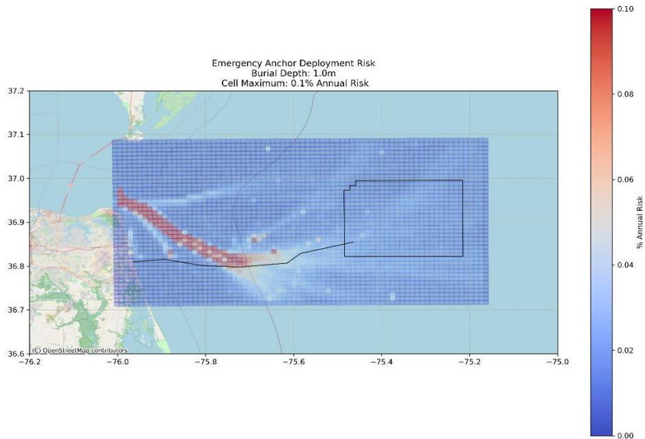
Figure W-52. Area Based Emergency Anchoring Risk Chart, 3.3-ft (1.0-m) Burial Depth
