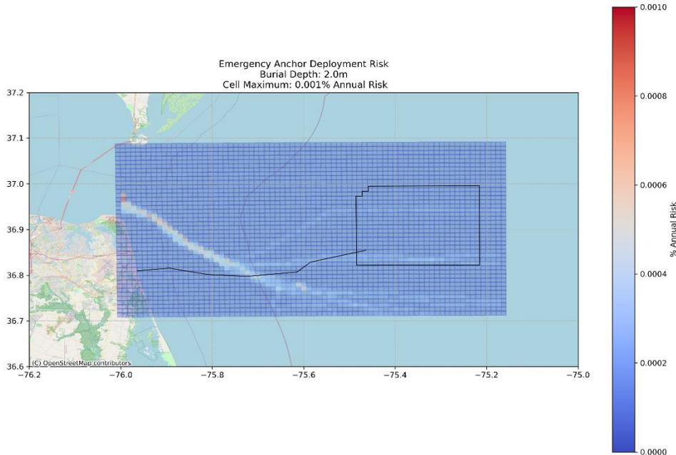
Figure W-54. Area Based Emergency Anchoring Risk Chart, 6.6-ft (2.0-m) Burial Depth
