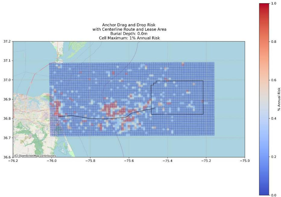
Figure W-55. Area Based Drag & Drop Anchoring Risk Chart, 0-m Burial Depth
