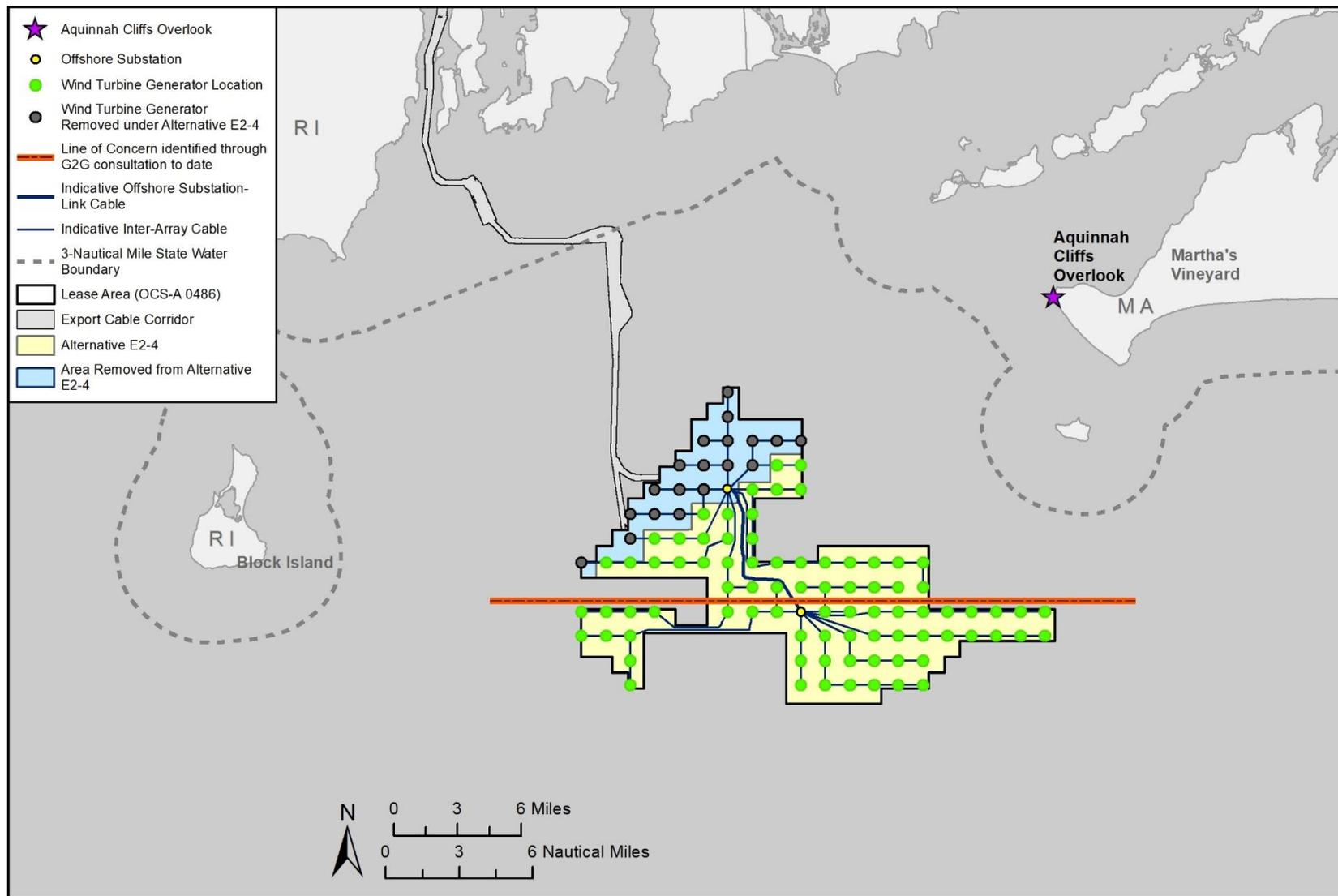
**Figure K-12. Layout Alternative E2-4. Gray shaded wind turbine generator positions in the blue field are those that would be eliminated from consideration. 880-megawatt maximum output; removal of 23 wind turbine generator positions (leaves 77 positions available).**
