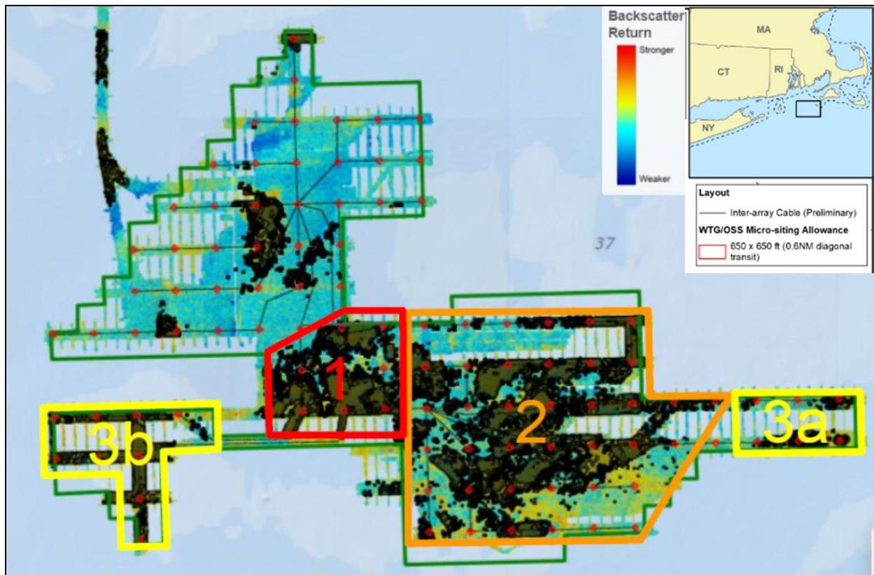
**Figure K-1. Alternative C development. Revolution Wind Lease Area with multi-beam backscatter and boulder presence (dark green with black outlines; data from construction and operations plan Appendix X2) shown in relation to the four priority areas identified for avoidance by the Greater Atlantic Regional Fisheries Office on November 5, 2021.**
