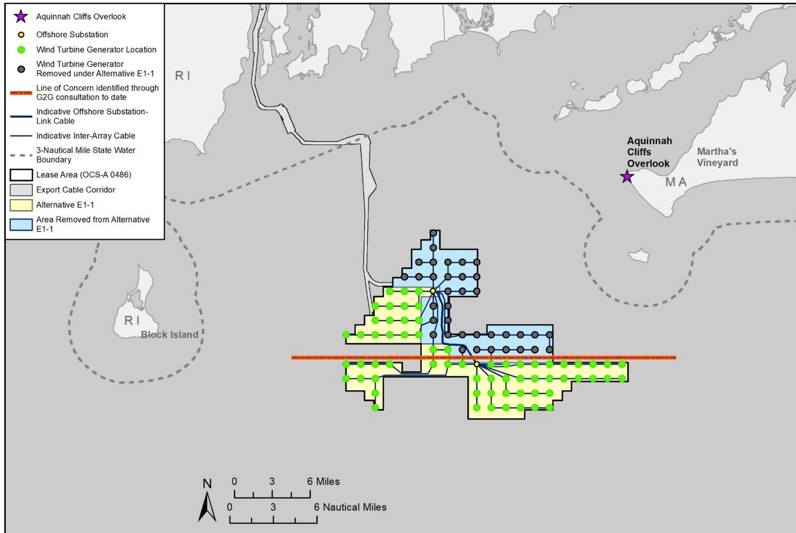
**Figure K-5. Layout Alternative E1-1. Gray shaded wind turbine generator positions in the blue field are those that would be eliminated from consideration. 704-megawatt maximum output; removal of 36 wind turbine generator positions (leaves 64 positions available).**
