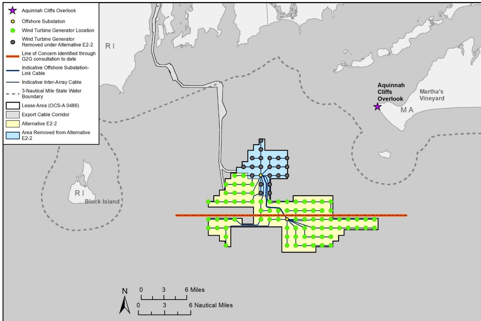
**Figure K-10. Layout Alternative E2-2. Gray shaded wind turbine generator positions in the blue field are those that would be eliminated from consideration. 880-megawatt maximum output; removal of 21 wind turbine generator positions (leaves 79 positions available).**
