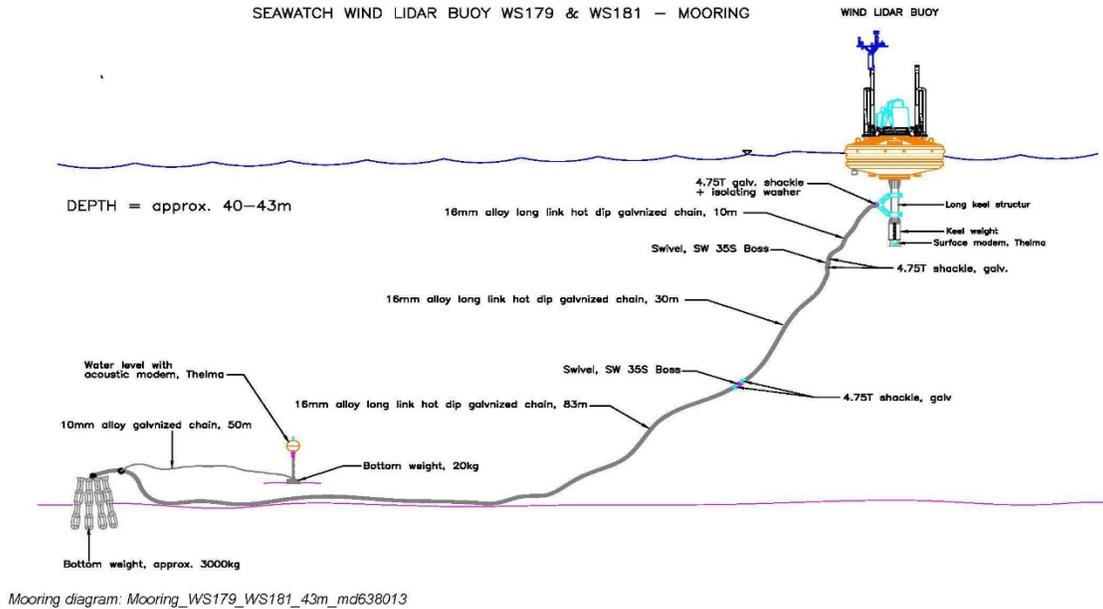
**Figure 2. Illustration of a meteorological buoy and mooring configuration (Vineyard Wind SAP 2020); Vineyard Wind may deploy up to two of buoys at areas SAP-1 and SAP-2.**
