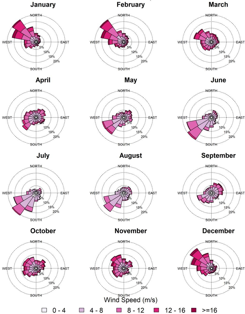
Figure A-6. Monthly CFSR wind roses in the vicinity of the booster station. Wind speeds in m/s, using meteorological convention (i.e., direction wind is coming from)
