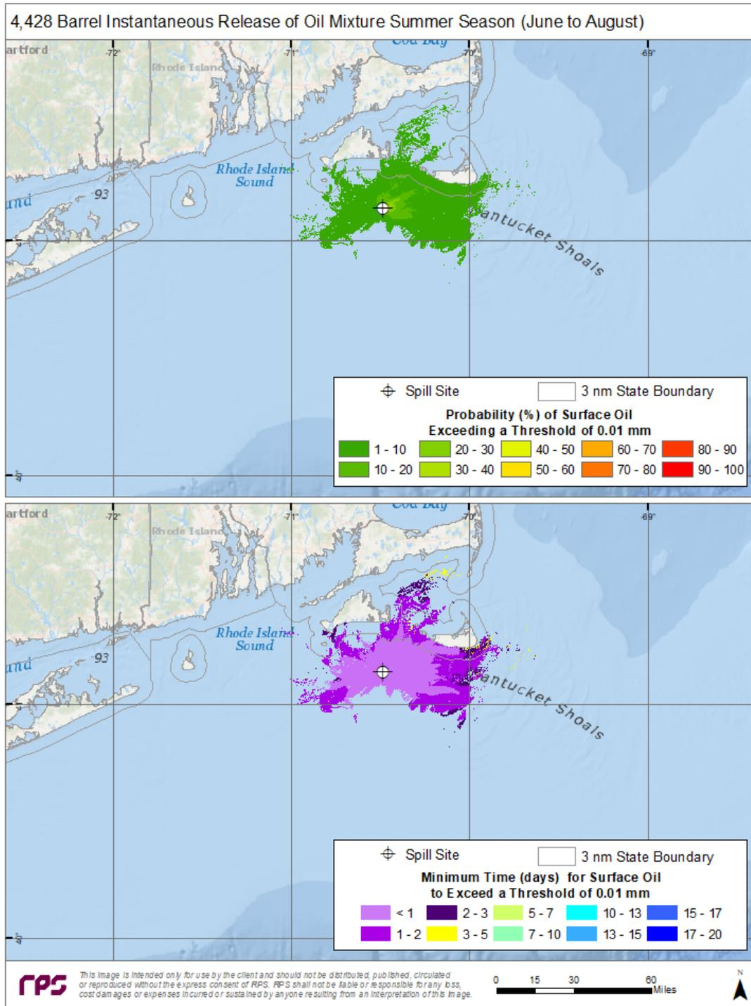
Figure A-19. Detail View. Top Panel—Probability of surface oiling above a minimum thickness of 10  $\mu\text{m}$  (10  $\text{g}/\text{m}^2$  on average over the grid cell) during summer months for an instantaneous discharge from the potential booster station. Bottom Panel—Minimum time for surface oiling to occur at thicknesses greater than 10  $\text{g}/\text{m}^2$ .
