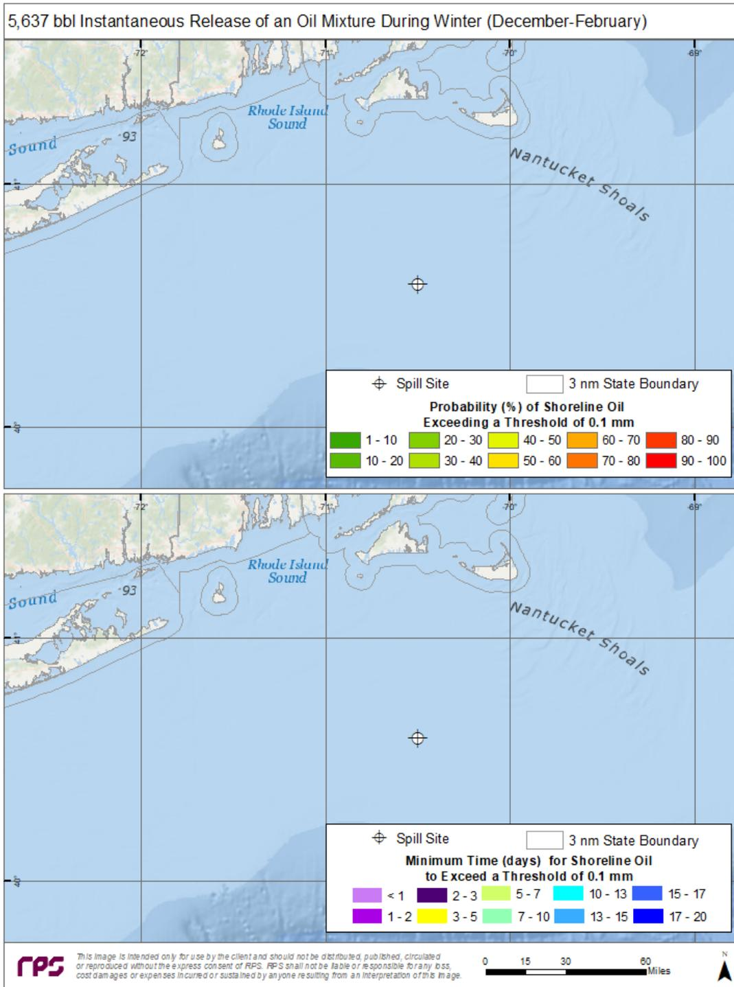
Figure 43. Top Panel—Probability of shoreline oiling above a minimum thickness of 100  $\mu\text{m}$  (100  $\text{g}/\text{m}^2$  on average over the grid cell) during winter months for an instantaneous discharge from the ESP 2 location. Bottom Panel—Minimum time for shoreline oiling to occur at thicknesses greater than 100  $\text{g}/\text{m}^2$ .
