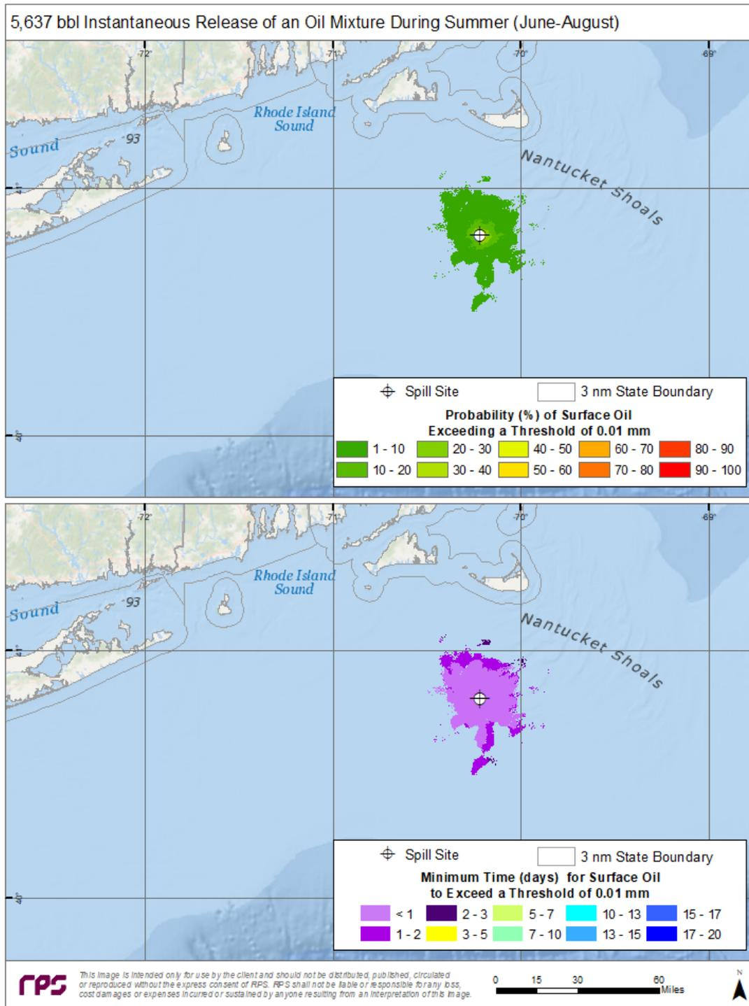
Figure 29. Top Panel—Probability of surface oiling above a minimum thickness of 10  $\mu\text{m}$  (10  $\text{g}/\text{m}^2$  on average over the grid cell) during summer months for an instantaneous discharge from the ESP 1 location. Bottom Panel—Minimum time for surface oiling to occur at thicknesses greater than 10  $\text{g}/\text{m}^2$ .
