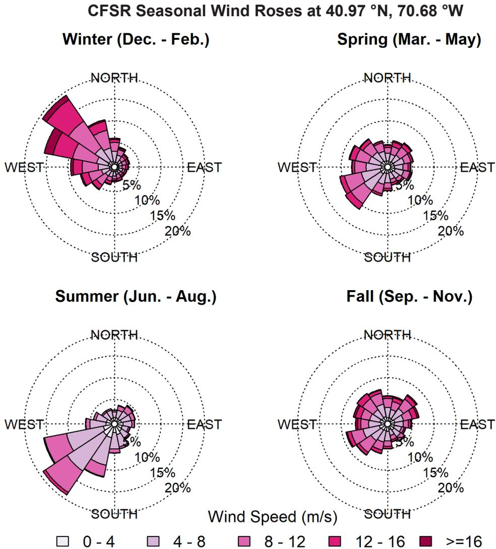
Figure A-7. Seasonal CFSR wind roses in the vicinity of the booster station. Wind speeds in m/s, using meteorological convention (i.e., direction wind is coming from).
