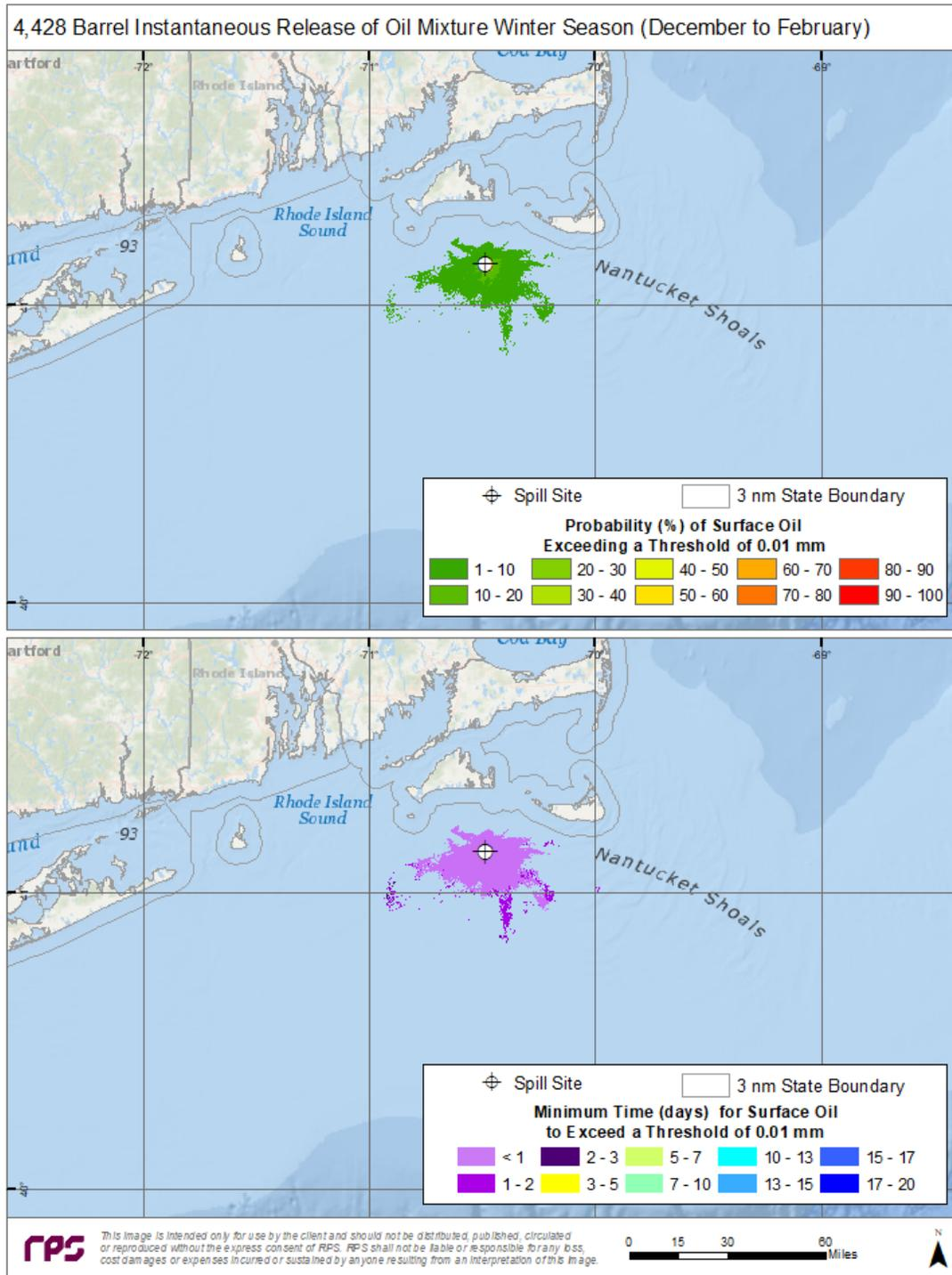
**Figure A-23. Detail View. Top Panel—Probability of surface oiling above a minimum thickness of 10  $\mu$ m (10 g/m<sup>2</sup> on average over the grid cell) during winter months for an instantaneous discharge from the potential booster station. Bottom Panel—Minimum time for surface oiling to occur at thicknesses greater than 10 g/m<sup>2</sup>.**
