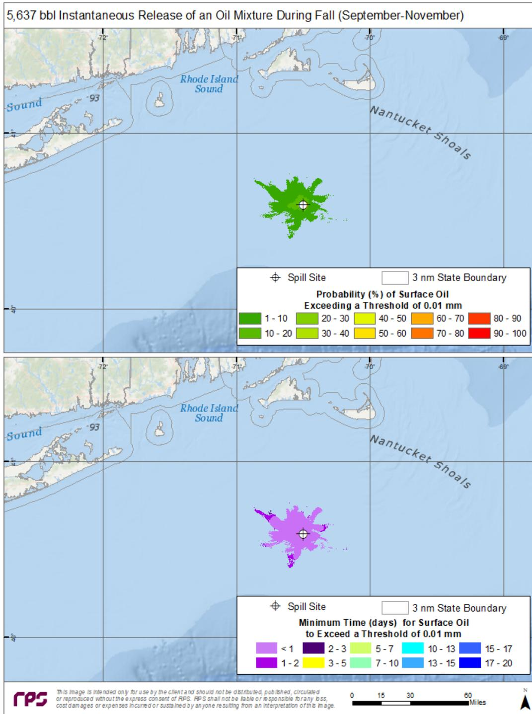
Figure 38. Top Panel—Probability of surface oiling above a minimum thickness of 10  $\mu\text{m}$  (10  $\text{g}/\text{m}^2$  on average over the grid cell) during fall months for an instantaneous discharge from the ESP 2 location. Bottom Panel—Minimum time for surface oiling to occur at thicknesses greater than 10  $\text{g}/\text{m}^2$ .
