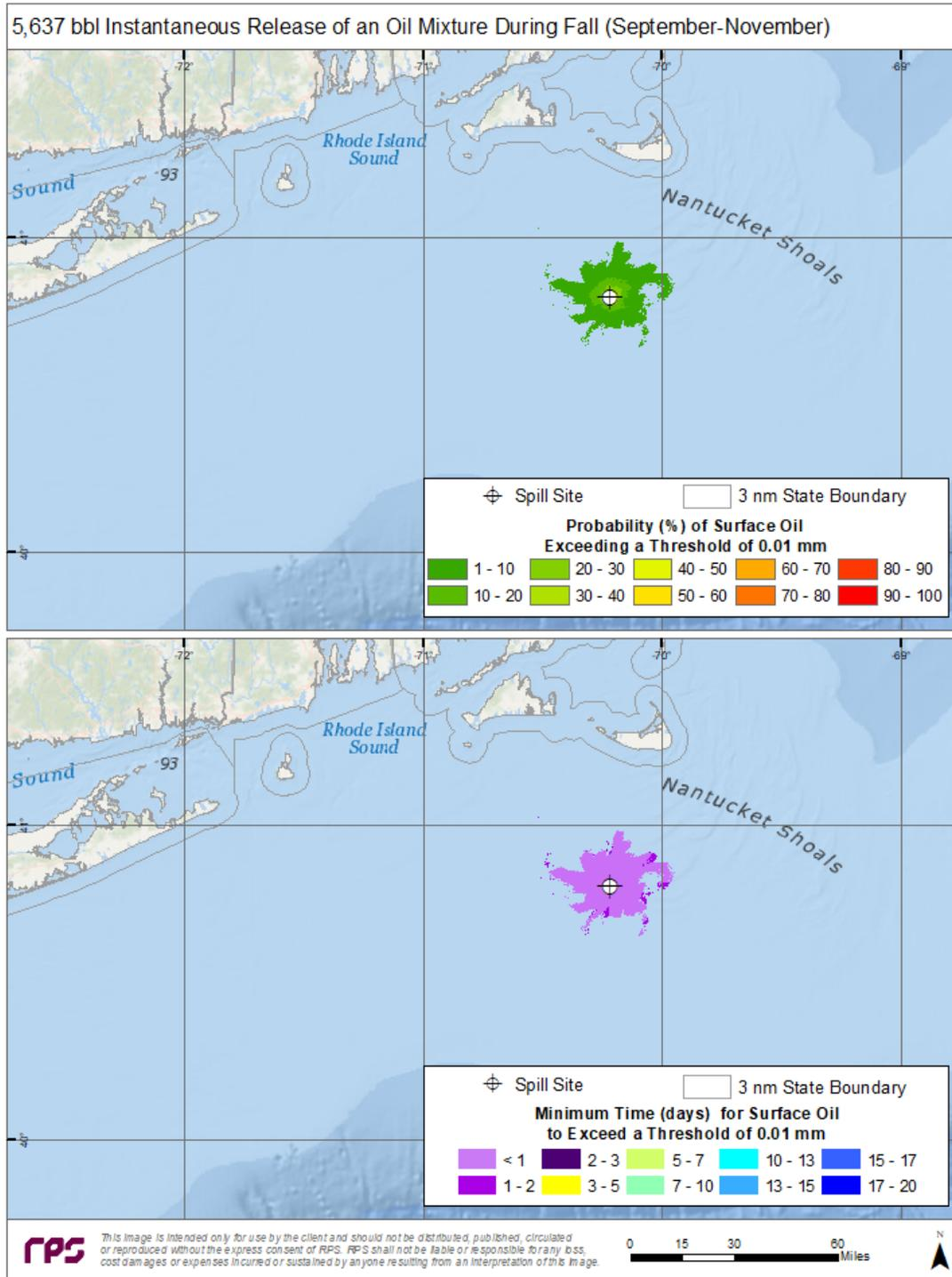
Figure 30. Top Panel—Probability of surface oiling above a minimum thickness of 10  $\mu\text{m}$  (10  $\text{g}/\text{m}^2$  on average over the grid cell) during fall months for an instantaneous discharge from the ESP 1 location. Bottom Panel—Minimum time for surface oiling to occur at thicknesses greater than 10  $\text{g}/\text{m}^2$ .
