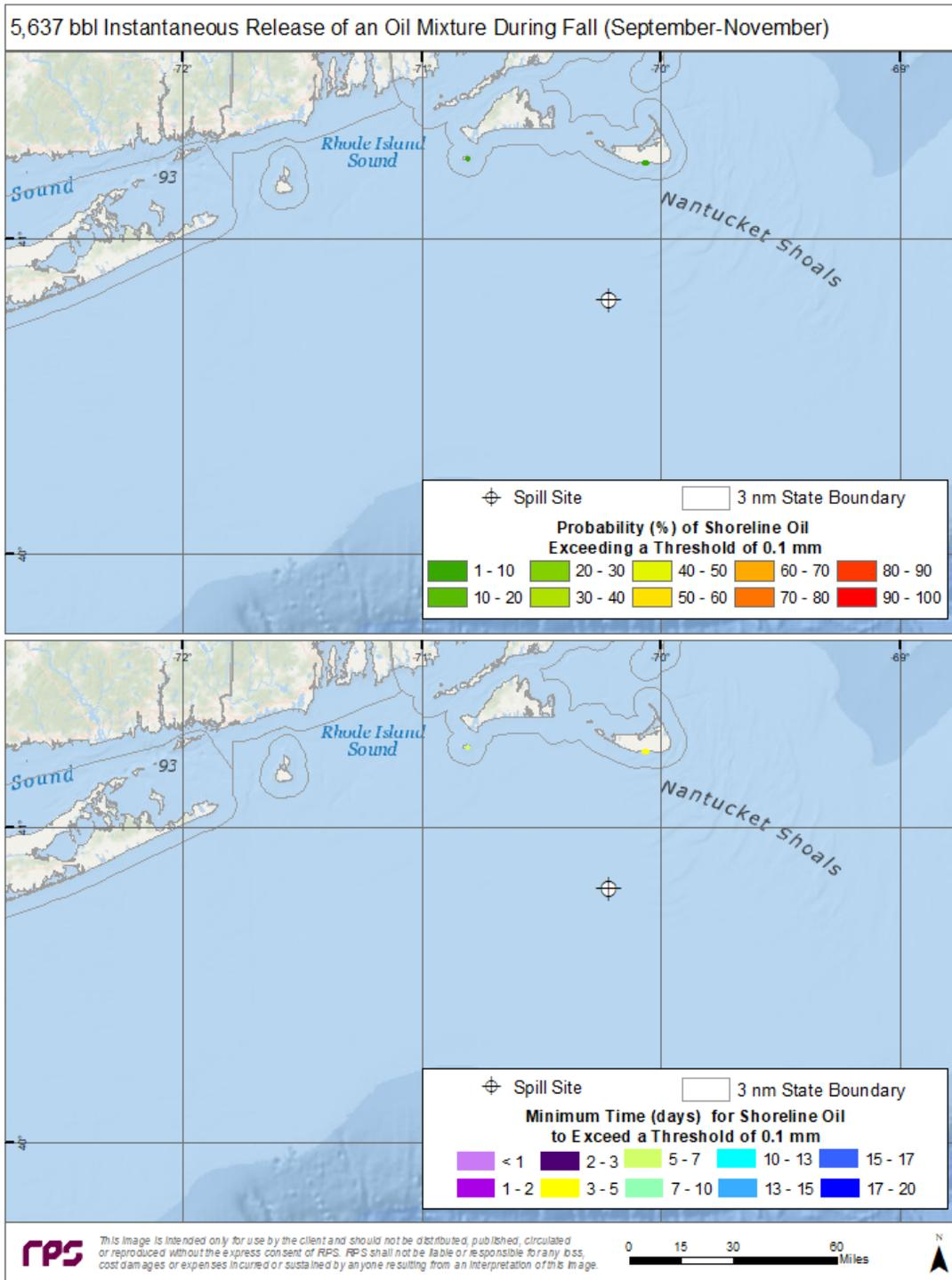
Figure 34. Top Panel—Probability of shoreline oiling above a minimum thickness of 100  $\mu\text{m}$  (100  $\text{g}/\text{m}^2$  on average over the grid cell) during fall months for an instantaneous discharge from the ESP 1 location. Bottom Panel—Minimum time for shoreline oiling to occur at thicknesses greater than 100  $\text{g}/\text{m}^2$ .
