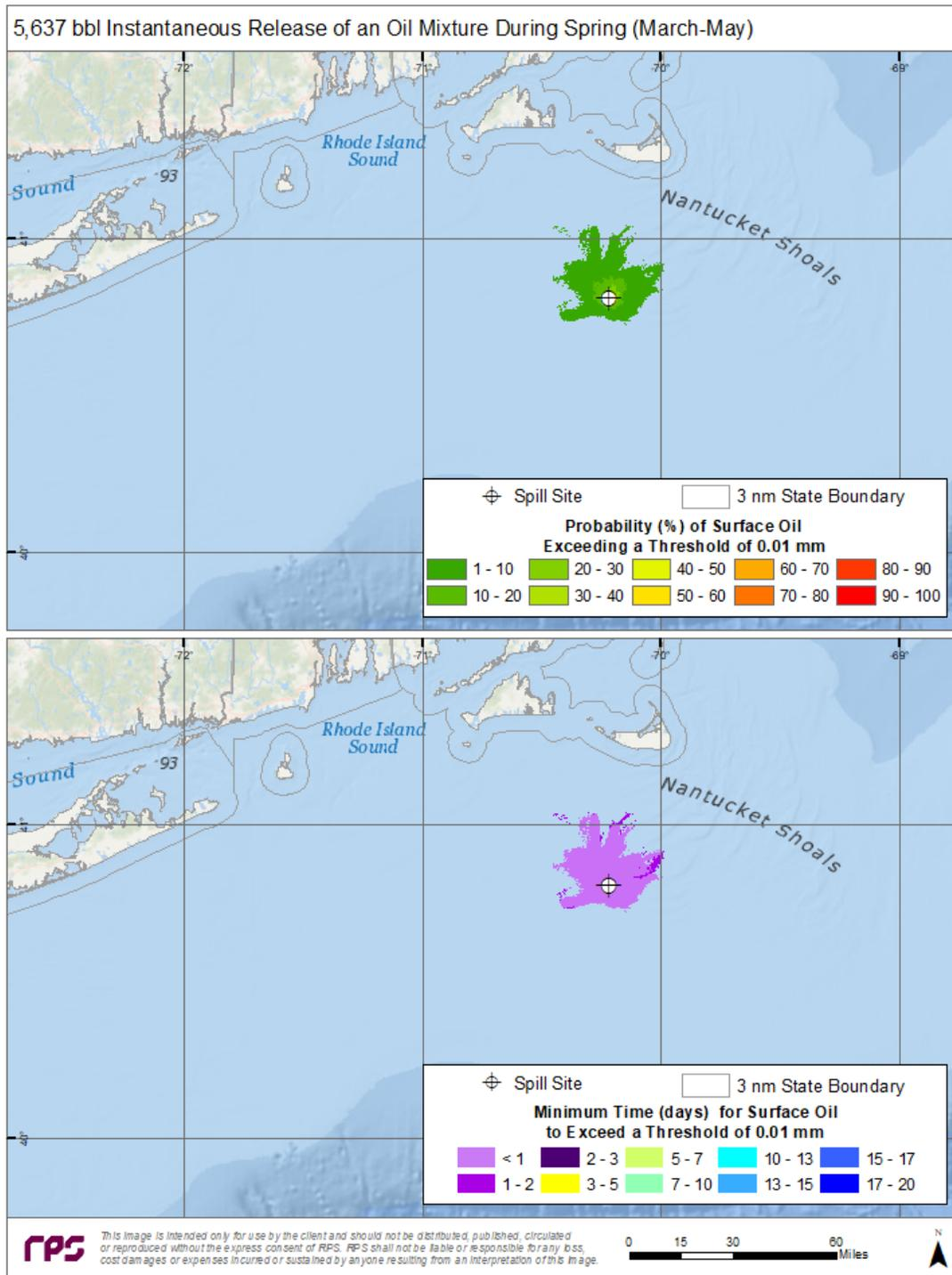
Figure 28. Top Panel—Probability of surface oiling above a minimum thickness of 10  $\mu\text{m}$  (10  $\text{g}/\text{m}^2$  on average over the grid cell) during spring months for an instantaneous discharge from the ESP 1 location. Bottom Panel—Minimum time for surface oiling to occur at thicknesses greater than 10  $\text{g}/\text{m}^2$ .
