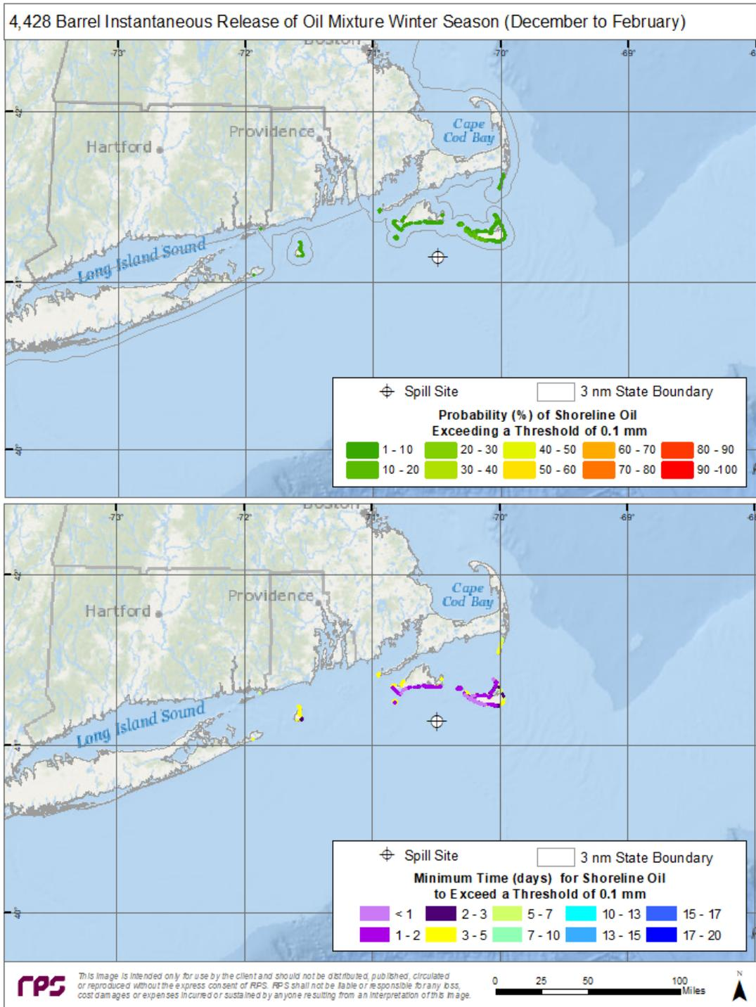
Figure A-27. Top Panel—Probability of shoreline oiling above a minimum thickness of 100  $\mu\text{m}$  (100  $\text{g}/\text{m}^2$  on average over the grid cell) during winter months for an instantaneous discharge from the potential booster station. Bottom Panel—Minimum time for shoreline oiling to occur at thicknesses greater than 100  $\text{g}/\text{m}^2$ .
