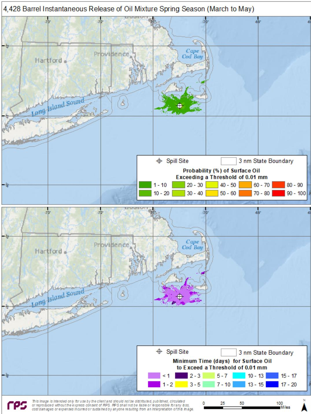
**Figure A-16. Top Panel—Probability of surface oiling above a minimum thickness of 10  $\mu\text{m}$  (10  $\text{g}/\text{m}^2$  on average over the grid cell) during spring months for an instantaneous discharge from the potential booster station. Bottom Panel—Minimum time for surface oiling to occur at thicknesses greater than 10  $\text{g}/\text{m}^2$ .**
