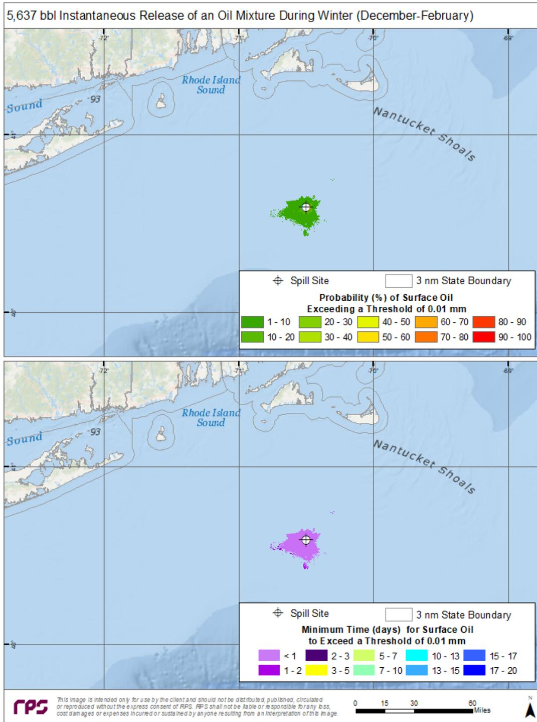
Figure 39. Top Panel—Probability of surface oiling above a minimum thickness of 10  $\mu\text{m}$  (10  $\text{g}/\text{m}^2$  on average over the grid cell) during winter months for an instantaneous discharge from the ESP 2 location. Bottom Panel—Minimum time for surface oiling to occur at thicknesses greater than 10  $\text{g}/\text{m}^2$ .
