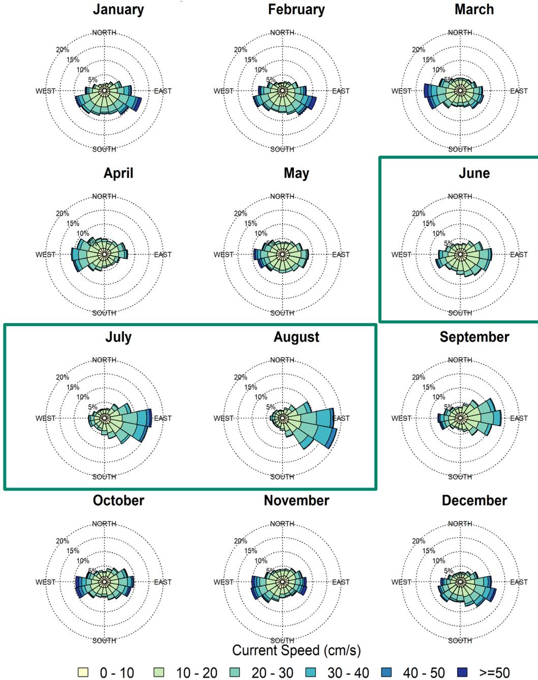
Figure A-12. Monthly HYCOM+HYDROMAP current roses in the vicinity of the booster station. Current speeds in cm/s, using oceanographic convention (direction currents are heading towards). The green box highlights summer.
