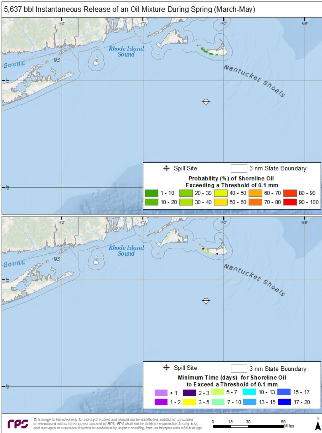
Figure 32. Top Panel—Probability of shoreline oiling above a minimum thickness of 100  $\mu\text{m}$  (100  $\text{g}/\text{m}^2$  on average over the grid cell) during spring months for an instantaneous discharge from the ESP 1 location. Bottom Panel—Minimum time for shoreline oiling to occur at thicknesses greater than 100  $\text{g}/\text{m}^2$ .
