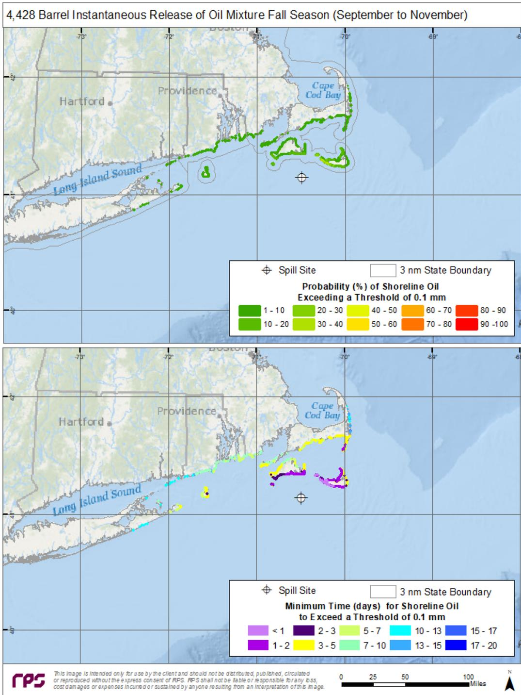
Figure A-26. Top Panel—Probability of shoreline oiling above a minimum thickness of 100  $\mu\text{m}$  (100  $\text{g}/\text{m}^2$  on average over the grid cell) during fall months for an instantaneous discharge from the potential booster station. Bottom Panel—Minimum time for shoreline oiling to occur at thicknesses greater than 100  $\text{g}/\text{m}^2$ .
