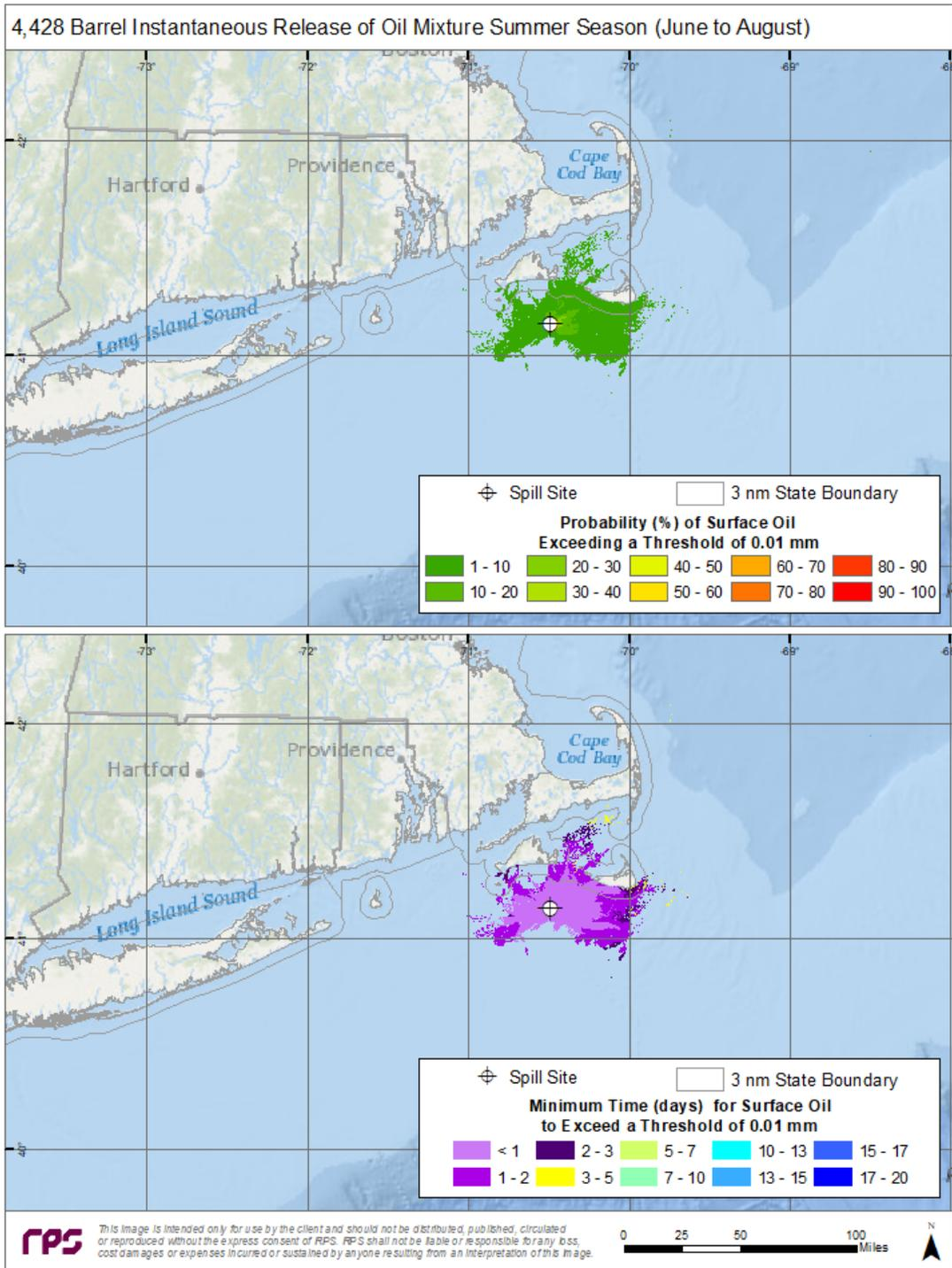
Figure A-18. Top Panel—Probability of surface oiling above a minimum thickness of 10  $\mu\text{m}$  (10  $\text{g}/\text{m}^2$  on average over the grid cell) during summer months for an instantaneous discharge from the potential booster station. Bottom Panel—Minimum time for surface oiling to occur at thicknesses greater than 10  $\text{g}/\text{m}^2$ .
