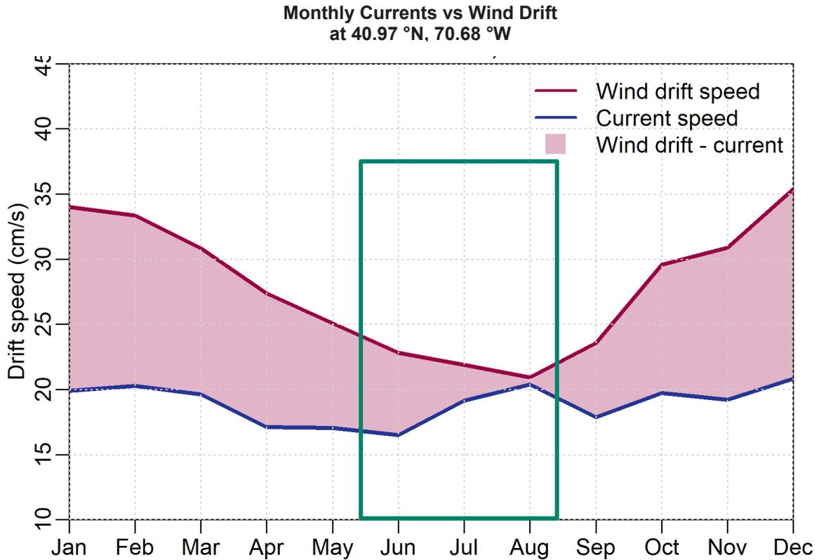
Figure A-14. Surface drift forcing comparison statistics in the vicinity of the booster station: monthly-averaged CSFR wind drift compared with HYCOM+HYDROMAP current speed. Wind drift is calculated as 3.5% of the wind speed. Periods with predominant wind transport are shaded pink. The green box highlights summer.
