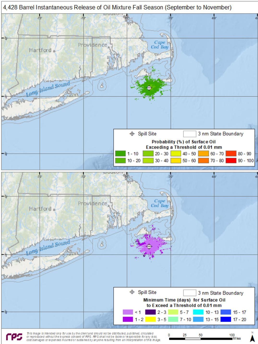
Figure A-20. Top Panel—Probability of surface oiling above a minimum thickness of 10  $\mu\text{m}$  (10  $\text{g}/\text{m}^2$  on average over the grid cell) during fall months for an instantaneous discharge from the potential booster station. Bottom Panel—Minimum time for surface oiling to occur at thicknesses greater than 10  $\text{g}/\text{m}^2$ .
