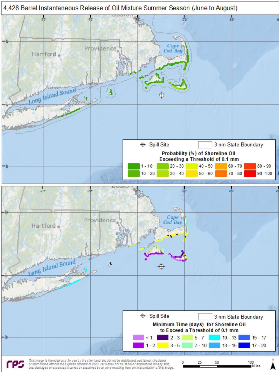
Figure A-25. Top Panel—Probability of shoreline oiling above a minimum thickness of 100  $\mu\text{m}$  (100  $\text{g}/\text{m}^2$  on average over the grid cell) during summer months for an instantaneous discharge from the potential booster station. Bottom Panel—Minimum time for shoreline oiling to occur at thicknesses greater than 100  $\text{g}/\text{m}^2$ .
