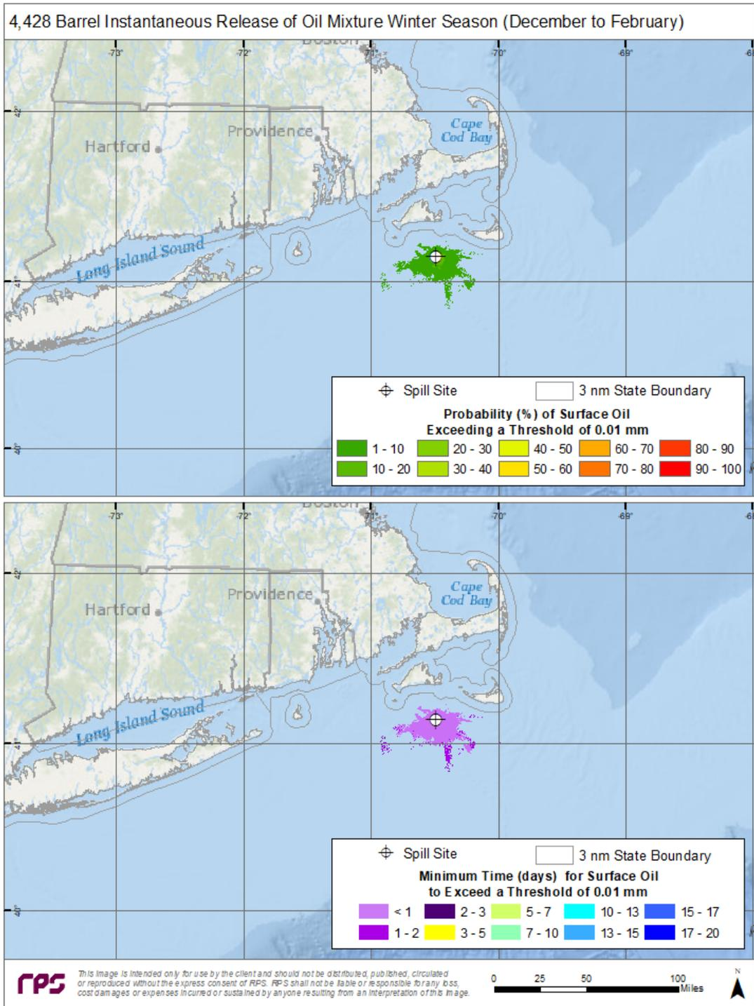
Figure A-22. Top Panel—Probability of surface oiling above a minimum thickness of 10  $\mu\text{m}$  (10  $\text{g}/\text{m}^2$  on average over the grid cell) during winter months for an instantaneous discharge from the potential booster station. Bottom Panel—Minimum time for surface oiling to occur at thicknesses greater than 10  $\text{g}/\text{m}^2$ .
