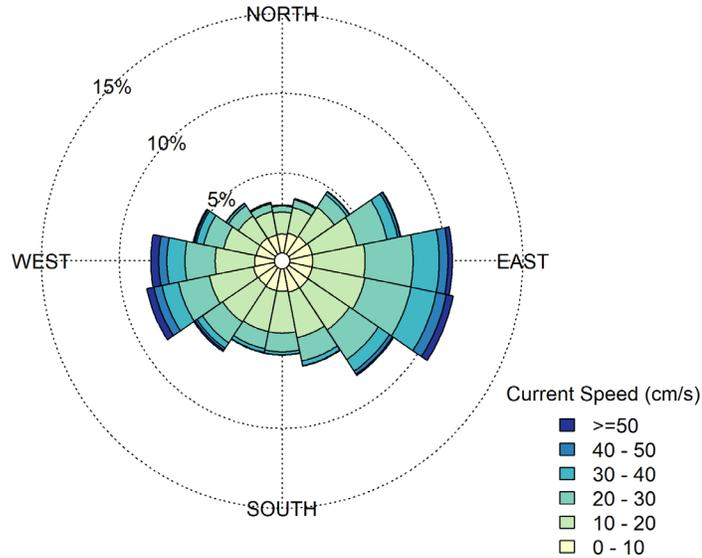
Figure A-10. Annual HYCOM+HYDROMAP surface current rose in the vicinity of the booster station following oceanographic convention (direction currents are heading towards). Current speeds are in cm/s.
