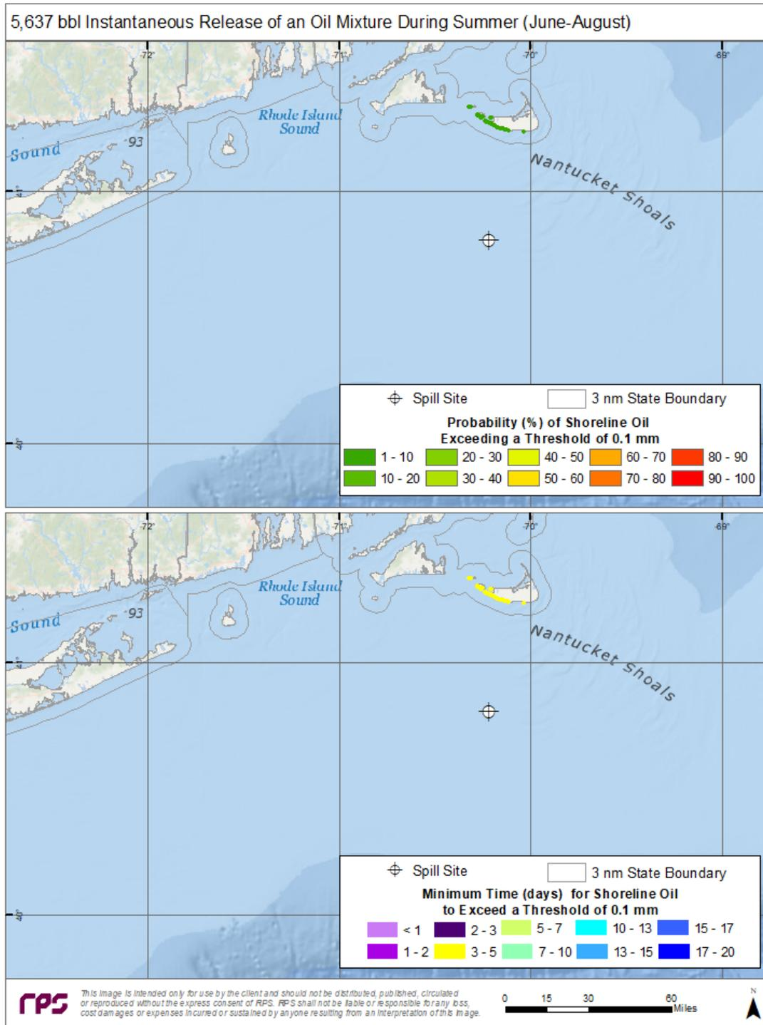
Figure 33. Top Panel—Probability of shoreline oiling above a minimum thickness of 100  $\mu\text{m}$  (100  $\text{g}/\text{m}^2$  on average over the grid cell) during summer months for an instantaneous discharge from the ESP 1 location. Bottom Panel—Minimum time for shoreline oiling to occur at thicknesses greater than 100  $\text{g}/\text{m}^2$ .
