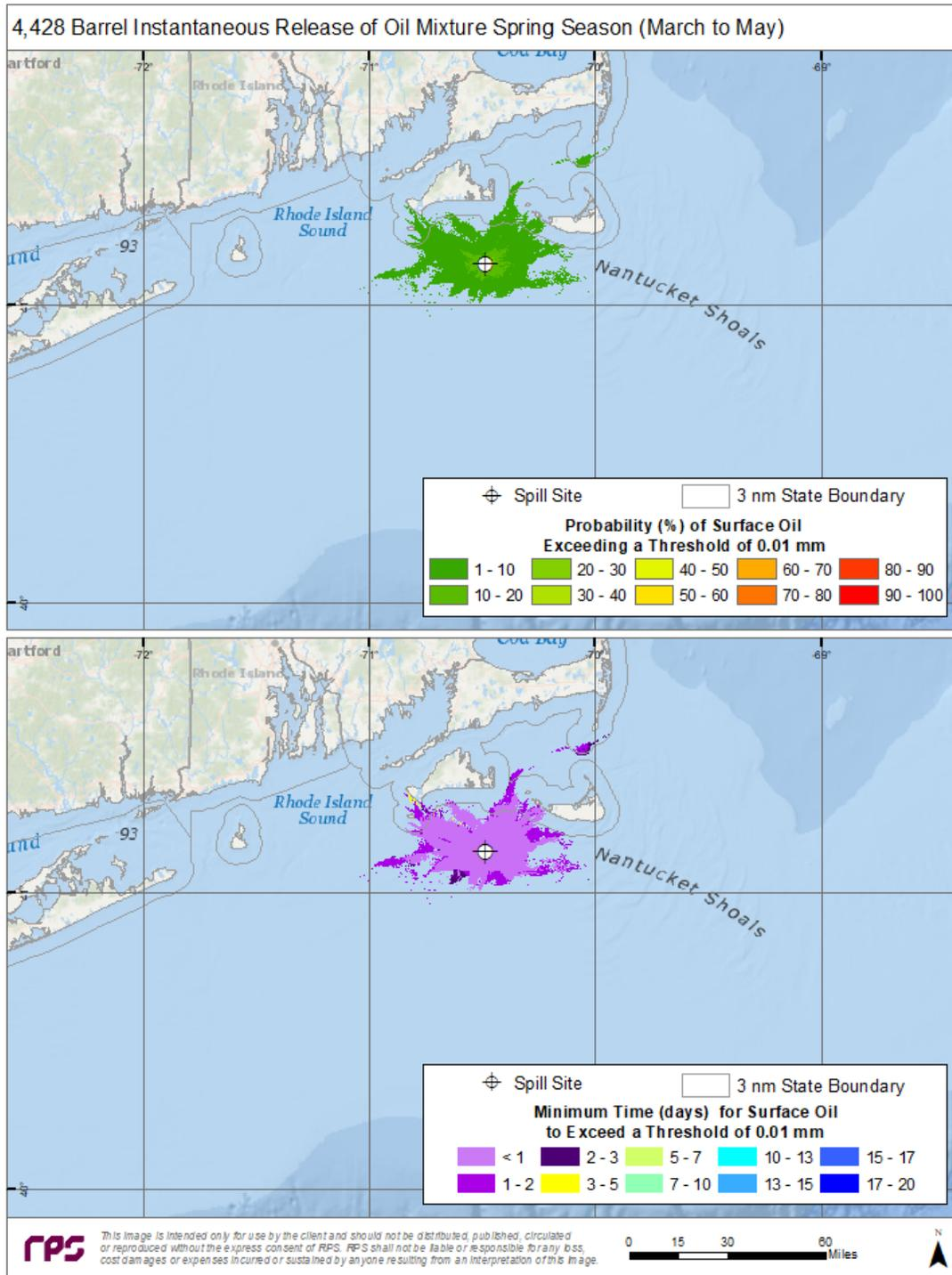
**Figure A-17. Detail View. Top Panel—Probability of surface oiling above a minimum thickness of 10  $\mu\text{m}$  (10  $\text{g}/\text{m}^2$  on average over the grid cell) during spring months for an instantaneous discharge from the potential booster station. Bottom Panel—Minimum time for surface oiling to occur at thicknesses greater than 10  $\text{g}/\text{m}^2$ .**
