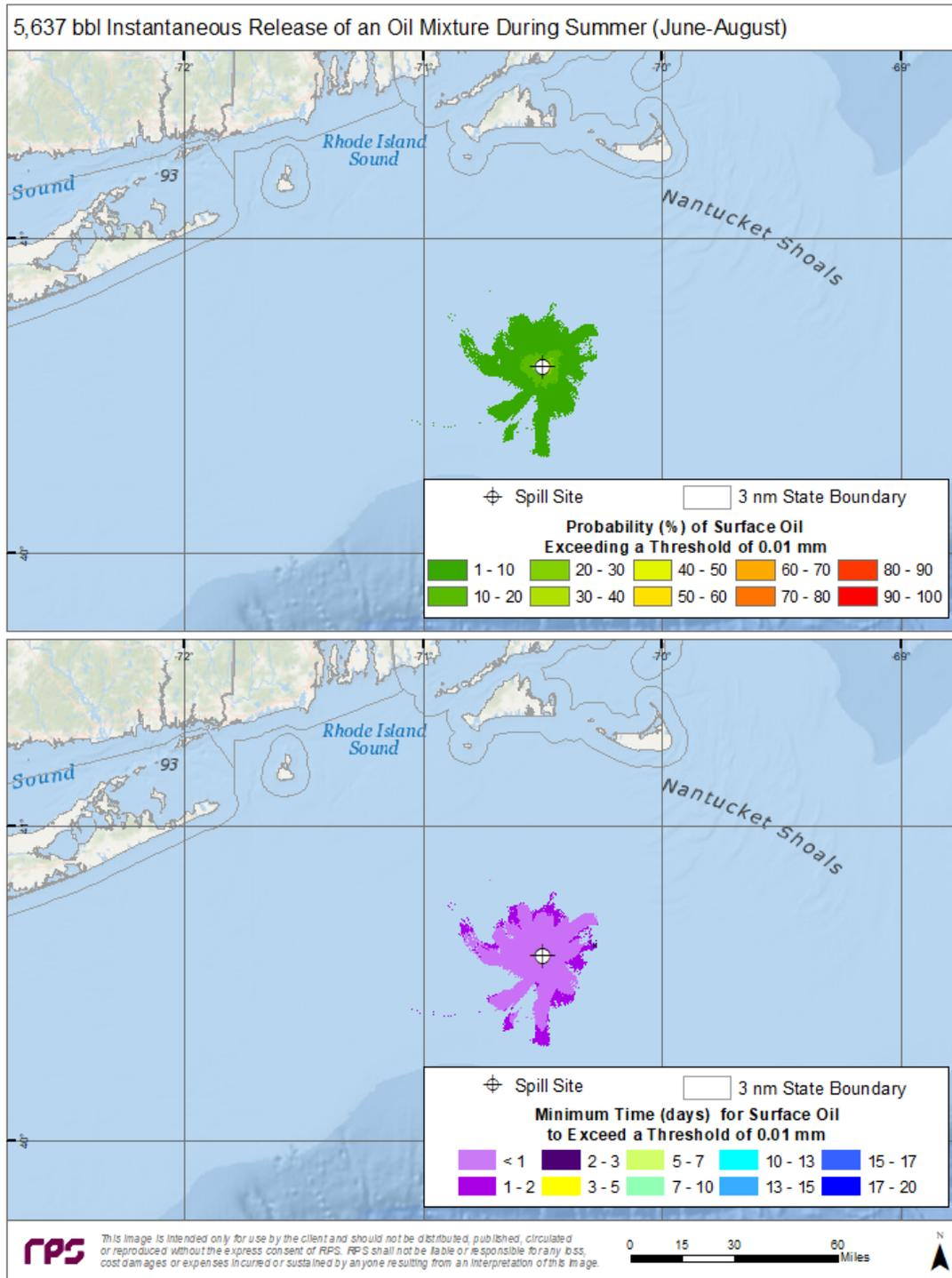
Figure 37. Top Panel—Probability of surface oiling above a minimum thickness of 10  $\mu\text{m}$  (10  $\text{g}/\text{m}^2$  on average over the grid cell) during summer months for an instantaneous discharge from the ESP 2 location. Bottom Panel—Minimum time for surface oiling to occur at thicknesses greater than 10  $\text{g}/\text{m}^2$ .
