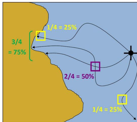
Figure 27. Example illustration of the difference between surface and shoreline oiling probabilities. Surface probabilities in yellow and purple, shoreline probabilities in green.
