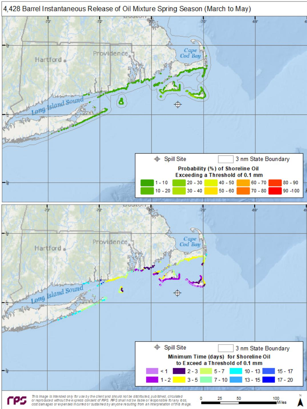
Figure A-24. Top Panel—Probability of shoreline oiling above a minimum thickness of 100  $\mu\text{m}$  (100  $\text{g}/\text{m}^2$  on average over the grid cell) during spring months for an instantaneous discharge from the potential booster station. Bottom Panel—Minimum time for shoreline oiling to occur at thicknesses greater than 100  $\text{g}/\text{m}^2$ .
