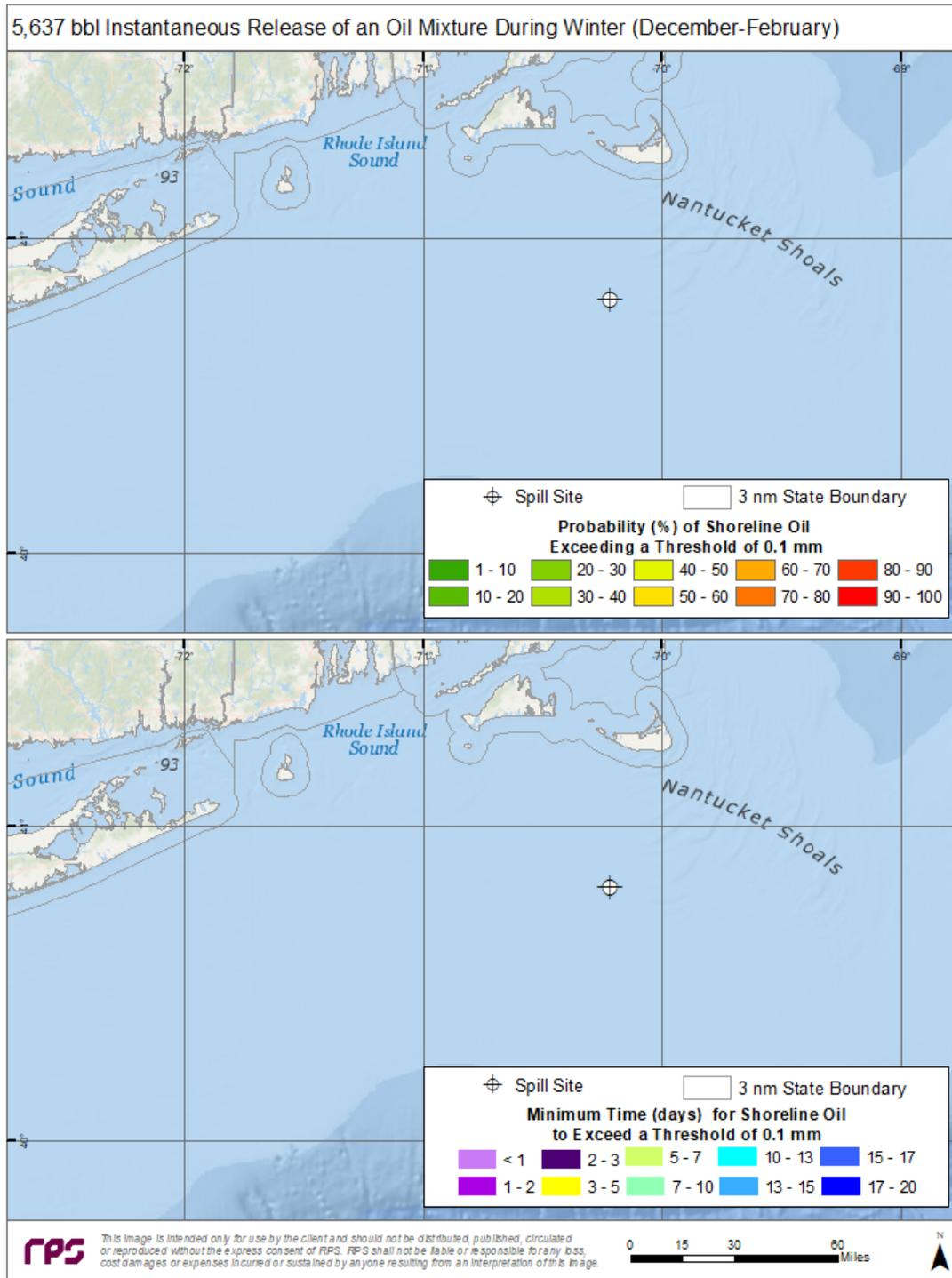
Figure 35. Top Panel—Probability of shoreline oiling above a minimum thickness of 100  $\mu\text{m}$  ( $100 \text{ g/m}^2$  on average over the grid cell) during winter months for an instantaneous discharge from the ESP 1 location. Bottom Panel—Minimum time for shoreline oiling to occur at thicknesses greater than  $100 \text{ g/m}^2$ .
