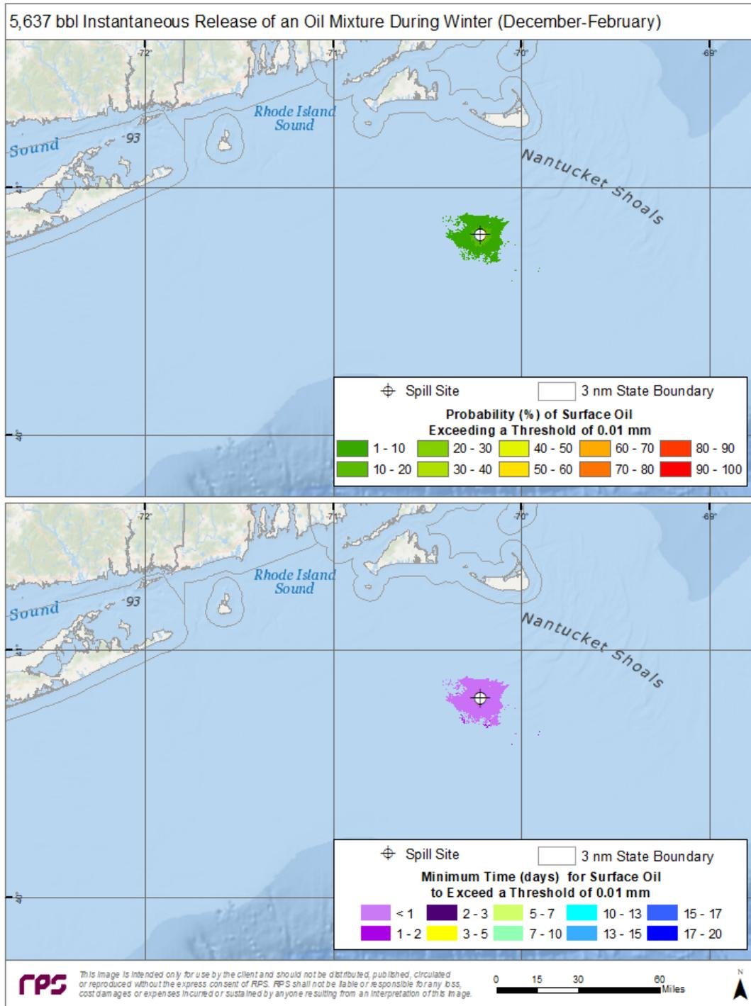
Figure 31. Top Panel—Probability of surface oiling above a minimum thickness of 10  $\mu\text{m}$  (10  $\text{g}/\text{m}^2$  on average over the grid cell) during winter months for an instantaneous discharge from the ESP 1 location. Bottom Panel—Minimum time for surface oiling to occur at thicknesses greater than 10  $\text{g}/\text{m}^2$ .
