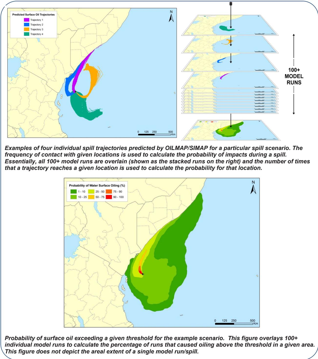
Figure 26. Diagram of RPS stochastic modeling approach; an ensemble of individual trajectories creates the stochastic probability footprint.
