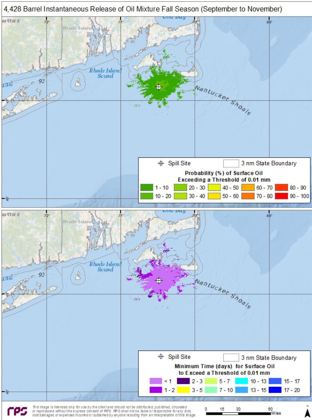
Figure A-21. Detail View. Top Panel—Probability of surface oiling above a minimum thickness of 10  $\mu\text{m}$  (10  $\text{g}/\text{m}^2$  on average over the grid cell) during fall months for an instantaneous discharge from the potential booster station. Bottom Panel—Minimum time for surface oiling to occur at thicknesses greater than 10  $\text{g}/\text{m}^2$ .
