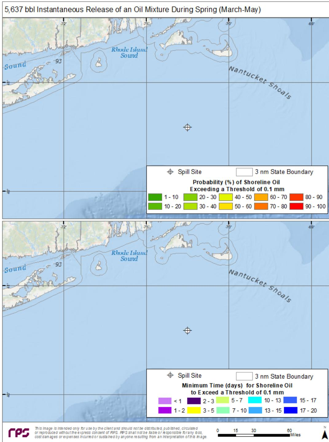
Figure 40. Top Panel—Probability of shoreline oiling above a minimum thickness of 100  $\mu\text{m}$  (100  $\text{g}/\text{m}^2$  on average over the grid cell) during spring months for an instantaneous discharge from the ESP 2 location. Bottom Panel—Minimum time for shoreline oiling to occur at thicknesses greater than 100  $\text{g}/\text{m}^2$ .
