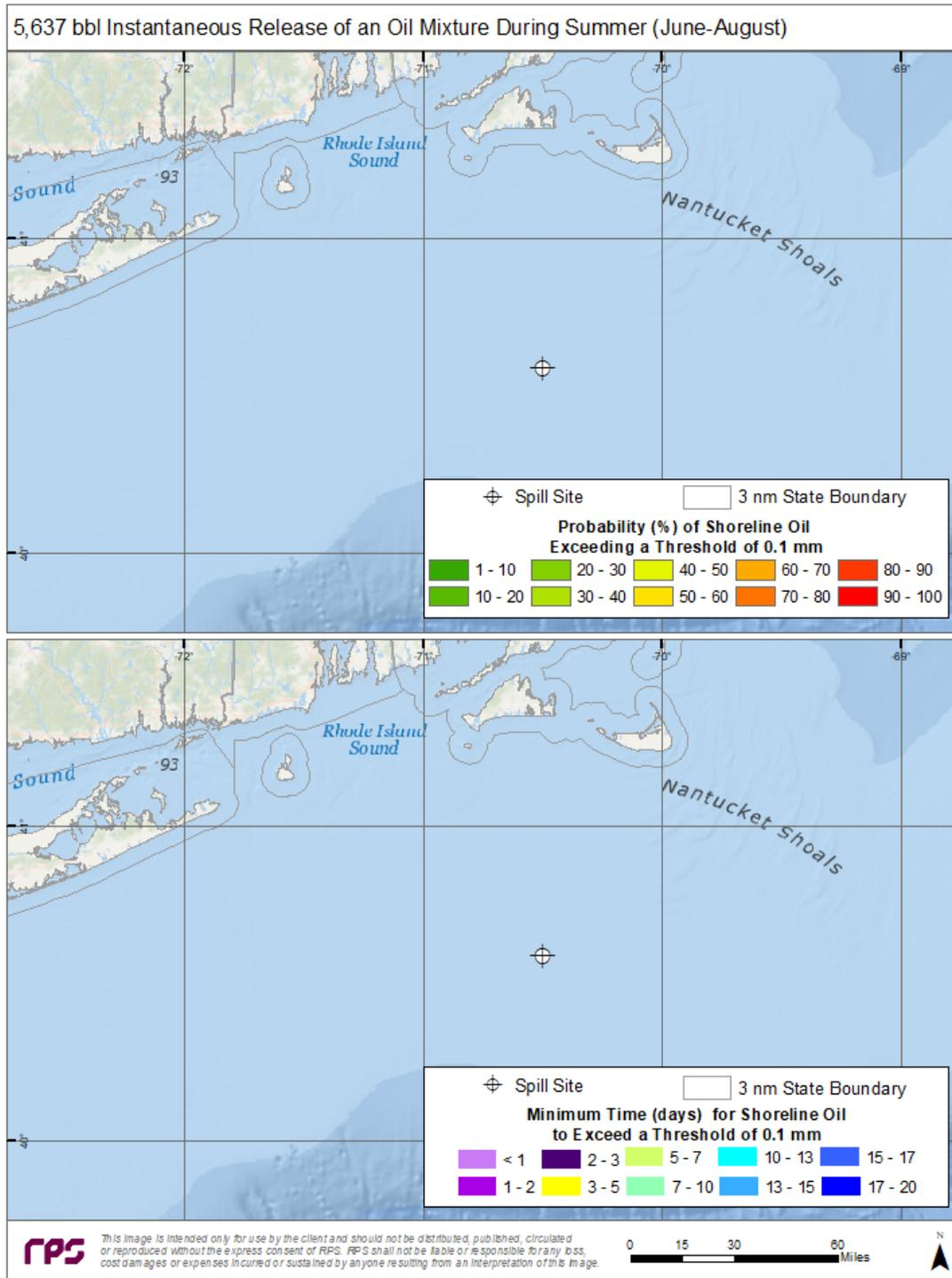
Figure 41. Top Panel—Probability of shoreline oiling above a minimum thickness of 100  $\mu\text{m}$  (100  $\text{g}/\text{m}^2$  on average over the grid cell) during summer months for an instantaneous discharge from the ESP 2 location. Bottom Panel—Minimum time for shoreline oiling to occur at thicknesses greater than 100  $\text{g}/\text{m}^2$ .
