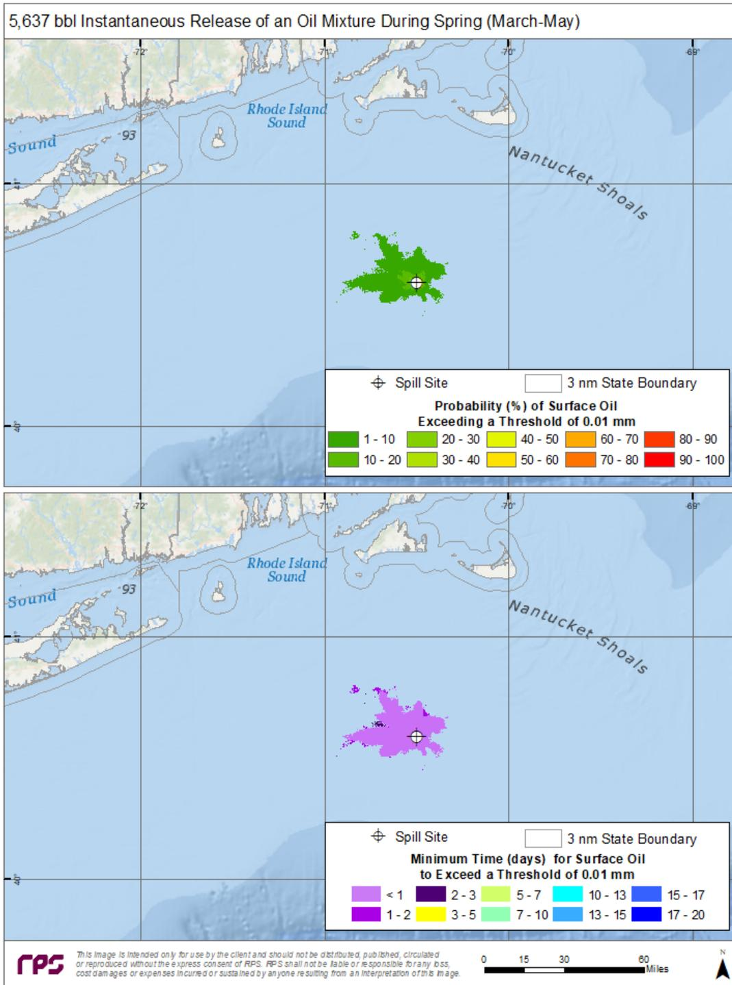
Figure 36. Top Panel—Probability of surface oiling above a minimum thickness of 10  $\mu\text{m}$  ( $10 \text{ g/m}^2$  on average over the grid cell) during spring months for an instantaneous discharge from the ESP 2 location. Bottom Panel—Minimum time for surface oiling to occur at thicknesses greater than  $10 \text{ g/m}^2$ .
