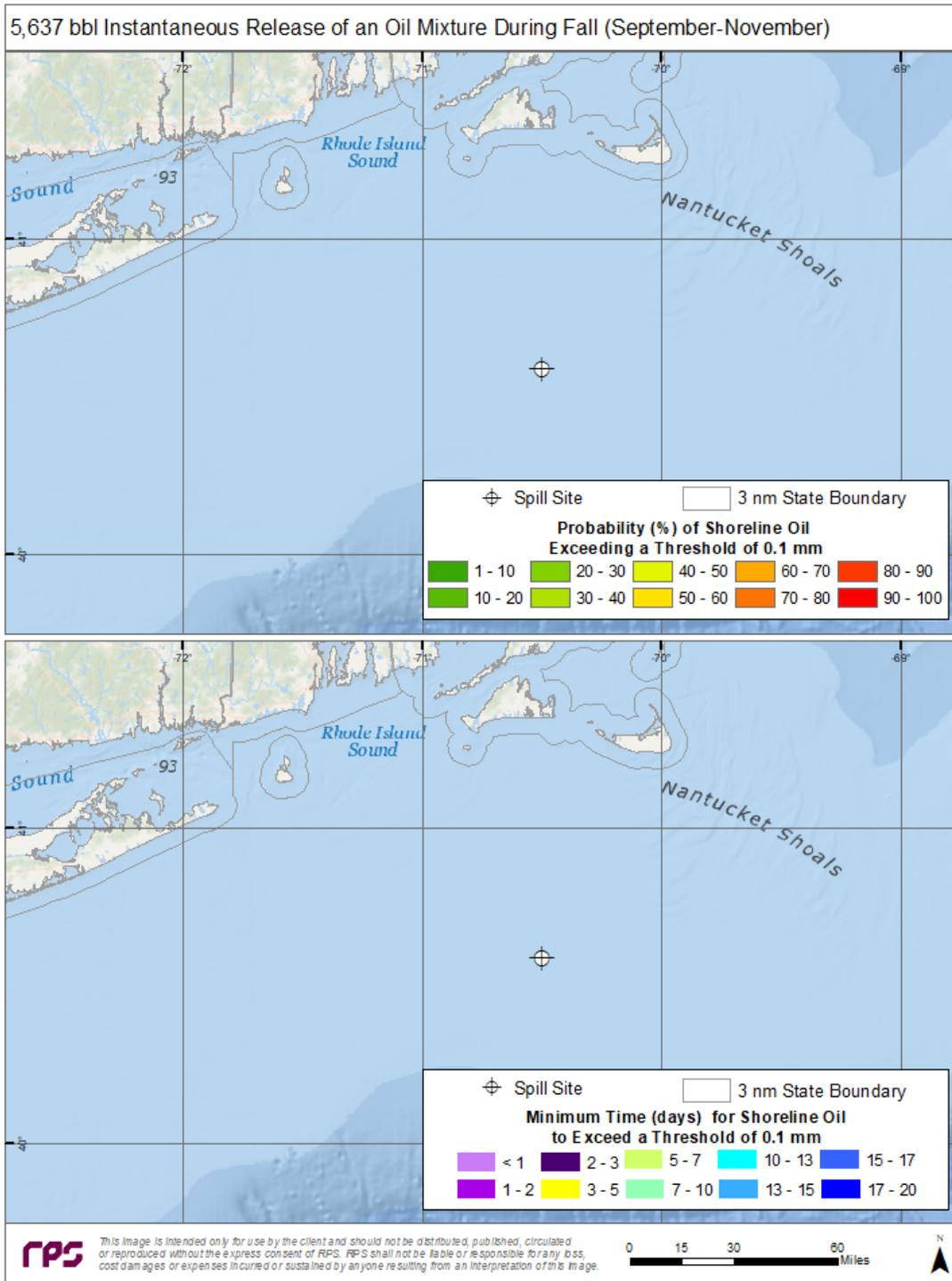
Figure 42. Top Panel—Probability of shoreline oiling above a minimum thickness of 100  $\mu\text{m}$  (100  $\text{g}/\text{m}^2$  on average over the grid cell) during fall months for an instantaneous discharge from the ESP 2 location. Bottom Panel—Minimum time for shoreline oiling to occur at thicknesses greater than 100  $\text{g}/\text{m}^2$ .
