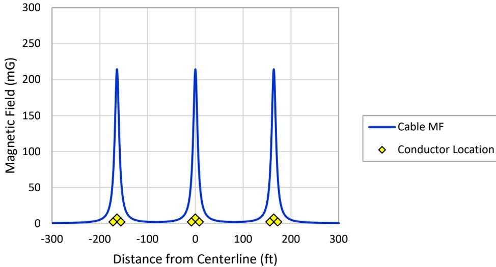
**Figure 4.4 AC Magnetic Field Modeling Results at the Seabed for Buried 345-kV HVAC Offshore Export Cables.** mG = Milligauss. Modeling results are based on three cables buried 1.5 m (4.9 ft) beneath the seabed, each carrying 1,700 A and with 50-m (164-ft) spacing between cables. Conductor locations on the graph are not to scale and are provided to show relative locations.
