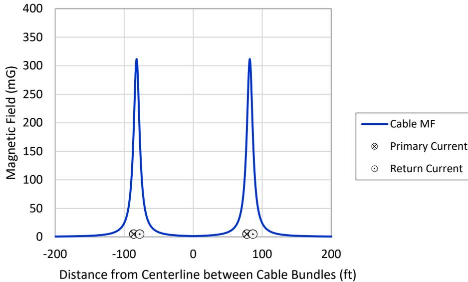
**Figure 3.4 Cable-Specific DC Magnetic Field Modeling Results at the Seabed for Buried  $\pm 525$ -kV HVDC Offshore Export Cables.** mg= Milligauss. Modeling results are based on two cable bundles buried 1.5 m (4.9 ft) beneath the seabed, each carrying 2,300 A and with 50-m (164-ft) spacing between cable bundles. Conductor locations on the graph are not to scale and are provided to show relative locations.
