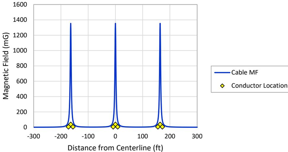
**Figure 4.5 AC Magnetic Field Modeling Results at 0.82 m (2.68 ft) Above the Seabed for Surface-Laid 345-kV HVAC Offshore Export Cables.** mG = Milligauss. Modeling results are based on three cables installed on the seabed covered by 0.5-m (1.6-ft) thick cable protection, each carrying 1,700 A and with 50-m (164-ft) spacing between cables. Conductor locations on the graph are not to scale and are provided to show relative locations.
