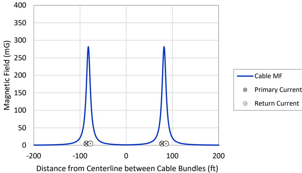
**Figure 3.2 Cable-Specific DC Magnetic Field Modeling Results at the Seabed for Buried  $\pm 320$ -kV HVDC Offshore Export Cables.** mg= Milligauss. Modeling results are based on two cable bundles buried 1.5 m (4.9 ft) beneath the seabed, each carrying 2,300 A and with 50-m (164-ft) spacing between cable bundles. Conductor locations on the graph are not to scale and are provided to show relative locations.
