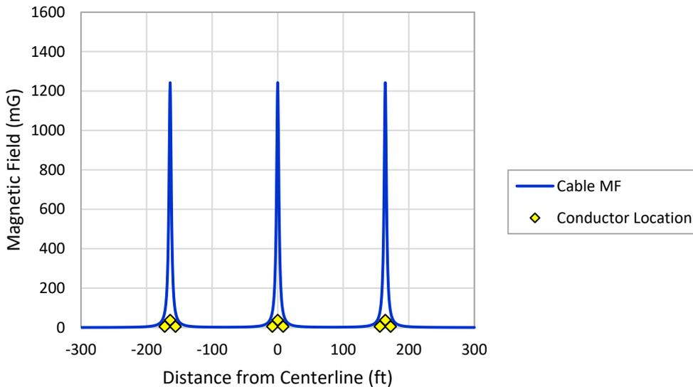
**Figure 4.3 AC Magnetic Field Modeling Results at 0.79 m (2.58 ft) Above the Seabed for Surface-Laid 220-kV HVAC Offshore Export Cables.** mG = Milligauss. Modeling results are based on three cables installed on the seabed covered by 0.5-m (1.6-ft) thick cable protection, each carrying 1,700 A and with 50-m (164-ft) spacing between cables. Conductor locations on the graph are not to scale and are provided to show relative locations.
