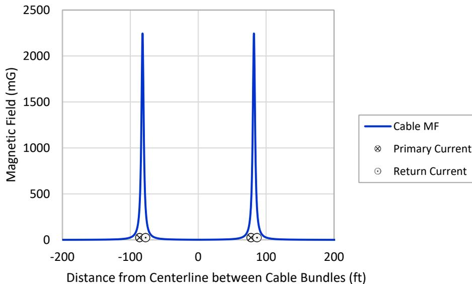
**Figure 3.5 Cable-Specific DC Magnetic Field Modeling Results at 0.67 m (2.20 ft) Above the Seabed for Surface-Laid  $\pm 525$ -kV HVDC Offshore Export Cables.** mg= Milligauss. It is assumed that cable bundles are installed on the seabed and covered by cable protection with 0.5-m (1.6-ft) thickness. Conductor locations on the graph are not to scale and are provided to show relative locations.
