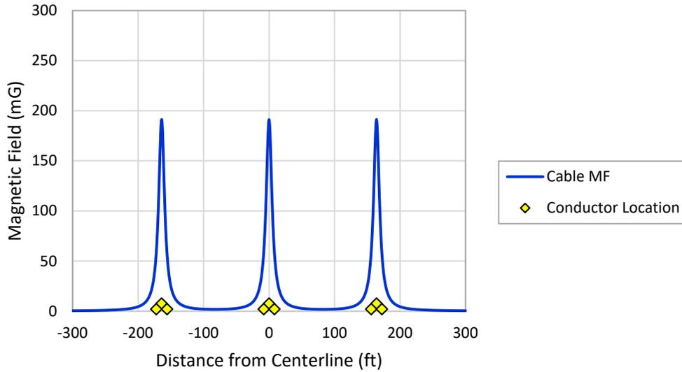
**Figure 4.2 AC Magnetic Field Modeling Results at the Seabed for Buried 220-kV HVAC Offshore Export Cables.** mG = Milligauss. Modeling results are based on three cables buried 1.5 m (4.9 ft) beneath the seabed, each carrying 1,700 A and with 50-m (164-ft) spacing between cables. Conductor locations on the graph are not to scale and are provided to show relative locations.
