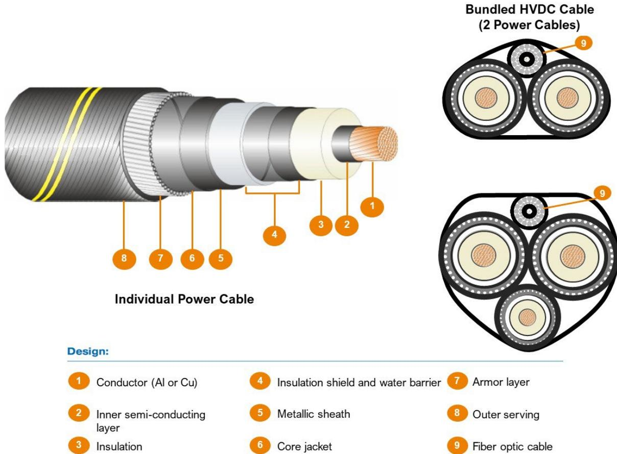
**Figure 3.1 Example HVDC Cable Cross Section Illustration.**
