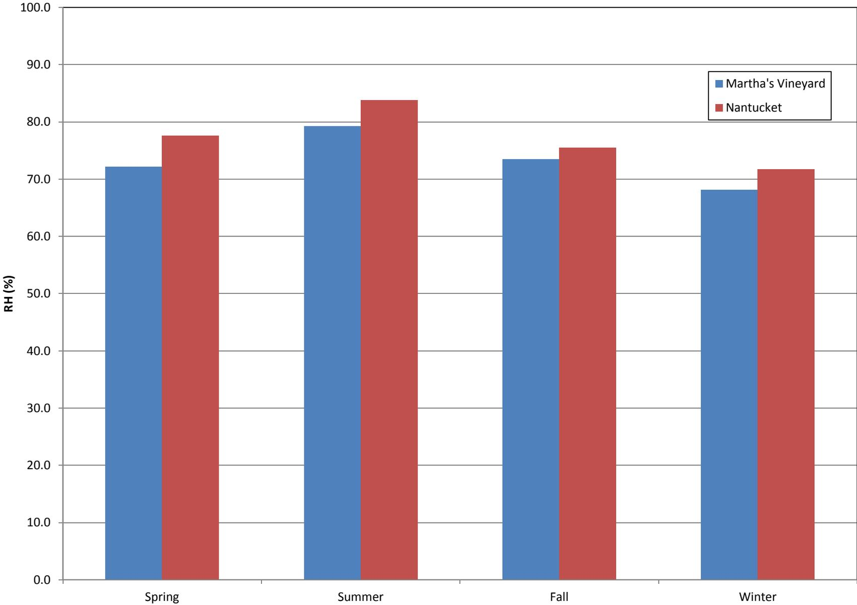
Relative humidity has been shown to have a strong effect on visibility (Zhang et al. 2015; Malm 1999). Water vapor condenses on particles in the air, thereby increasing their size and the corresponding amount of light scattered or absorbed. Figure 7 shows the seasonal changes in relative humidity amongst the two stations with Nantucket having slightly higher average relative humidity.
