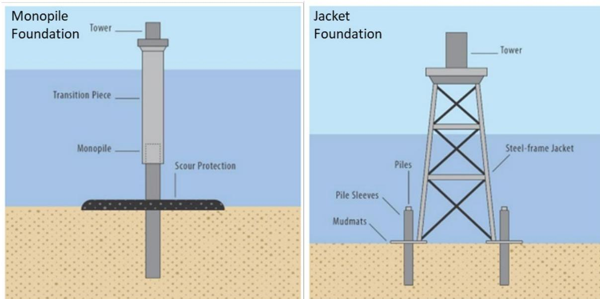
**Figure 5. Examples of Monopile and Jacket Foundations**
