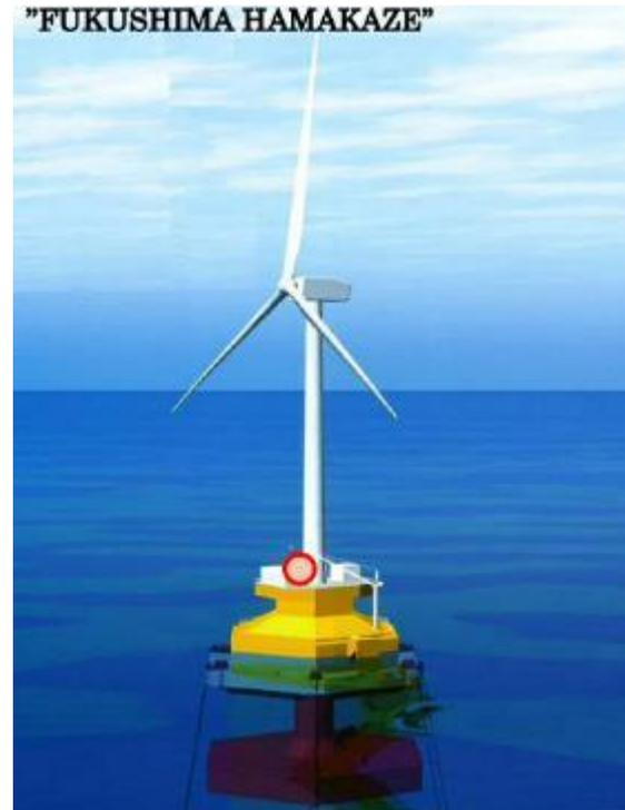
Figure 3 FOWT Design Concept - Fukushima Advanced Spar
