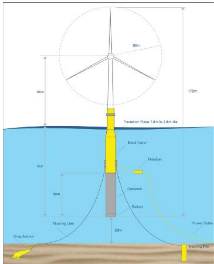
Figure 2 FOWT Design Concept - Toda Hybrid Spar
