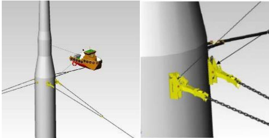
**Figure 33 Mooring Tensioning Process – Hywind Scotland Project (Statoil, 2015)**
