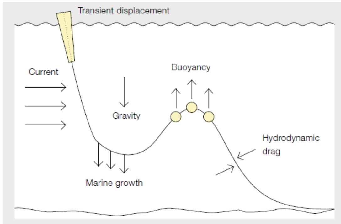
**Figure 44 Factors Affecting the Mechanical Load on the Dynamic Cable (Eriksson et al., 2011)**
