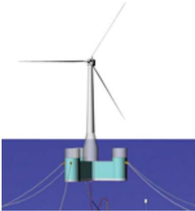
The cobra semi-spar consists of a central cylinder, which provides structural continuity to the tower, and three outer cylinders that provide metacentric stability and buoyancy during transport and operation.
