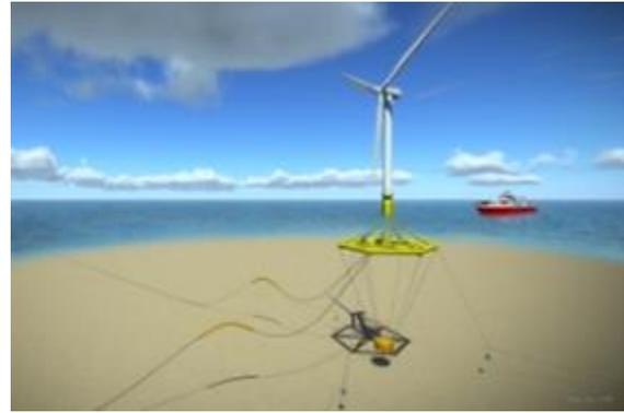
Figure 13 FOWT Design Concept – Hexafloat
