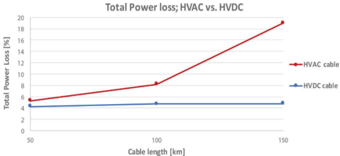
**Figure 43 Total power loss in a HVAC and a HVDC system (Våben and Gudmestad, 2018)**
