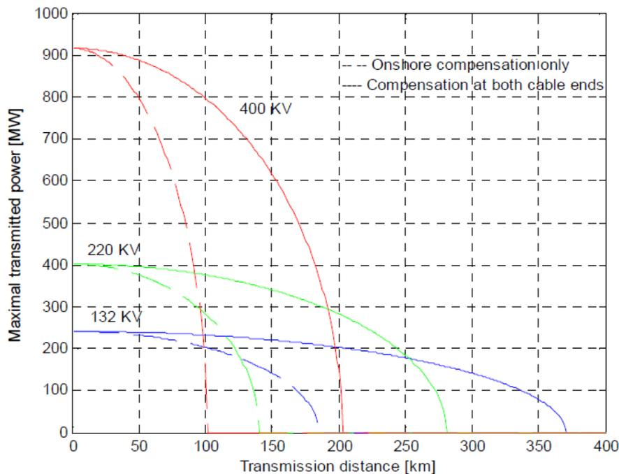
**Figure 42 Limits of HVAC Cables Transmission Capacity for Three Voltage Levels, 132 kV, 220 kV, and 400 kV (Ackermann et al., 2005)**
