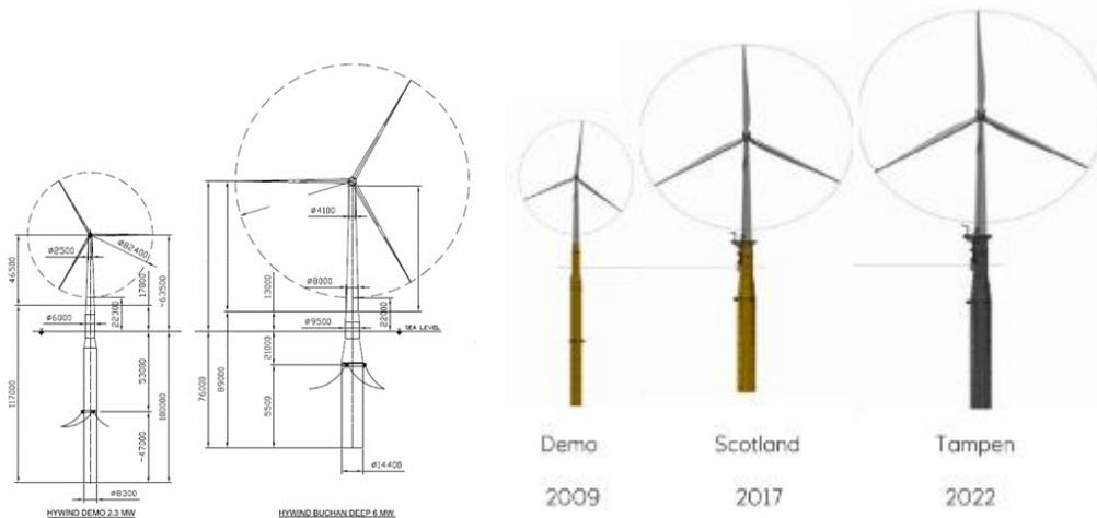
**Figure 30 Comparison of Hywind Demo (2.3 MW) to Hywind Scotland (6 MW), and Hywind Tampen (Equinor, 2014; Equinor, 2019)**
