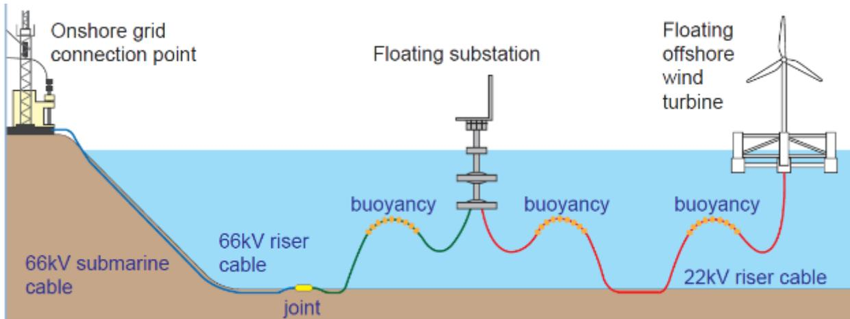
Figure 37 Fukushima FORWARD Project Power Cable System (Fukushima Offshore Wind Consortium, n.d.)
