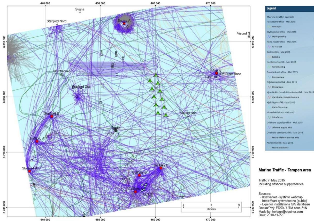
Figure 68 All vessel transits on the Tampen field in May 2015. (Equinor, 2019)
