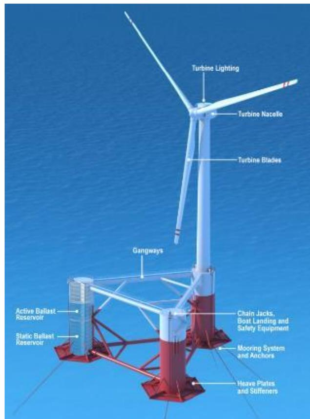
Figure 6 FOWT Design Concept - WindFloat
