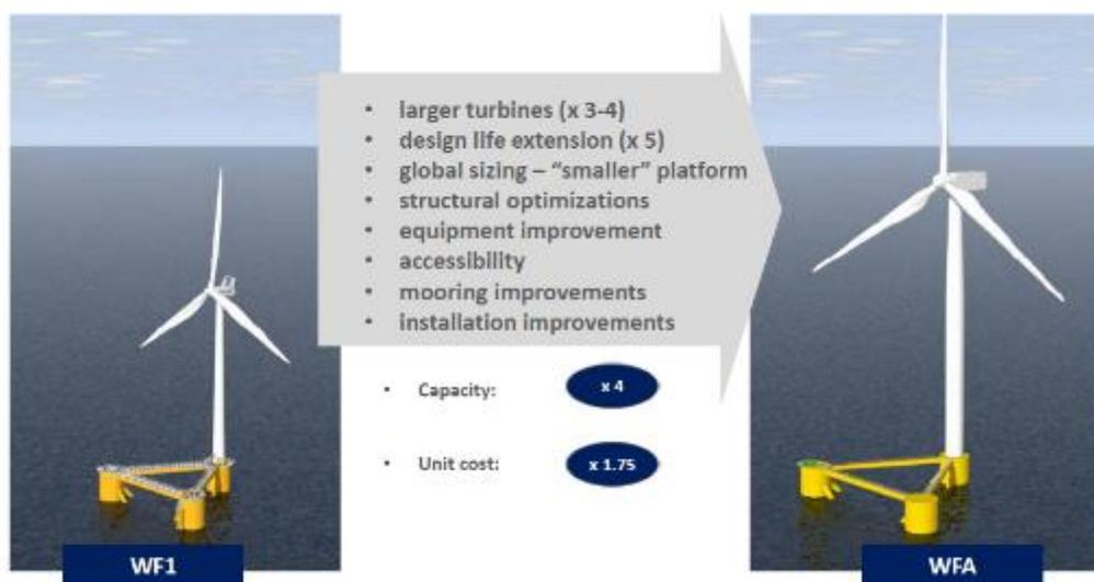
Figure 31 Windfloat Atlantic - Scaling-up and additional innovations (WindPlus, 2019)
