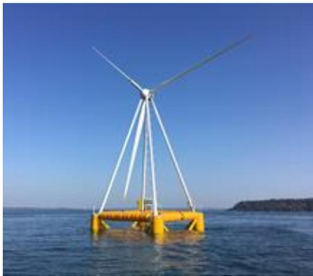
Figure 14 FOWT Design Concept – Eolink
