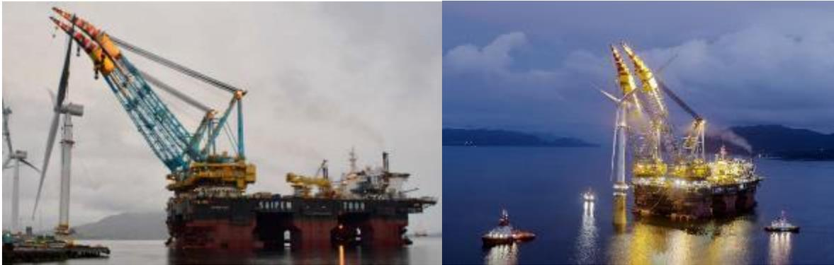
Figure 53 Hywind Scotland – Inshore Assembly of a FOWT (Equinor, n.d.; Technip, 2016)
