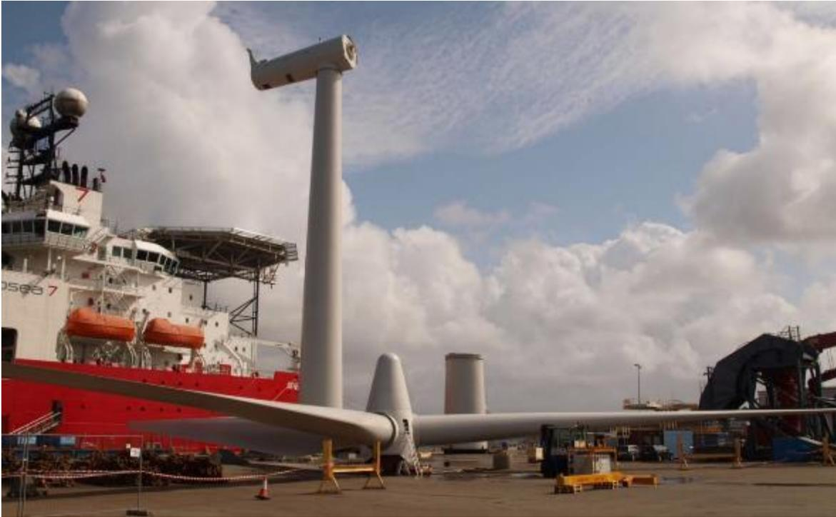
**Figure 49 Hywind Demo Project – Partially Assembled Wind Turbine and Tower (Statoil, 2009)**
