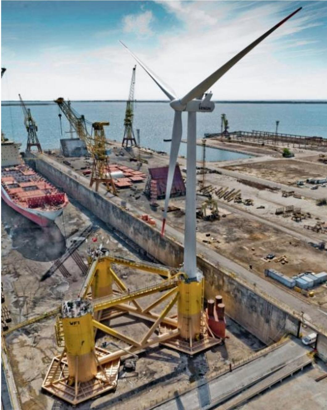
Figure 51 The WindFloat Prototype in Preparation for its Tow Offshore (ASM Industries, 2020)
