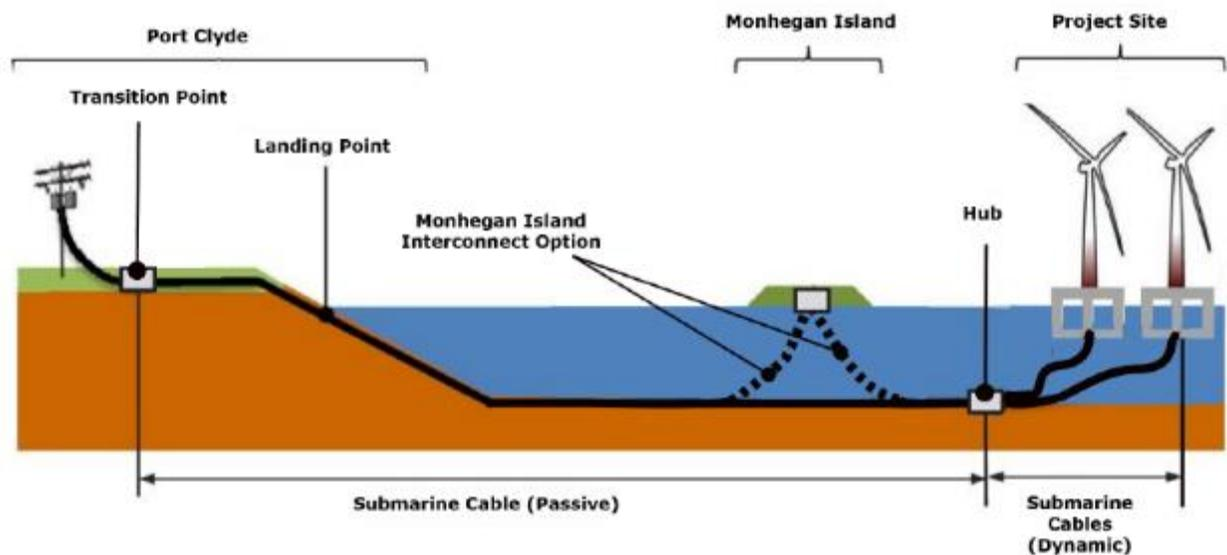
Figure 36 Components of Project Electrical Interconnection – New England Aqua Ventus I Wind Project (Durakovic, 2020)
