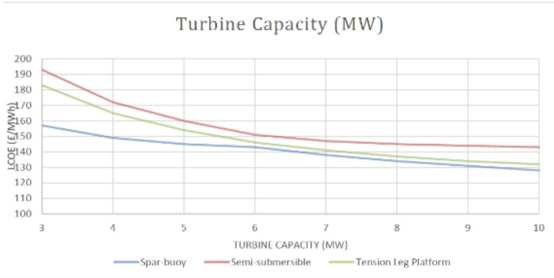
Figure 86 Modeled Turbine Capacity and LCOE by Foundation Type (Heidari, 2017, pg. 42)
