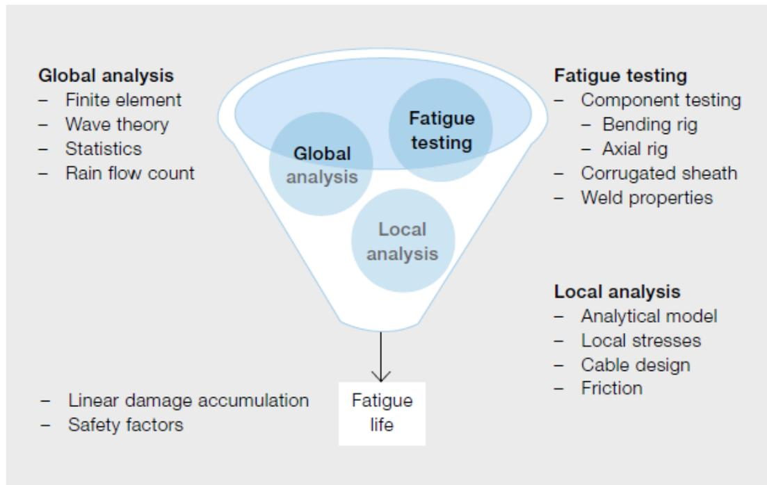
**Figure 45 Conceptual Layout of Foundation in order to Determine Fatigue Life (Eriksson et al., 2011)**
