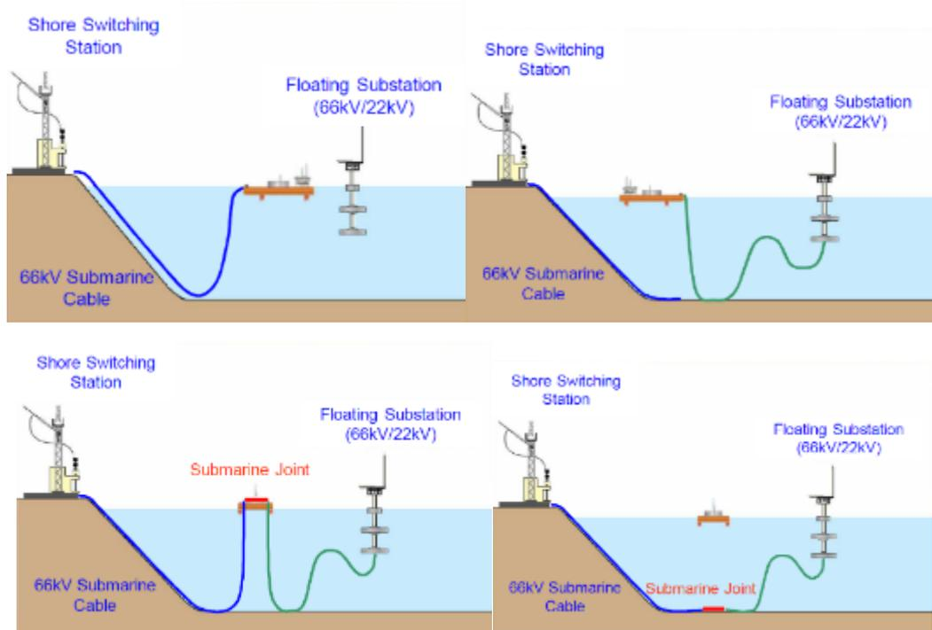
Figure 56 Installation 66 kV Static and Dynamic Export Cable – Fukushima FORWARD Project (Yagihashi et al., 2015)
