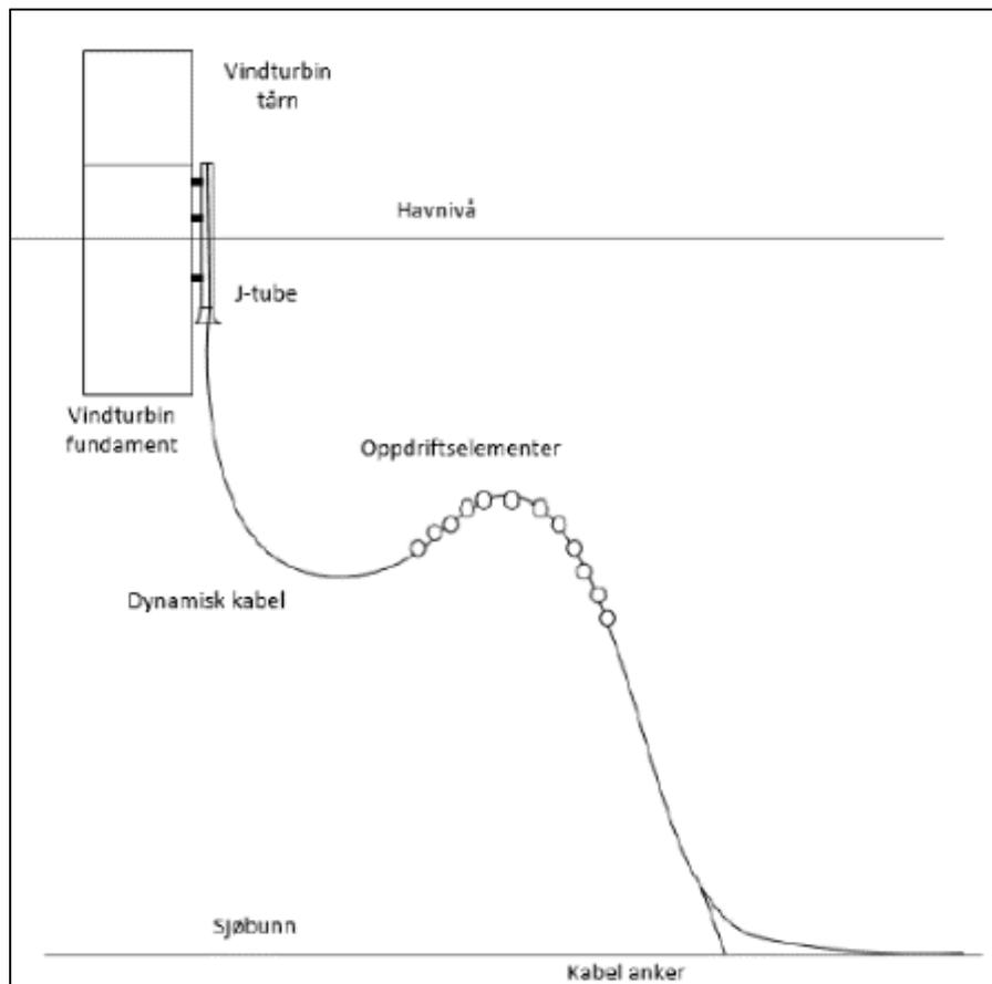
Figure 58 Hywind Tampen dynamic power cable in the water column (Equinor, 2019)
