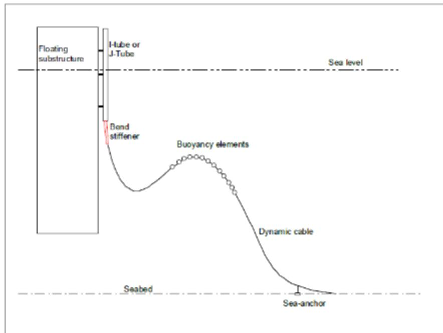
**Figure 41 Schematic of the Attachment of the Array Cable to the WTG (Statoi, 2015)**
