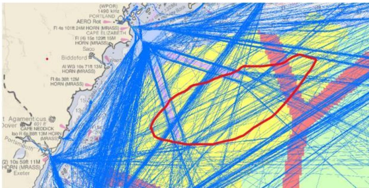
Figure 76 Cargo, Tanker and Tug&Tow vessel transits in the Gulf of Maine (MarineCadastre.gov)
