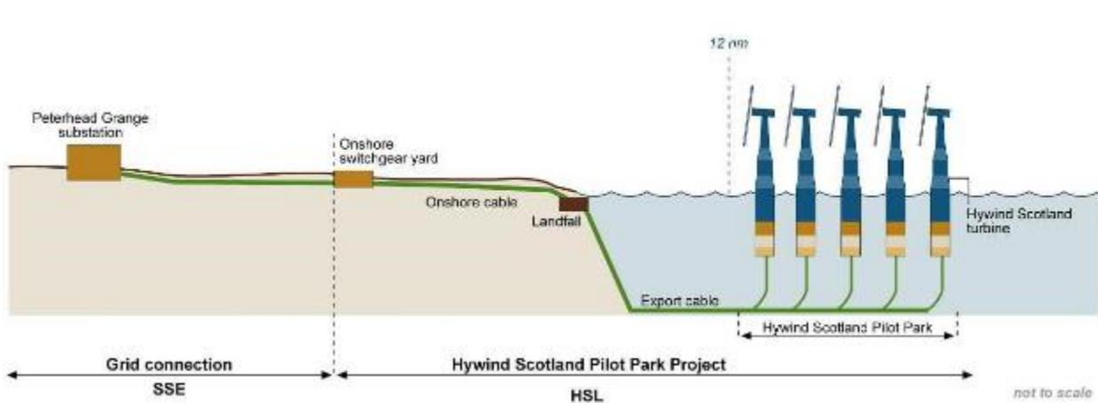
**Figure 40 Key components of the Hywind Scotland Pilot Park Project (Statoil, 2015)**
