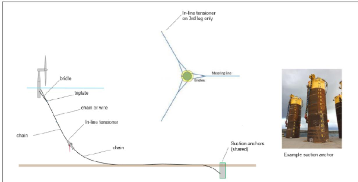
Figure 59 Hywind Tampen anchoring system (Equinor, 2019)
