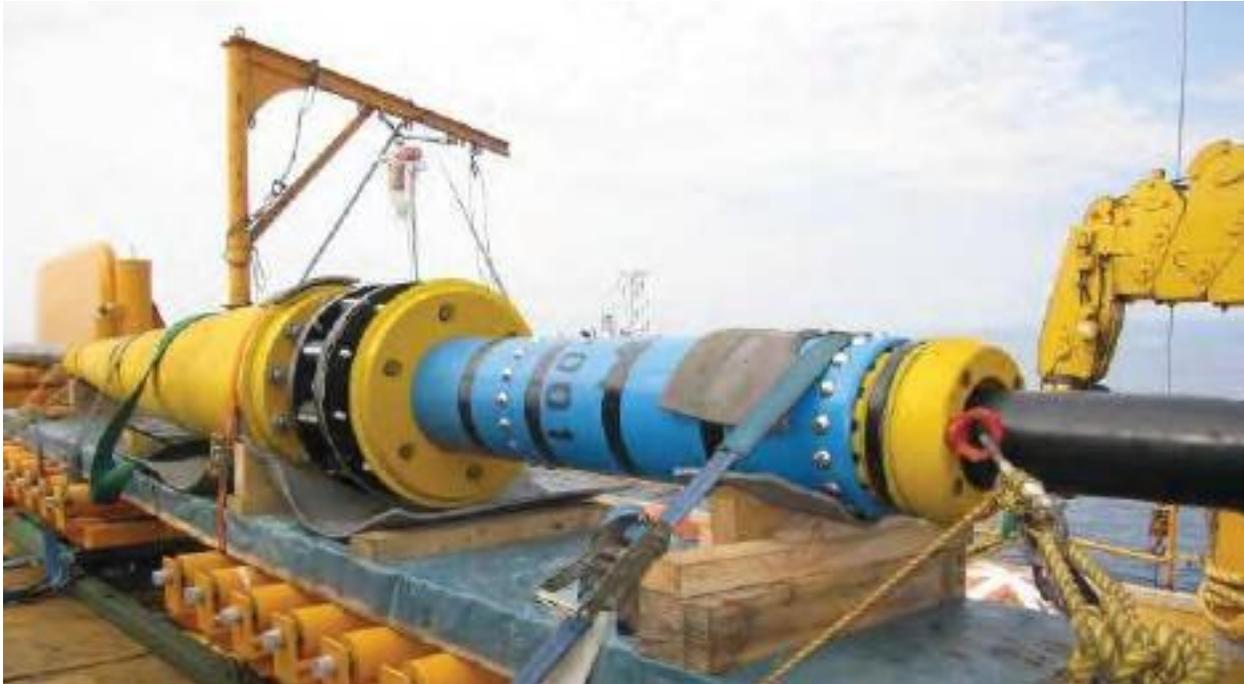
**Figure 39 Fukushima FORWARD Project 66 kV Bend Stiffener Connector by First Subsea (Fuji and Tanaka, 2013)**
