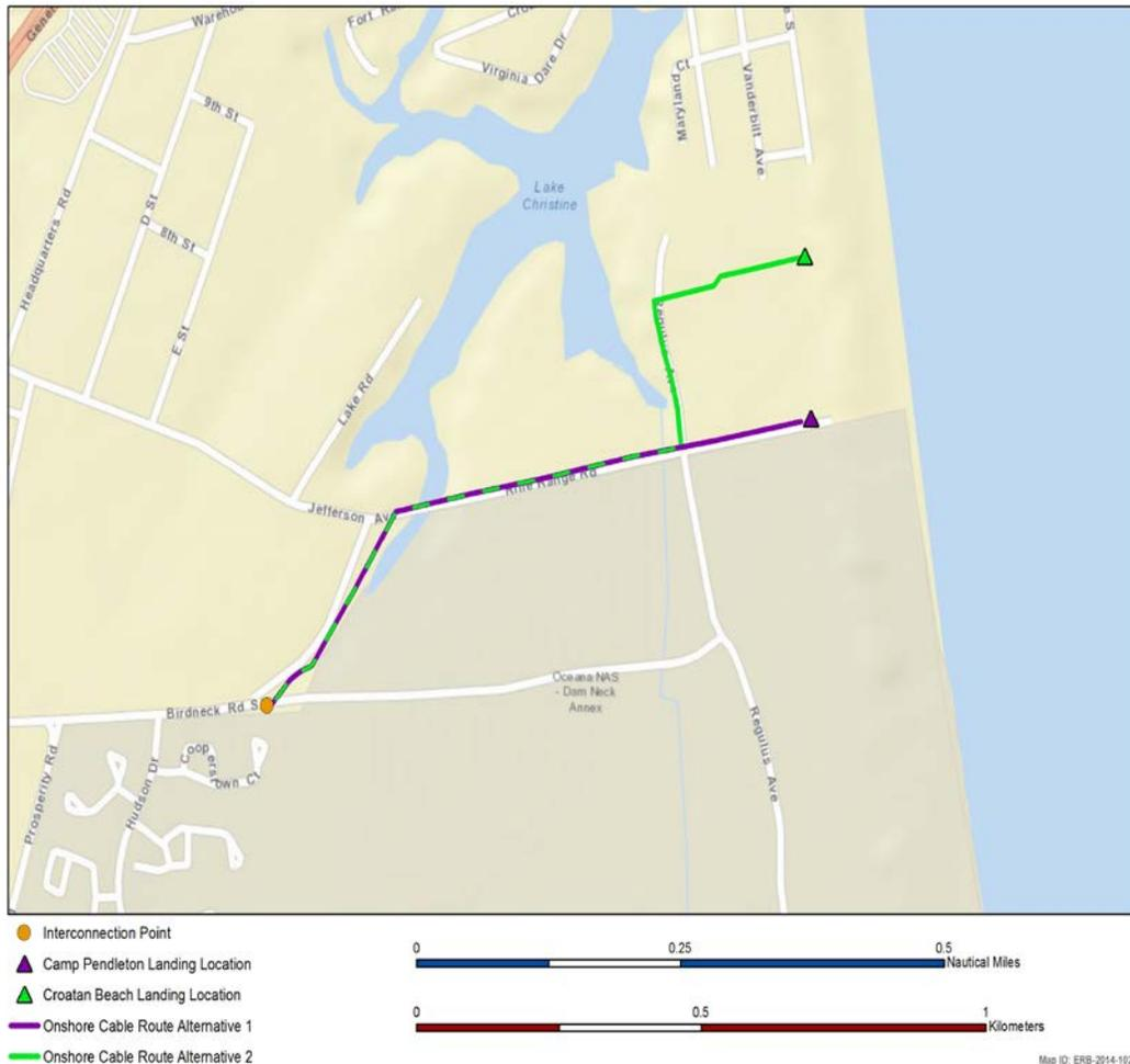
**Figure 2. The VOWTAP onshore portion of the project area. Preferred on shore underground cable route (purple) and the alternative landfall and cable route (green) within Camp Pendleton.**
