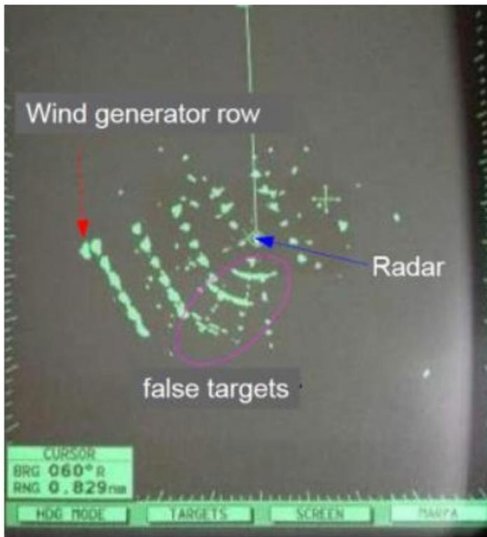
**Figure 9.14: False Targets on the Radar Display [Source: PIANC, 2018]**
