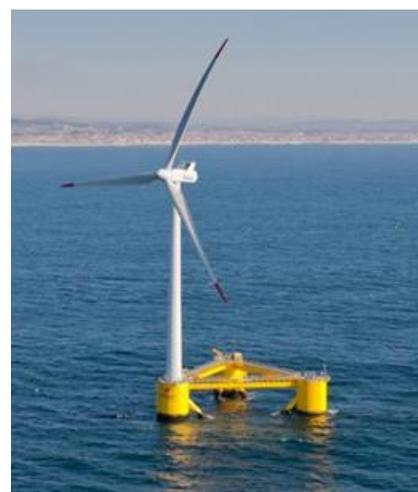
**Full-scale prototype of WindFloat device**
