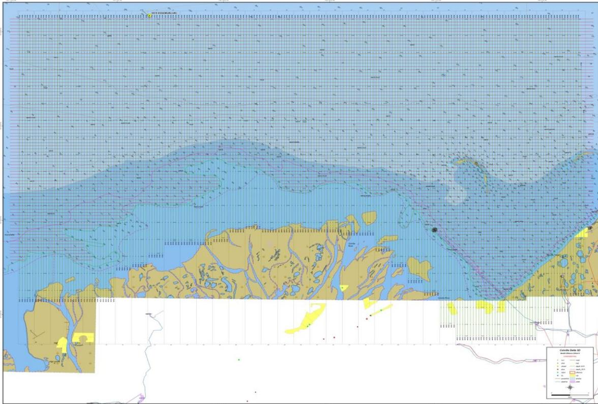
**Figure 1-2. Configuration of Shot and Receiver Lines**
