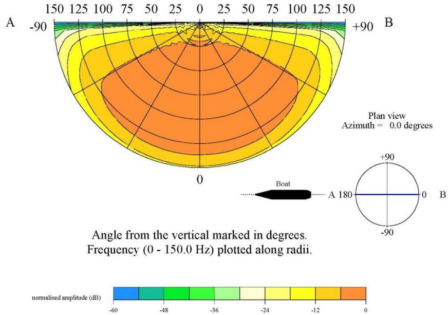
Source Directivity Plot - azimuth : 90.0 degrees - array SeaScan\_USW\_4x220\_2m
