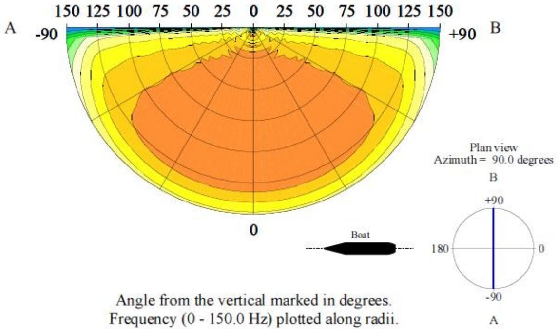
Source Directivity Plot - azimuth : 0.0 degrees - array SeaScan\_USW\_440\_2m
