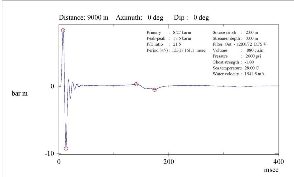
Source Directivity Plot - azimuth : 0.0 degrees - array SeaScan\_USW\_4x220\_2m
