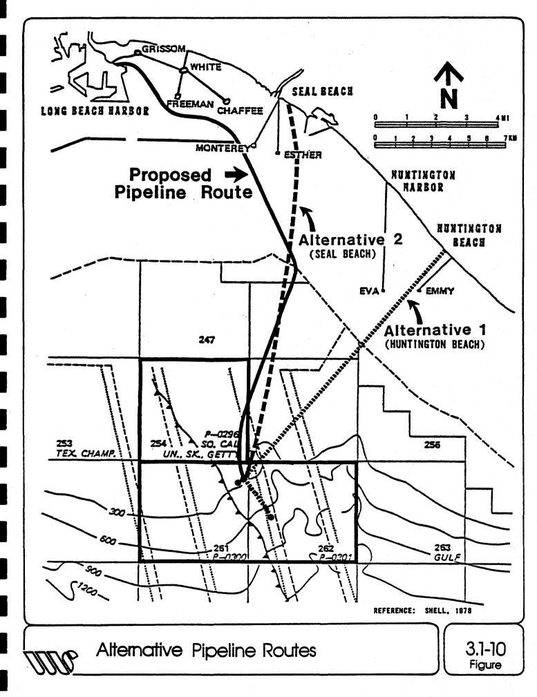
range from 18 to 270 feet (5.5 to 82 m). The overall slope of the seafloor within the pipeline corridor is southerly with slopes ranging from 0.15 degrees to 3 degrees. The seafloor is relatively featureless, with some depressions noted in the Long Beach Harbor (Dames and Moore, 1977b).
