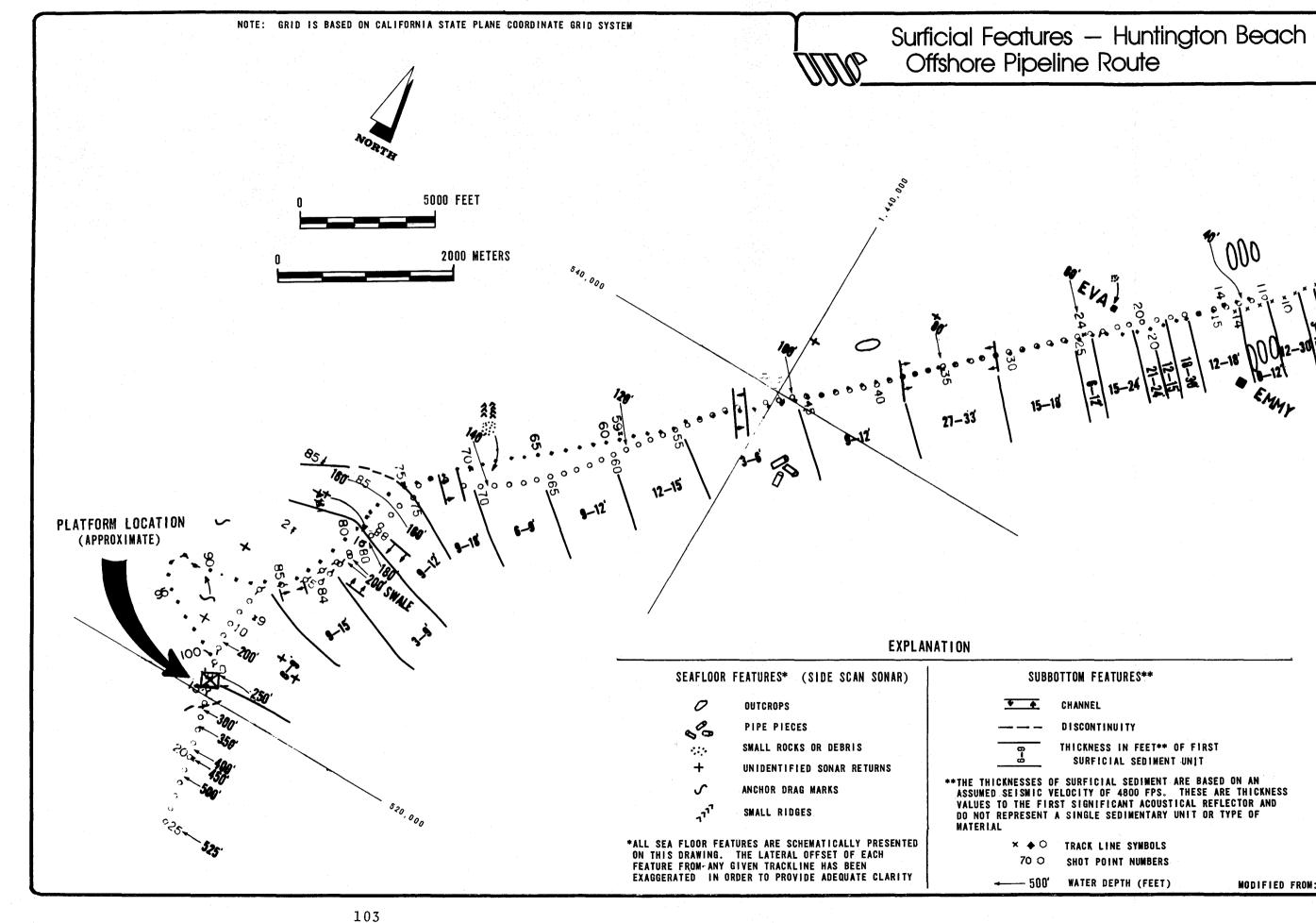
3.1-15 Figure ///0 SHORE LINE THICKNESS IN FEET\*\* OF FIRST SURFICIAL SEDIMENT UNIT \*\*THE THICKNESSES OF SURFICIAL SEDIMENT ARE BASED ON AN Assumed seismic velocity of 4800 FPS. These are thickness VALUES TO THE FIRST SIGNIFICANT ACOUSTICAL REFLECTOR AND DO NOT REPRESENT A SINGLE SEDIMENTARY UNIT OR TYPE OF TRACK LINE SYMBOLS SHOT POINT NUMBERS MODIFIED FROM: DAMES AND MOORE (1977b)
