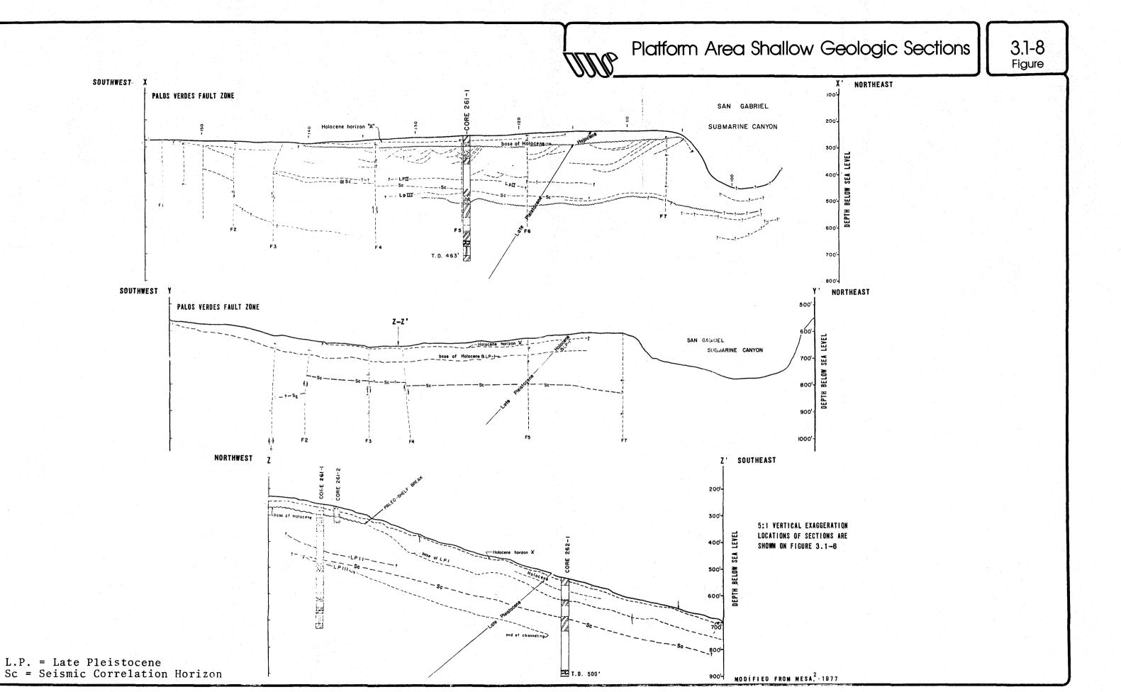
Their location relative to the proposed platforms are shown on Figure 3.1-9. The soil types encountered in these boreholes generally agree with the Quaternary stratigraphic section developed by Mesa<sup>2</sup> (1977) (Table 3.1-2), based on boreholes 261-1, 261-2, and 262-1.
