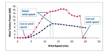
Each turbine and turbine type have different theoretical power curves – DC and Stall (above) and variable pitch for multiple class turbines (below)
