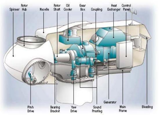
Components of a typical constant speed induction wind turbine
