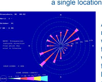
A wind power rose indicates which direction the energetic winds come from, which helps in turbine siting
