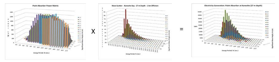
Wave Energy Conversion (WEC) Device Performance Power Matrix x Wave Scatter = Electricity Generation
