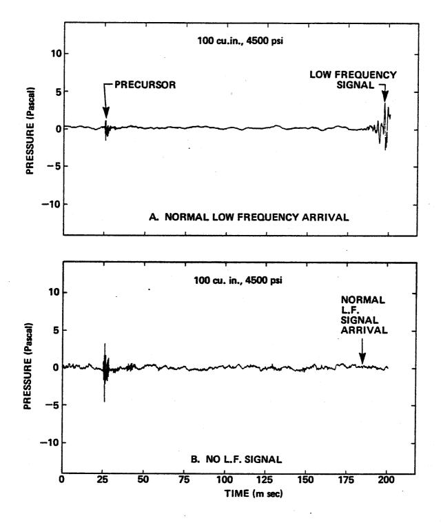
FIG. 5.6. AIR GUN SIGNALS AT 15.5 km RANGE (PRECURSOR COMPONENTS).
