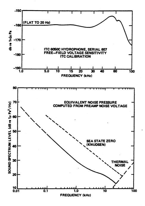
FIG. 3.3. MEASUREMENT HYDROPHONE CHARACTERISTICS.
