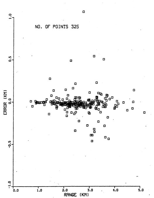
FIG. E.1. ERRORS IN RANGE FROM VERTICAL BEARINGS AT SOBERANES SITE IN 1984 AS A FUNCTION OF RANGE.
