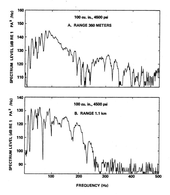
FIG. 5.3. AIR GUN SIGNAL SPECTRA.
