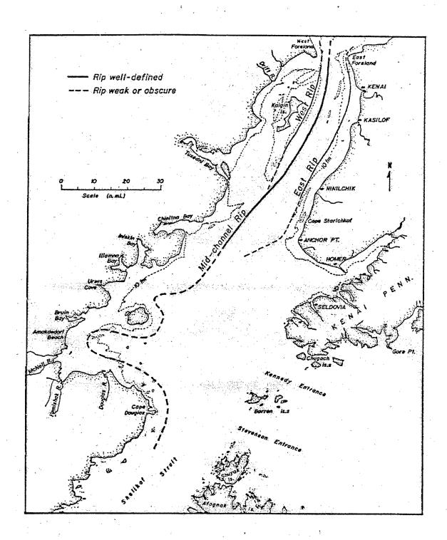
Figure 2. Historic map of major rip tides (frontal zones) in lower Cook Inlet, Alaska (Burbank 1977). The dashed lines indicate where the rips are weak or obscure. The bathymetry shows only the 10-fathom (20 m) contour. One fathom equals 1.8 meters.
