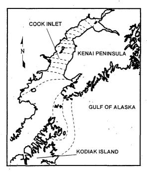
Figure 5. Cotidal lines for Cook Inlet, Alaska (graphics provided by Center For Operational Oceanographic Products and Services [CO-OPS]/NOAA).
