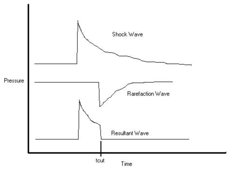
Figure 12. Superposition of Shock Waves.
