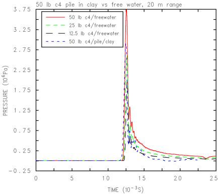
Figure 9. Pressure Time Histories for Pile in Clay and Free-water Numerical Simulations.
