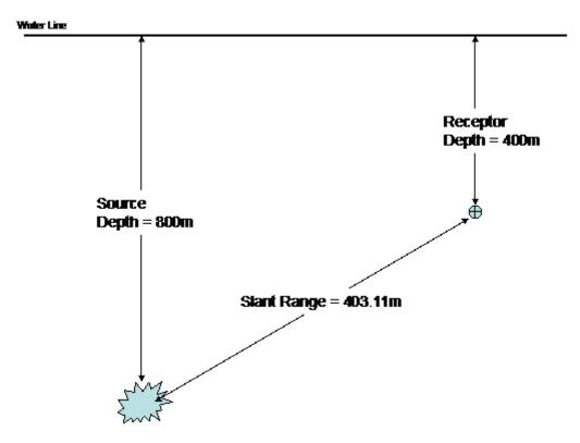
Figure 15. Free-water Configuration Used for Comparison.
