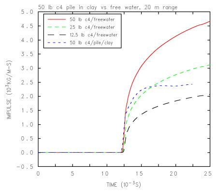
Figure 10. Impulse Time Histories for Pile in Clay and Free-water Simulations.
