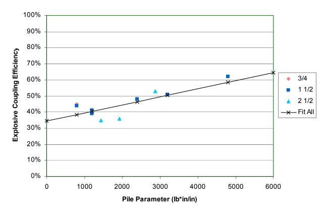
Figure 11. Relationship between the Explosive Coupling Efficiency and the Pile Parameter  $\left(w \cdot \frac{d}{t}\right)$ .
