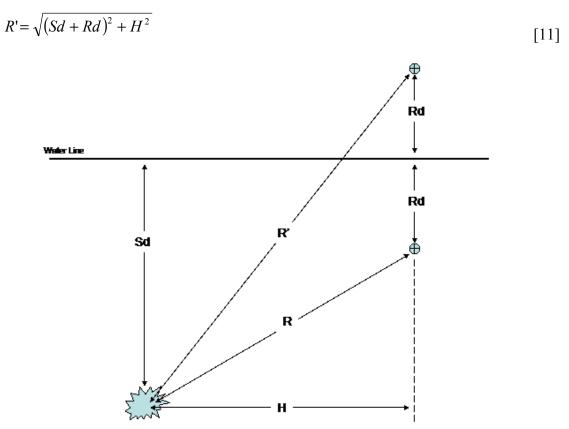
Figure 14. Geometry for Time Cut-Off of the Shock Pulse.
