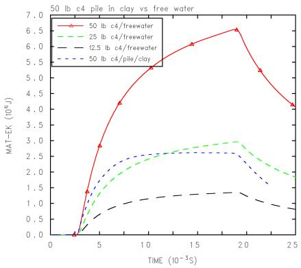
Figure 8. Kinetic Energy Coupled into the Water for Pile in Clay and Free-water Numerical Simulations.
