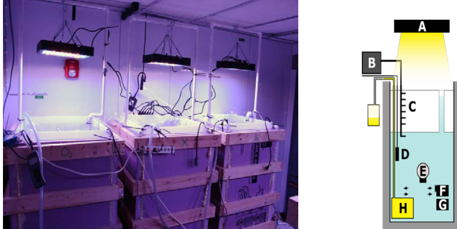
Figure 3. Incubation tanks (left) and schematic showing positions of sensors and equipment in each tank (right): (A) LED light fixture, (B) datalogger, (C) thermistor chain, (D) temperature and salinity probe, (E) 4\pi light sensor, (F) circulation pump, (G) heater, and (H) pressure release bladder.
