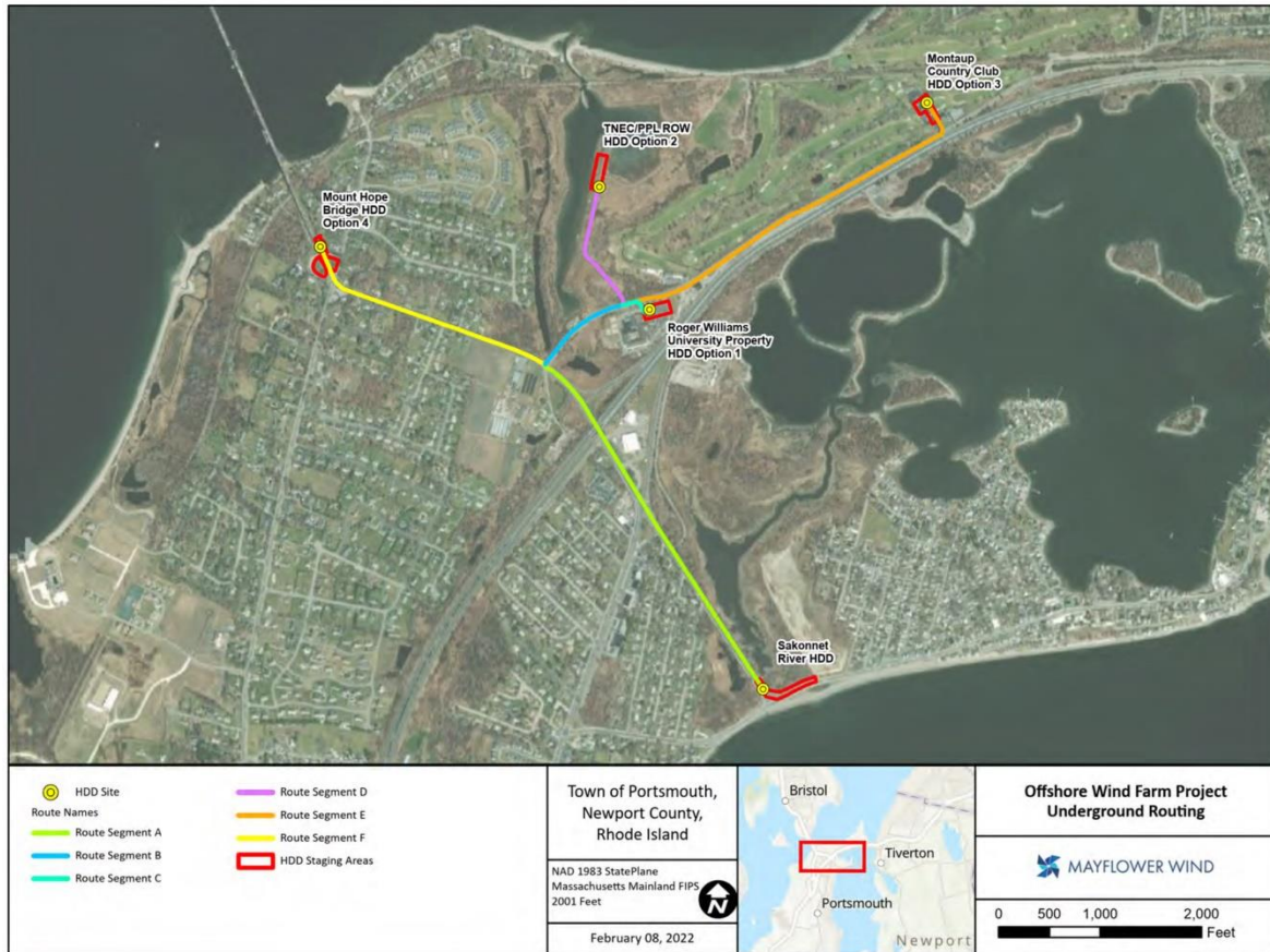
Figure 1. Proposed onshore cable routes and HDD locations for the Mayflower Wind Aquidneck Island (Portsmouth) Landfall.
