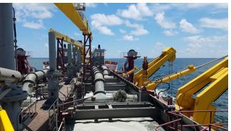
Hopper dredge used to collect sediment resources from the OCS
