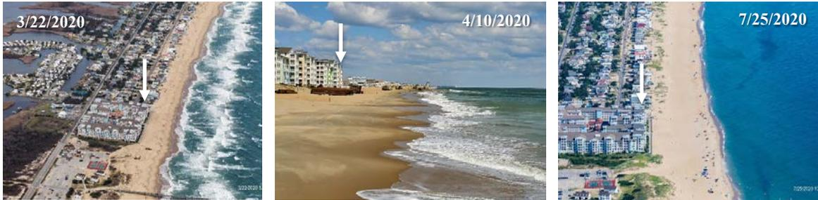
Project proponents completed the most recent construction cycle in summer 2020, using approximately 2.2 million cubic yards of sand from Sandbridge Shoal. BOEM worked with the project team to delineate a smaller dredging footprint within the larger Sandbridge Shoal borrow area to minimize environmental impacts and conserve the resource for future projects.
