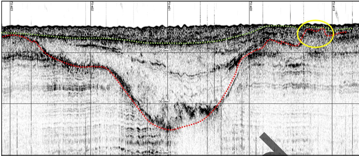
**Figure 1: Example of Interpreted sub-Bottom Data Sample (from Evans 2015:70).** A levee feature is circled in yellow, the channel horizon is indicated in red, and the ravinement surface is illustrated in green. Vertical scale lines are in 150 m intervals; horizontal scale lines are in 7.5 m intervals.
