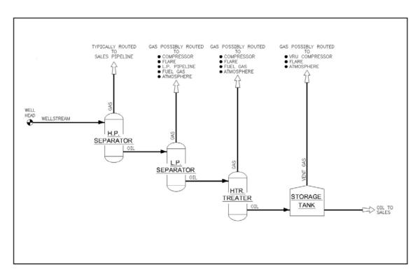
For each stage of flash (e.g., low-pressure separator oil to heater treater) that is vented to the atmosphere (locally or to remote vent) or flared (locally or to remote flare), the operator should give the following data:
