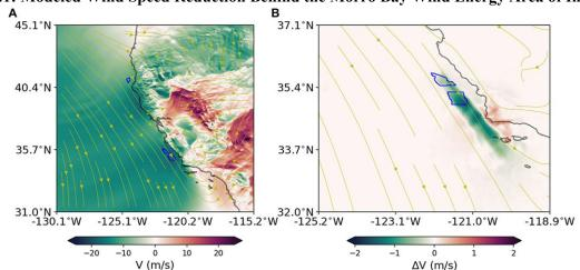
Figure 21: Modeled Wind Speed Reduction Behind the Morro Bay Wind Energy Area of Interest
