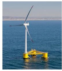
A full-scale prototype of the WindFloat device
