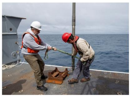
BOEM and USGS researchers recover a gravity core full of pelagic mud from a depth of approximately 3200 meters.
