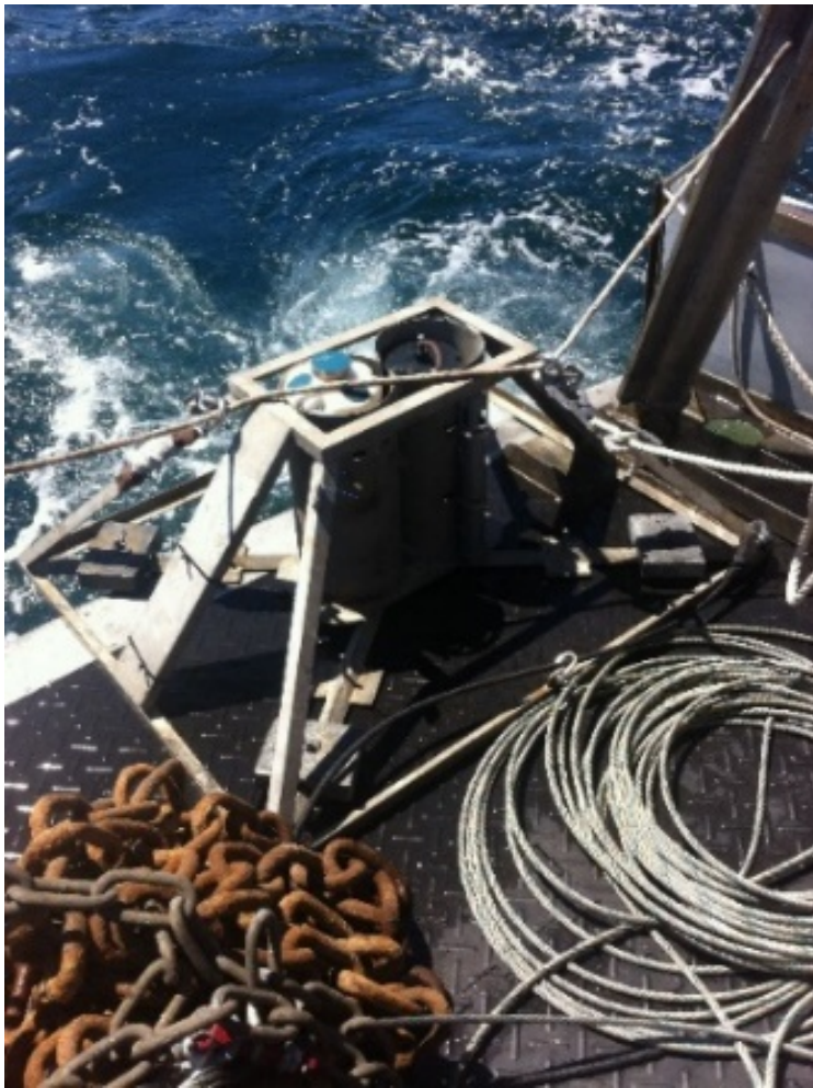
Figure 8. Scour monitor in bracketing (top); seafloor frame and AWAC (bottom).
