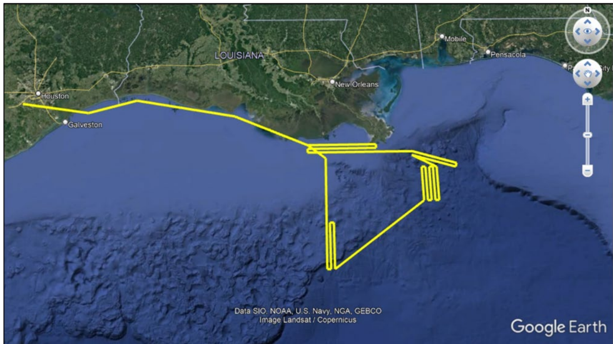
Figure 1. GV aircraft flight plan (yellow lines) over the GOM during TRACER-AQ to measure TROPNO 2 with GCAS, and ozone and aerosol profiles with HSRL2.
