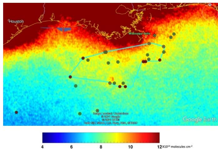
Figure 1: Using the Annual Average TROPOMI TROPC column NO<sub>2</sub> to determine the Draft G-V Flight Path
