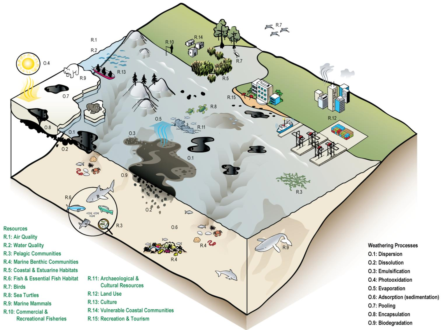
Figure 4-22. Oil spill weathering processes and impacted resources
