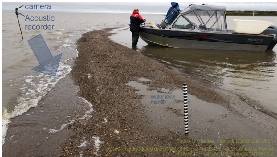
Figure 2. Monitoring equipment installed at Oarlock Island in Dease Inlet in July 2021. Each monitoring station included a time-lapse camera, acoustic recorder, and water-level marker. The arrow illustrates the direction of the camera angle toward the water-level marker and the rest of the spit where seals haul out. A second camera was placed to monitor seals hauling out on another section of the spit. A weather station was located on the tundra bluff above the spit. Photo courtesy D. Hauser (UAF).
