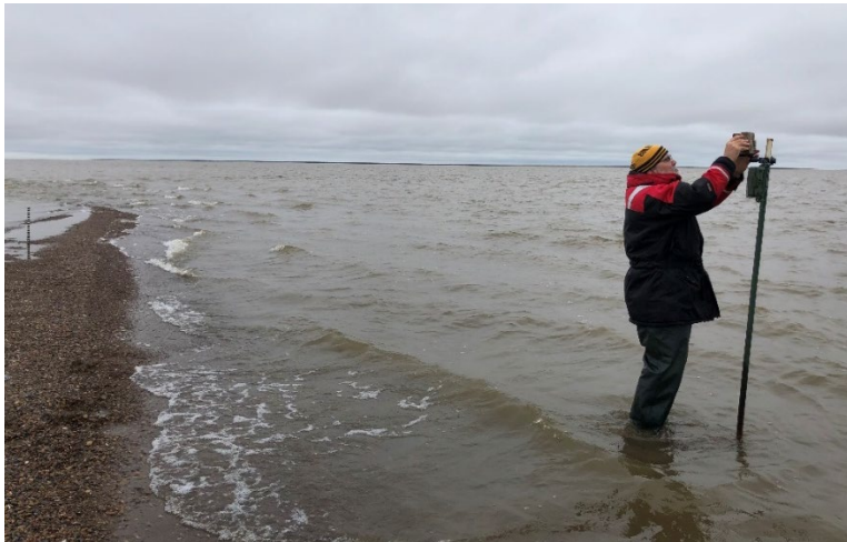
Figure 5. Oarlock Island haulout site on 24 July 2021. The water-level marker is in the background along the far side of the spit, while Co-PI Von Duyke replaces the time-lapse camera. The acoustic recorder is located on the post below the camera. Wind-driven erosion of the spit occurred after this photograph, and the spit was underwater and unavailable as a haulout for seals by August 2021. Photo by D. Hauser.
