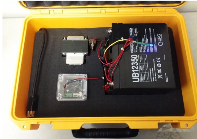
Figure 13. Sensor Able in Pelican case with 12V battery (at right), charger (upper left), and SVS-603 sensor (lower left). This unit can log data for more than 30 days at -20^{\circ}\text{C} .
