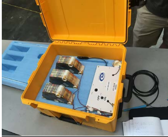
Figure 6. Three battery packs next to the control switch in an Ice Wave Rider unit. The USB flash drive is at the back of the case, easily accessible for field swap-out.
