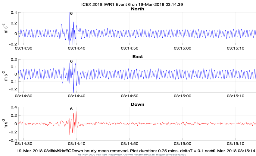
Figure 23. IWR1 ICEX2018 NED accelerations from Event 6 acquired near the airstrip. The vertical and horizontal accelerations due to planes landing on the ice are well above background values.
