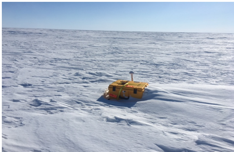
Figure 8. First IWR deployment on Elson Lagoon (December 2016) with an external antenna and ratchet straps to secure to the ice.
