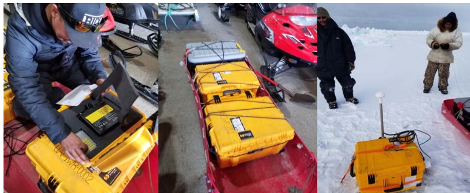
Figure 17. UIC personnel arming Able before deployment (left), IWRs loaded on sled for transport (center), and IWR deployed on Chukchi Sea landfast ice (right).
