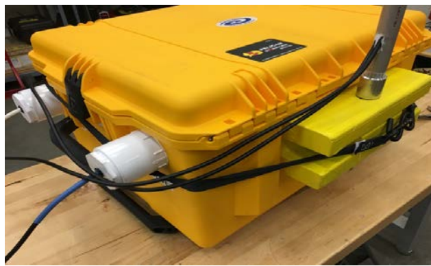
Figure 7. White PVC caps protect the antenna connectors that pass through the Pelican case to the external antenna.
