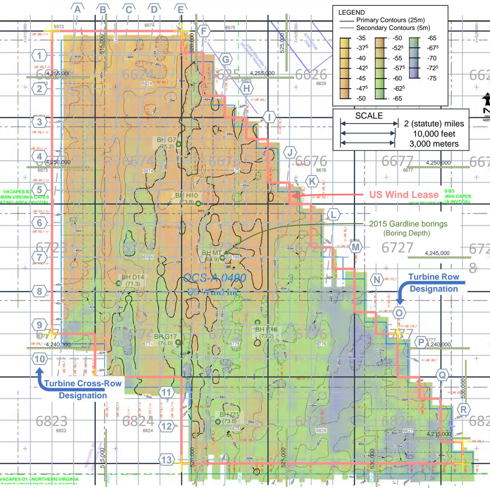
**STRUCTURAL CONTOURS on OCEANEERING CHANNEL BASE HORIZON**
