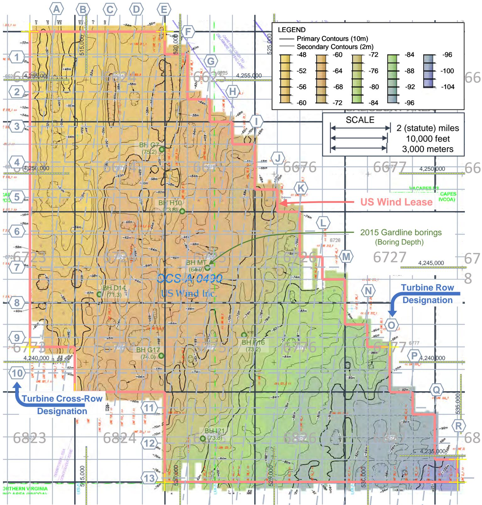
**STRUCTURAL CONTOURS on OCEANEERING HORIZON B**
