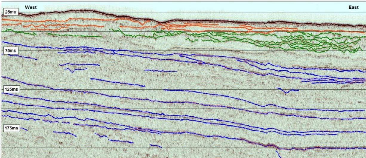
**Figure 46: Multi-channel seismic amplitude record for Line 315. Structurally relevant seismic horizons have been traced within the three general Seismic Facies Units identified. Reflectors within Seismic Facies Units 1, 2, and 3 are shown in orange, green and blue, respectively.**
