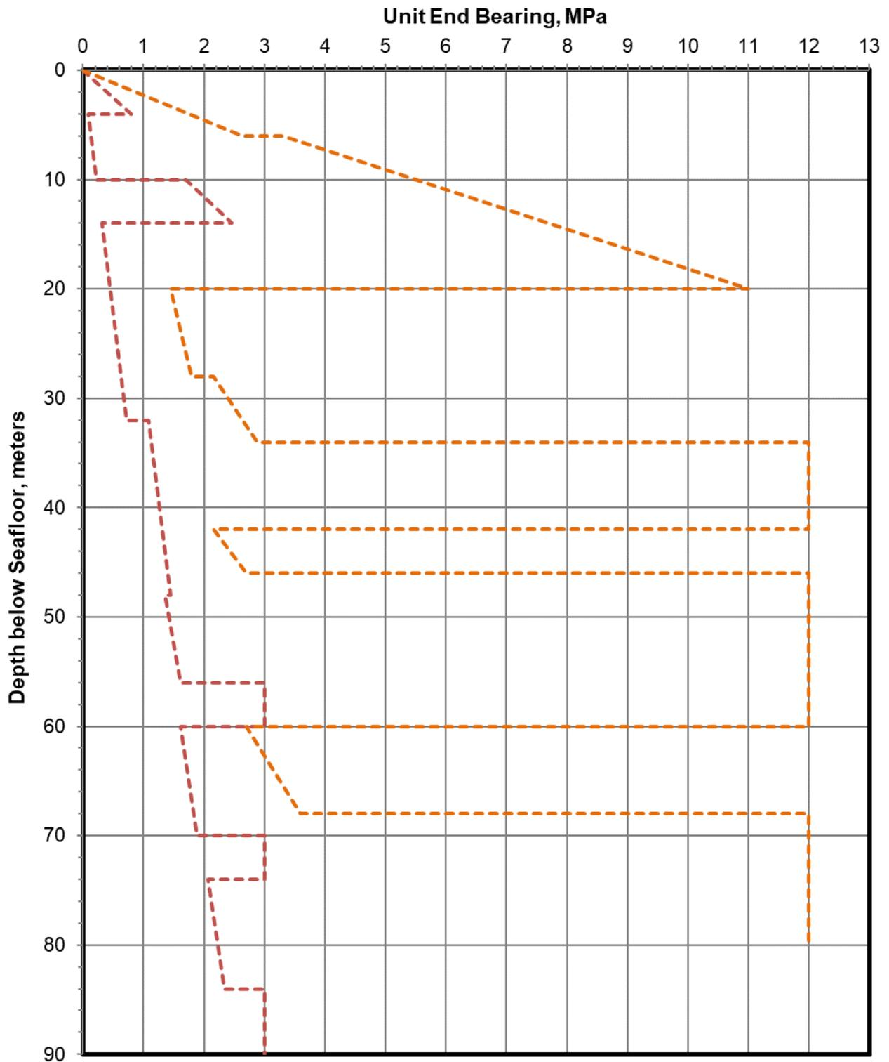
**ULTIMATE AXIAL PILE CAPACITY – UNIT END BEARING**
