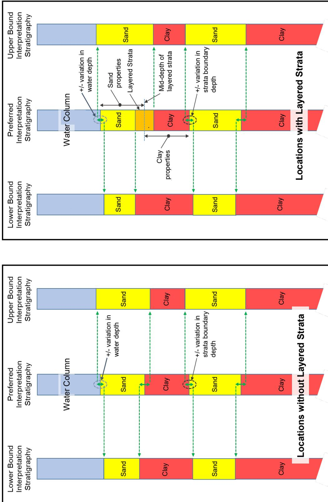
NOTE: Foundation Designer should verify that the different combinations of water depth, stratigraphy, and soil parameters as defined for the Lower & Upper Bound Conditions combine to produce weakest/softest or strongest/stiffest responses as intended for their design-specific analyses - particularly at low overburden (low stress) conditions.
