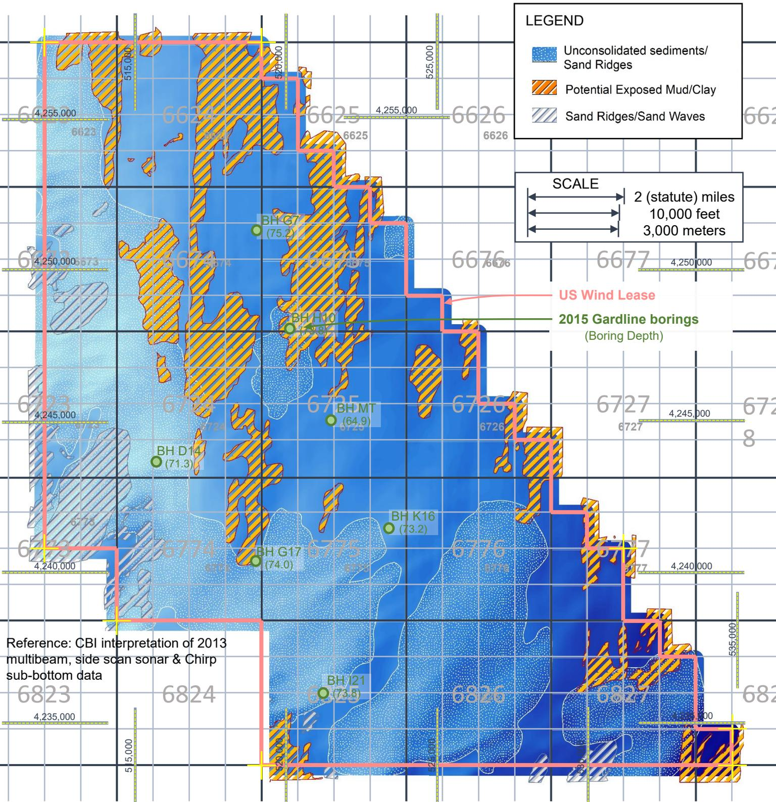
Reference: CBI interpretation of 2013 multibeam, side scan sonar & Chirp sub-bottom data
