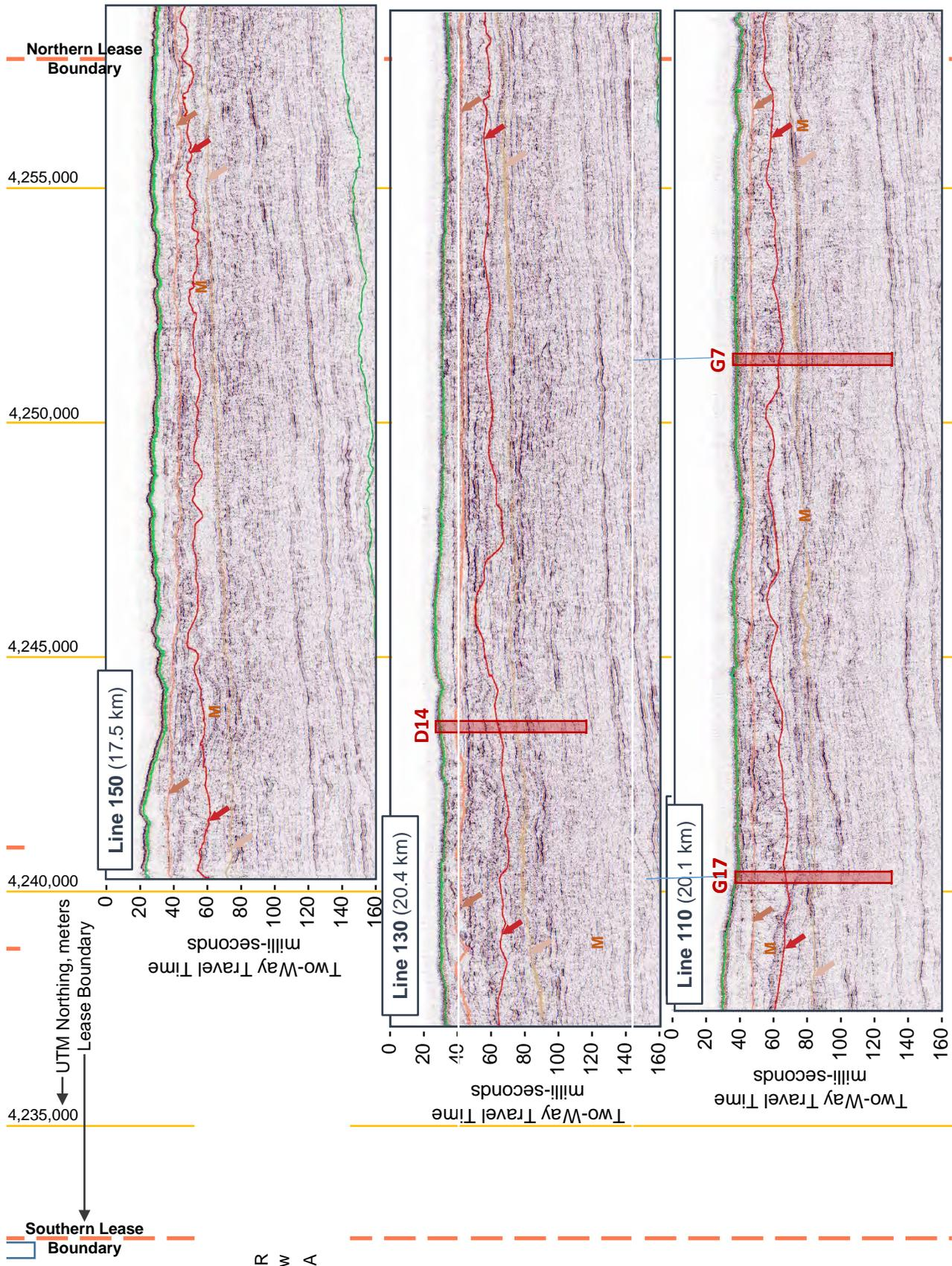
**NORTH – SOUTH MID-PENETRATION, SEISMIC REFLECTION RECORDS**
