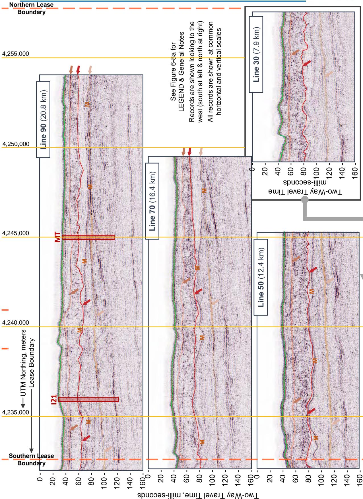
**NORTH – SOUTH MID-PENETRATION, SEISMIC REFLECTION RECORDS**
