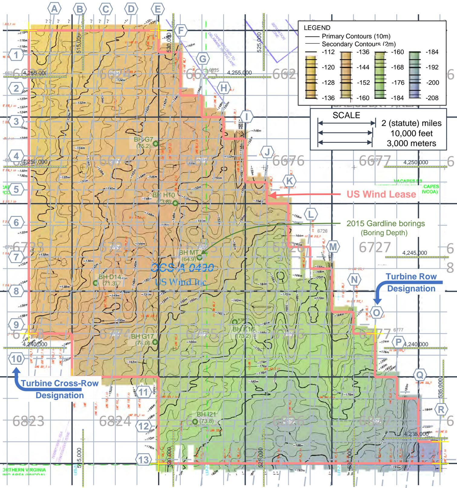
**STRUCTURAL CONTOURS on OCEANEERING HORIZON C**
