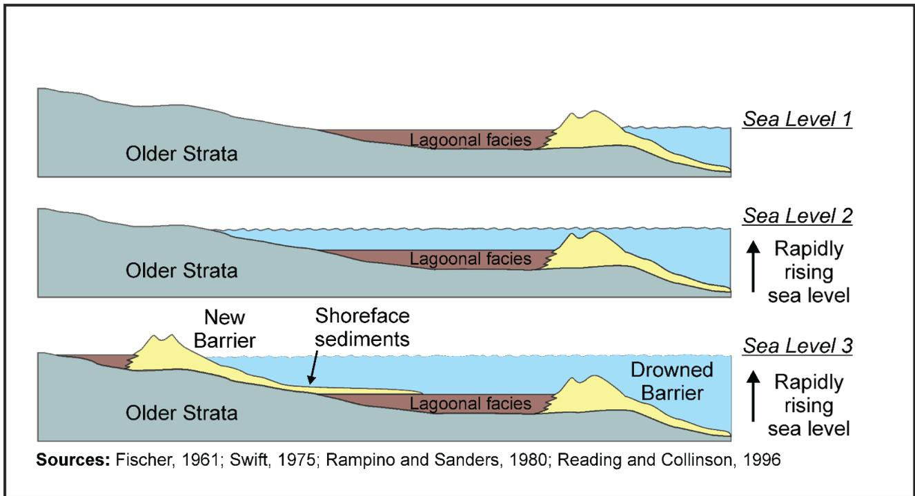
Schematic examples of barrier island evolution during slowly rising and rapidly rising sea levels are shown in the two geologic sketches shown above.
