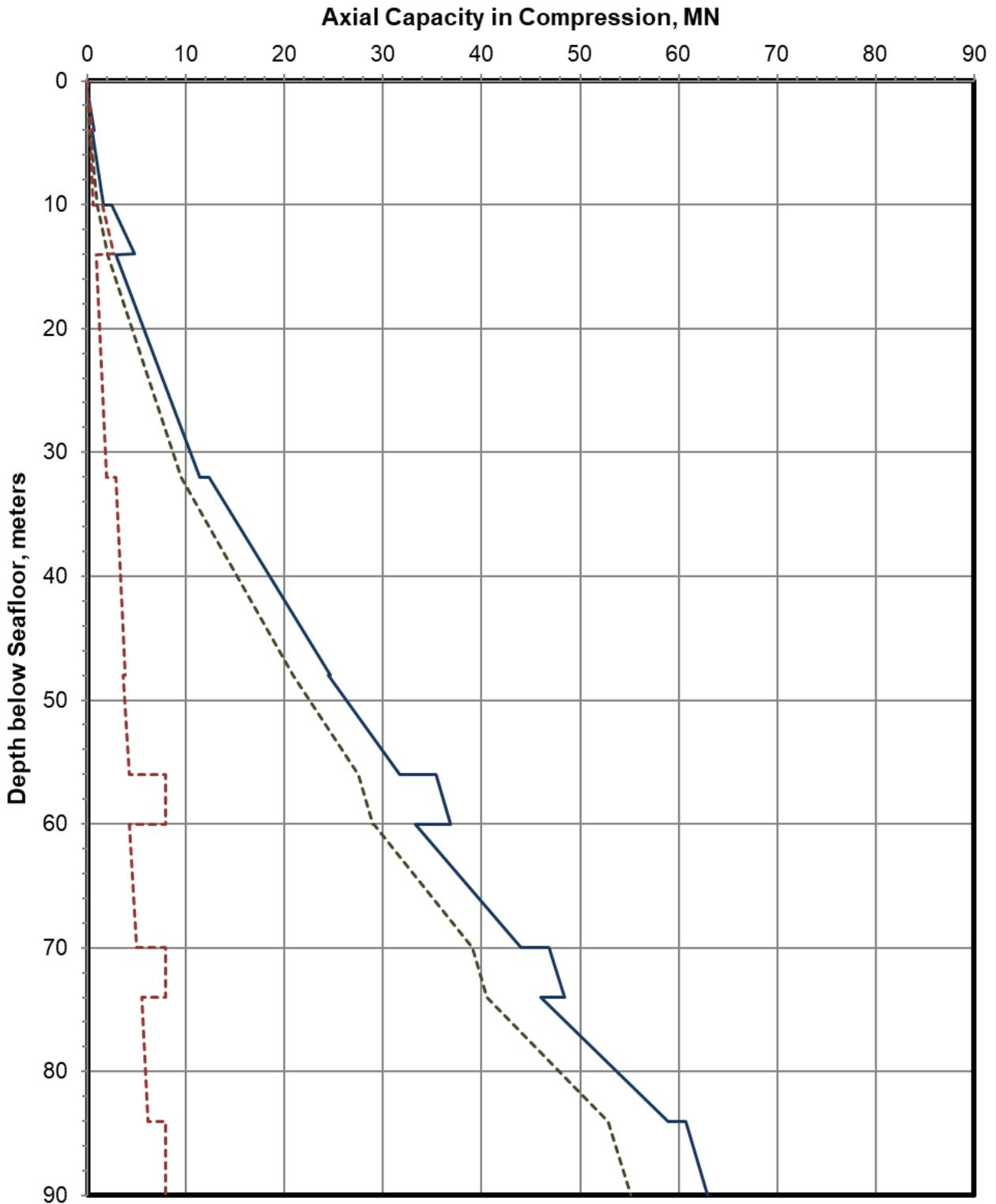
**ULTIMATE AXIAL PILE CAPACITY – GLOBAL LOWER-BOUND CONDITIONS**
