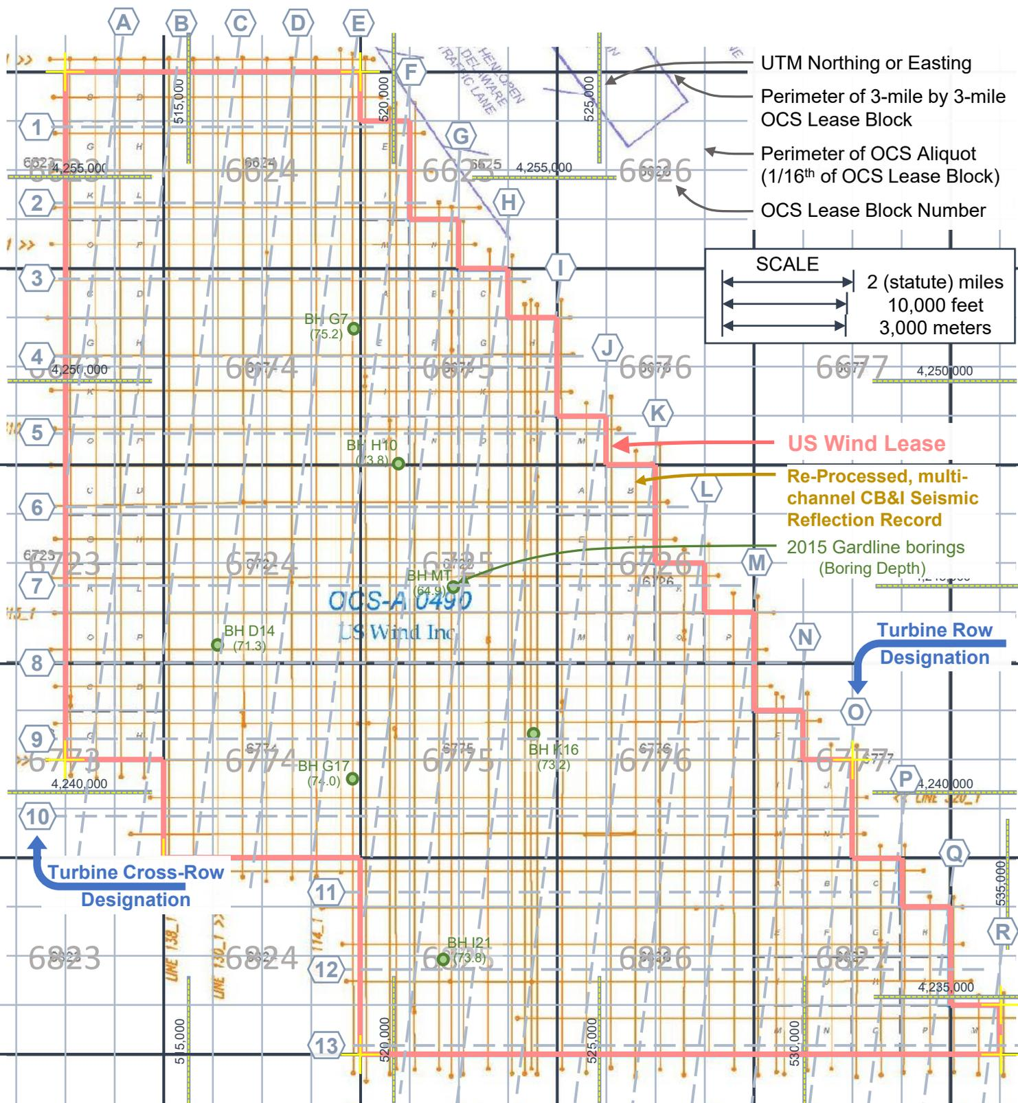
**REPROCESSED, CB&I 2013 M-C SEISMIC REFLECTION LINES**
