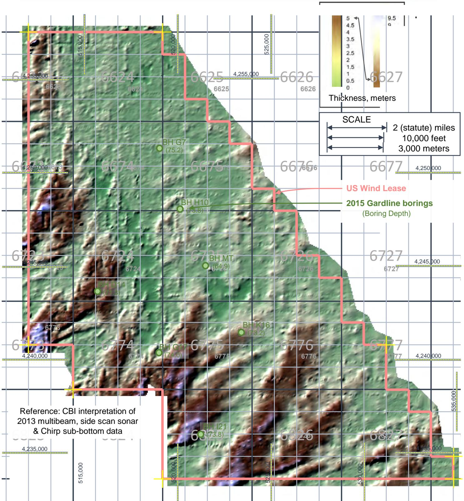
**ISOPACH (THICKNESS) OF SURFICIAL, HOLOCENE SEDIMENTS**
