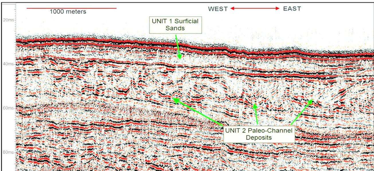
Figure 42: Portion of multi-channel sparker seismic Line 306 showing Pleistocene paleochannel complexes within Unit 2 overlain by the more recent (likely Holocene) sands of Unit 1.
