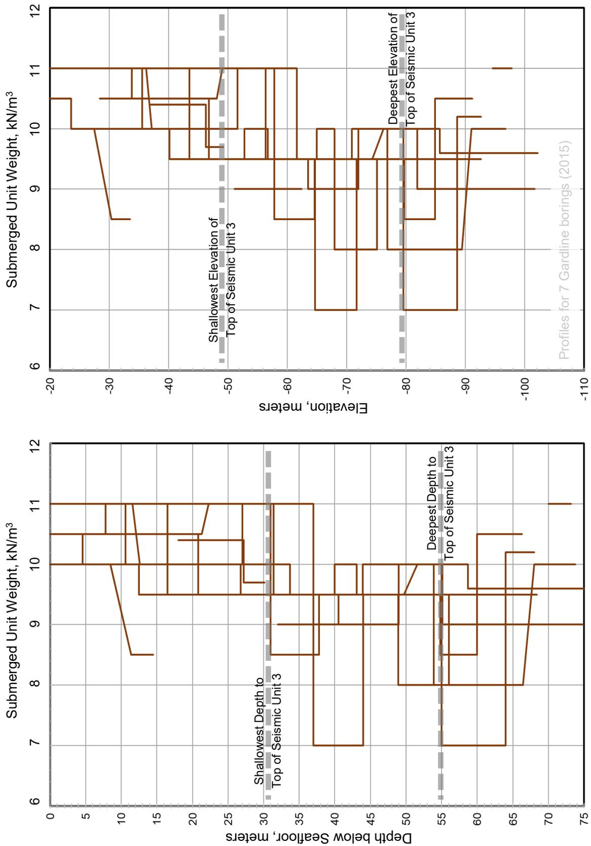
**INTERPRETED SUBMERGED UNIT WEIGHT PROFILES**
