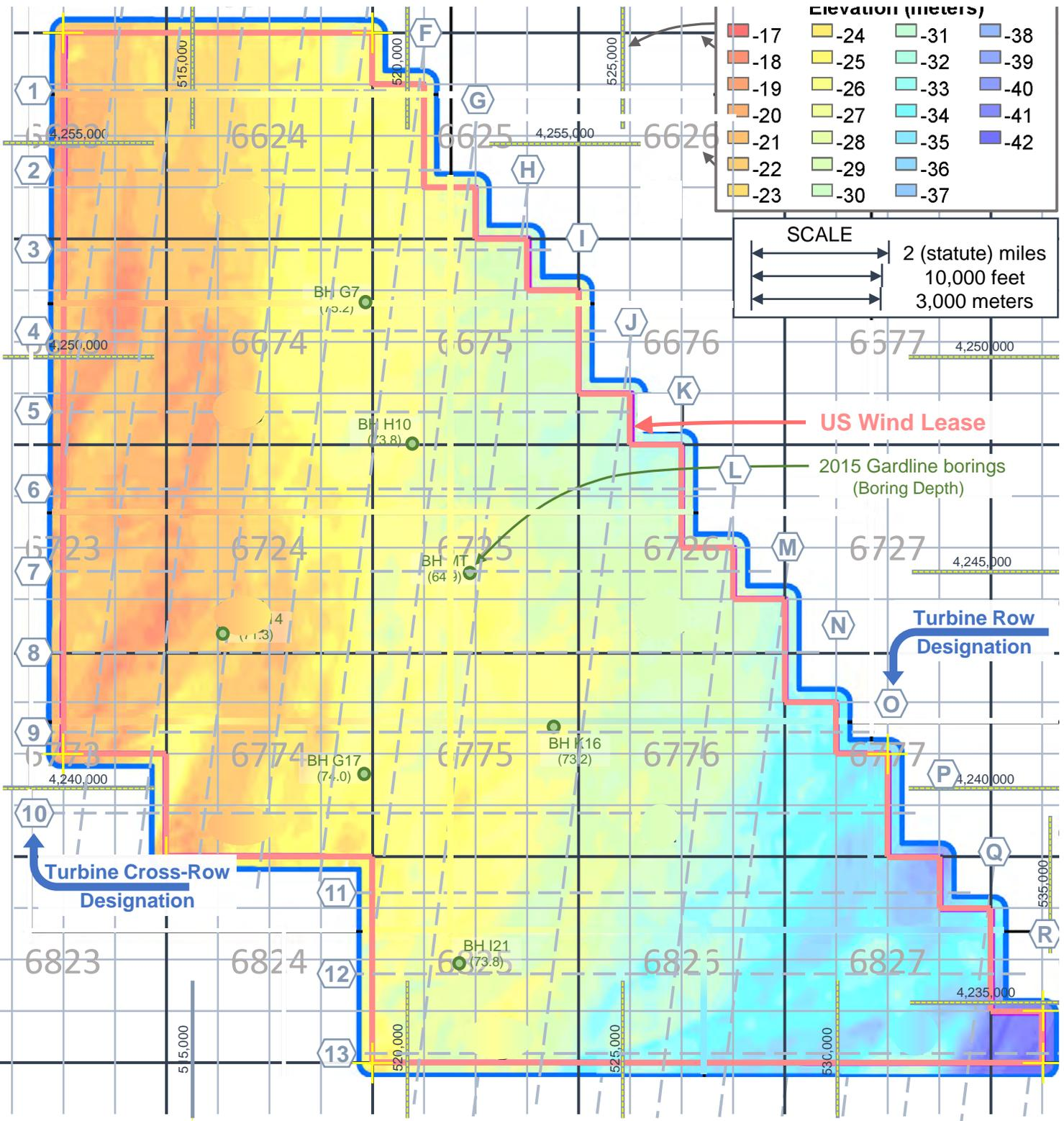
**STRUCTURAL CONTOURS on CB&I's BASE OF SURFACE SEDIMENTS**
