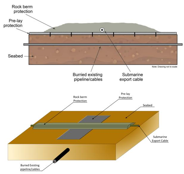
Figure 3.4-3 Typical Cable Crossing Design
