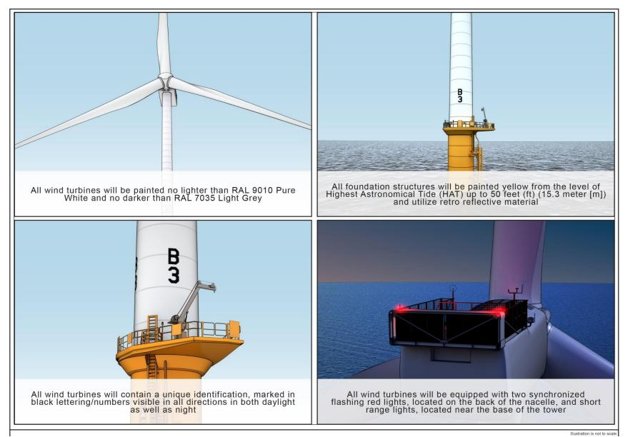
Figure 3.5-2 Paint Color and Marking Requirements for Wind Turbines
