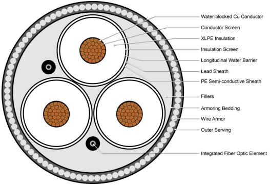
Figure 3.3-6 Representative Cross-Section of Submarine Export Cable
