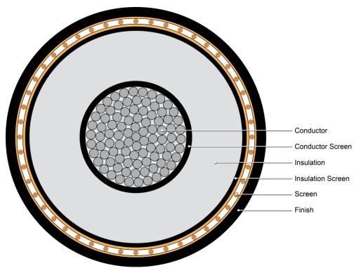
Figure 3.3-16 Representative Cross-Section of Onshore Interconnection Cable
