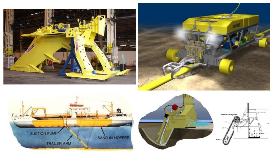
Figure 3.4-2 Examples of Cable Installation Methods
