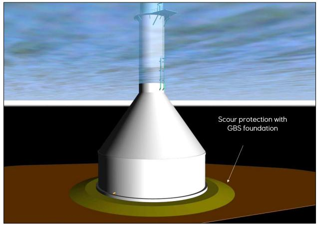
Figure 3.3-9 Example of Scour Protection Installation for GBS Foundation
