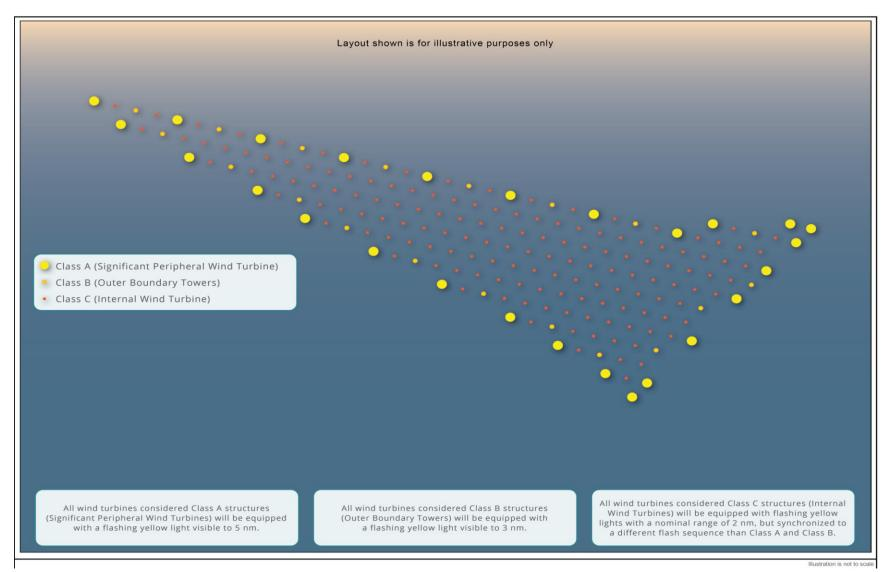
Figure 3.5-1 Navigation Lighting Requirements for Wind Turbines
