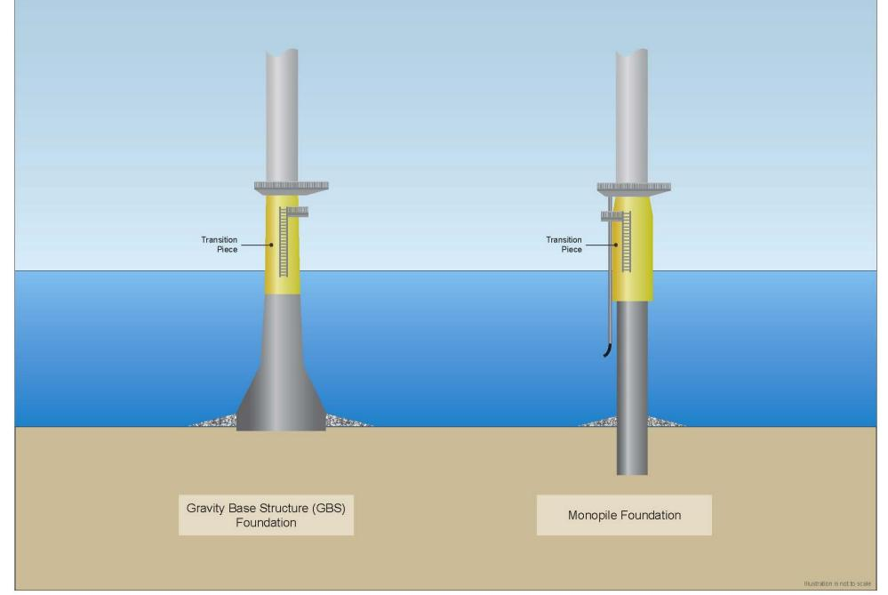
Figure 3.3-3 Wind Turbine Foundation Types
