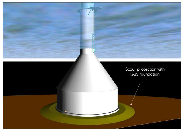
Figure 3.3-10 Example of Scour Protection Installation for GBS Foundation
