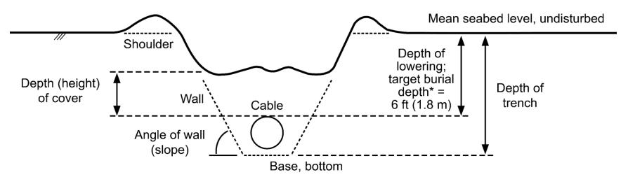
\*Note: Target burial depth will be 15 ft (4.7 m) below the current (and future) authorized depth or depth of existing seabed (whichever is deeper) in federally maintained navigation features (e.g., anchorages and shipping channels).
