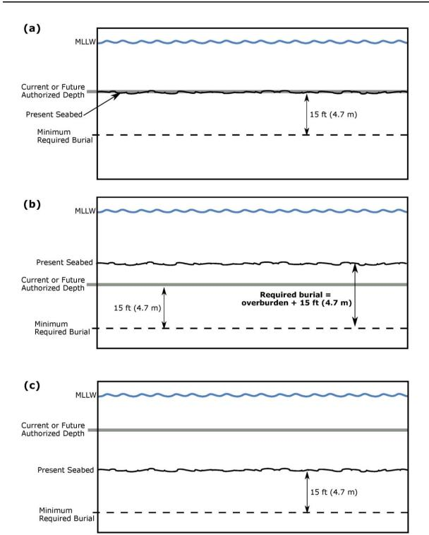
Figure 3.3-8 Diagrammatic representation of USACE minimum cable burial requirements for works within federal navigation projects (including their associated side slopes, based on guidance provided by USACE in a letter dated September 20, 2018) when (a) present seabed and authorized depth are the same; (b) authorized depth is deeper than present seabed; and (c) present seabed is deeper than authorized depth.
