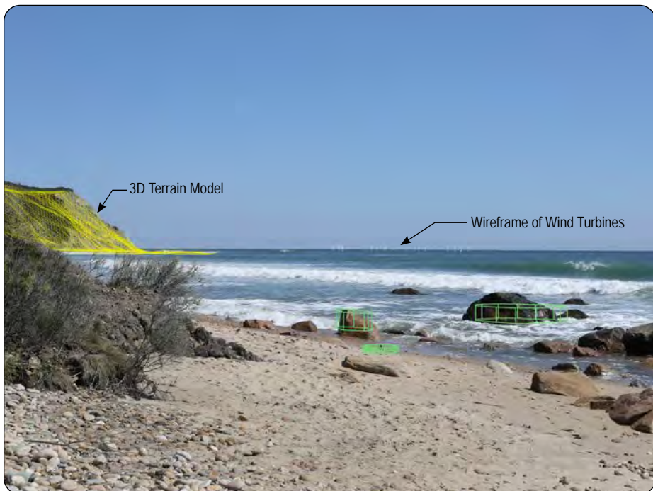
4. These data are superimposed over photographs from each of the viewpoints, and minor camera changes are made to align all known reference points within the view.
