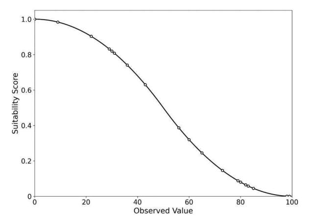
**Figure 2.5.** Example of hypothetical Z-shaped membership function, with the minimum observed value being 0 and the maximum observed value being 99. However, the total range of
