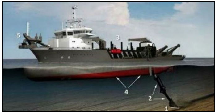
Figure B.3.2-4. Seafloor Disturbance from a Trailing Suction Hopper Dredge (TSHD). (The TSHD components include a draghead (1), on the end of a large suction pipe (2) through which large centrifugal pumps transport the dredged material as a slurry to the hopper (3) from where it is later discharged either through bottom doors (4) or pumped (5) through a pipeline from the bow.) (Michel et al. 2013).
