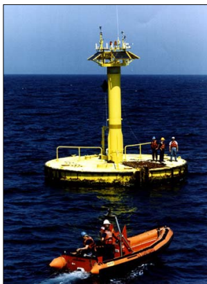
Figure A.4-2. 10-Meter Discus-Shaped Hull Buoy (Source: National Data Buoy Center 2012).
