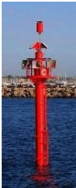
**Figure 2-5: Spar Buoy**
