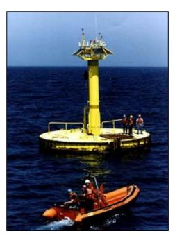
Figure 2-3: 10-m Discus-Shaped Hull Buoy Source: NDBC (2012)
