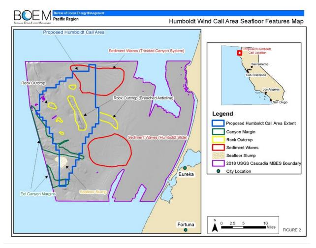
Figure 3-3: Humboldt Wind Energy Area Seafloor Features
