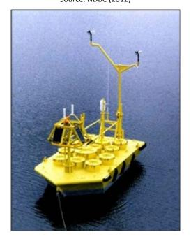
Figure 2-4: 6-m Boat-Shaped Hull Buoy Source: NDBC (2012)
