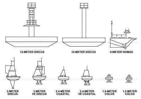
Figure 2-2: Buoy Schematic
