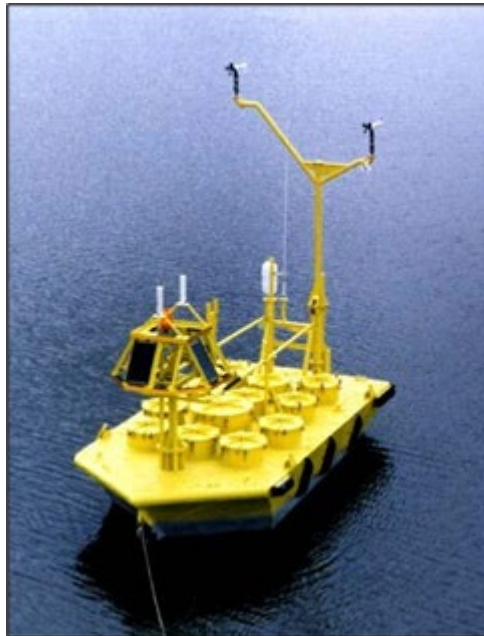
Figure 2-4: 6-m Boat-Shaped Hull Buoy
