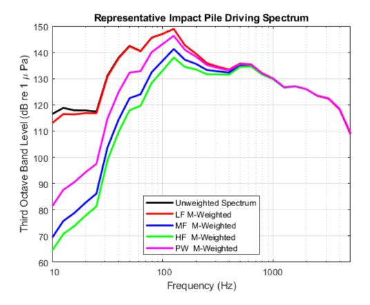
Figure 4. Representative spectrum measured from impact pile driving of a 7.8 m monopile
