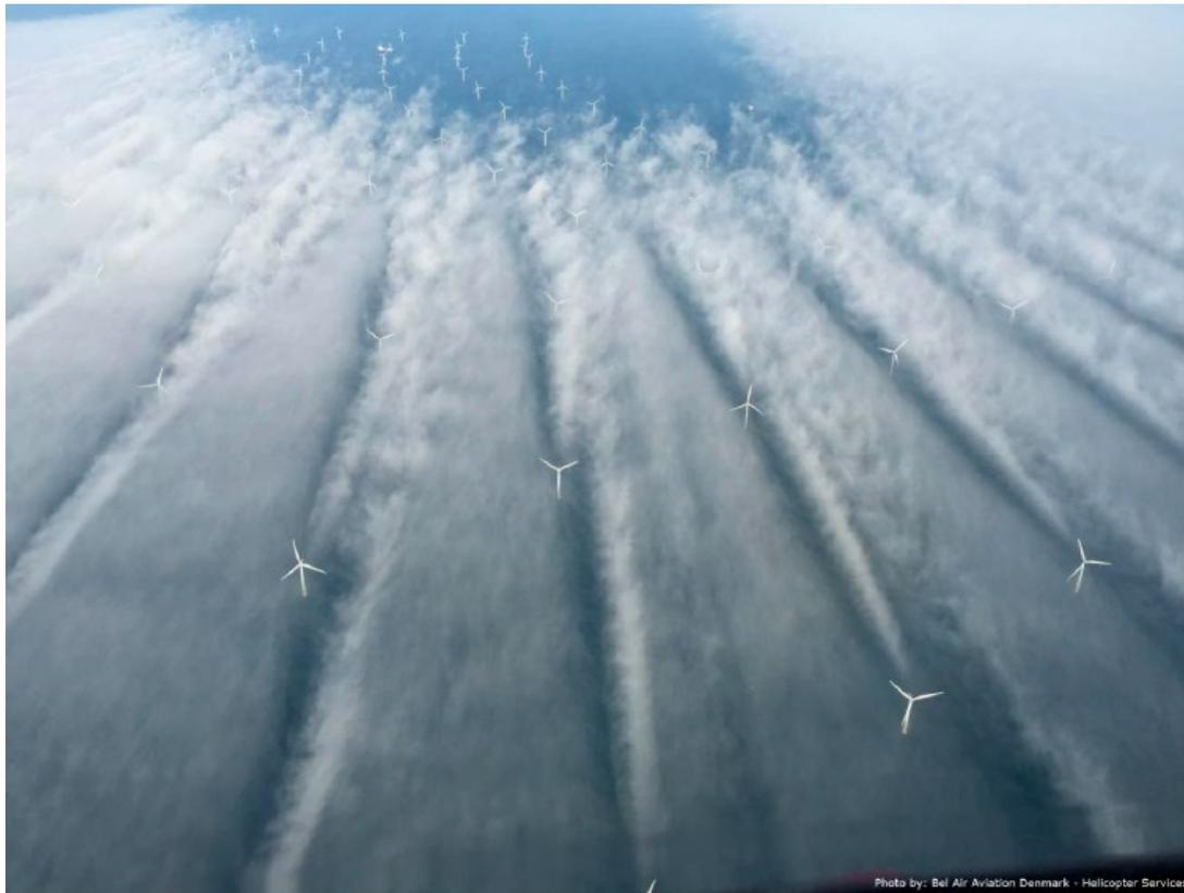
**Figure 2. Horns Rev 2 Visible Wakes**
