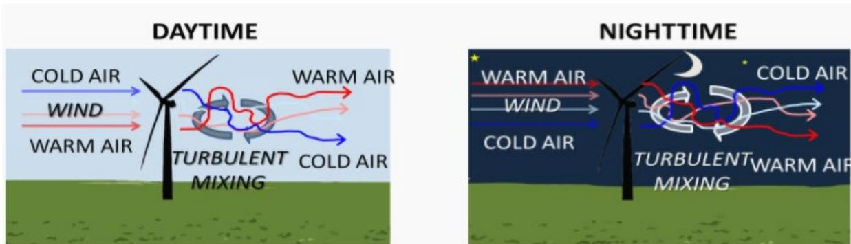
**Figure 3. Mixing of Air Layers – Day and Night**
