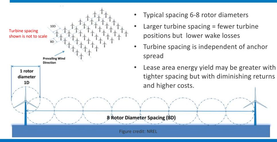
Example: GE 14-MW Haliade-X turbines with a 220-m rotor would be spaced over 1 mile apart
