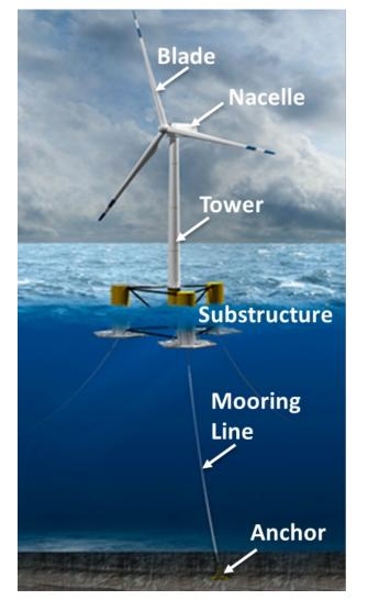
Parts of a Floating Offshore Wind Turbine NREL | 5
