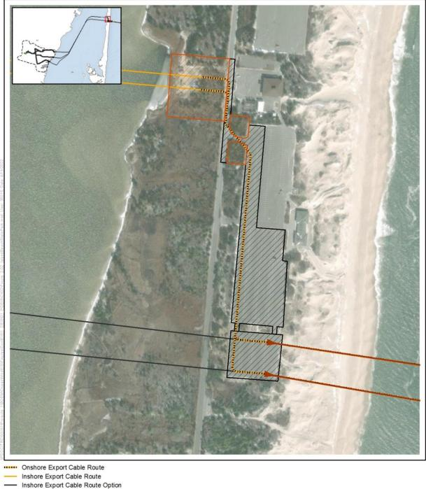
Inshore Export Cable F Temporary Work Area Work Area / Clearing HDD Duct Footprint
