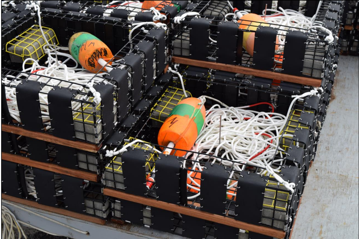
Figure 4.4-37. Conch (whelk) Pot Gear, Rigged Individually, Bricks Used to Keep Pot on Seabed
