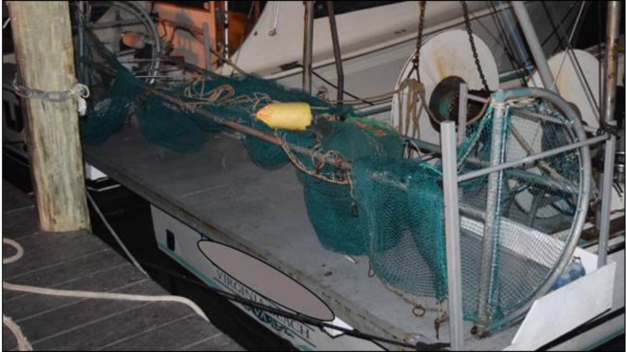
Figure 4.4-42. Beam Trawl, 16 feet in width, Secured to the Stern of a Fishing Vessel in Rudee Inlet
