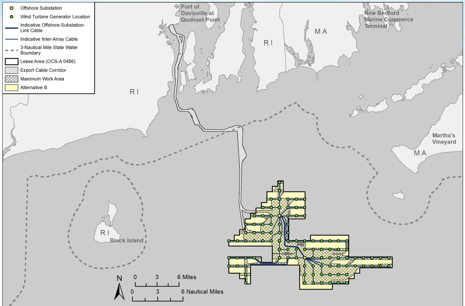
Offshore Project location and components under the Proposed Action.
