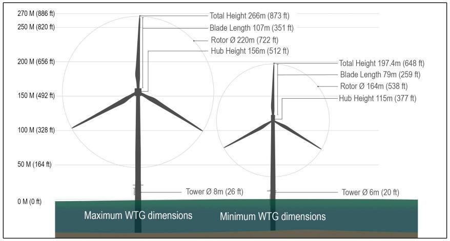
Figure 2.1-3. Wind turbine generator design envelope characteristics.
