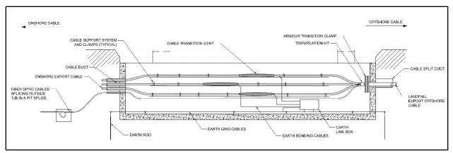
Figure 2.1-6. Transition joint bay and link box schematic (vhb 2022).
