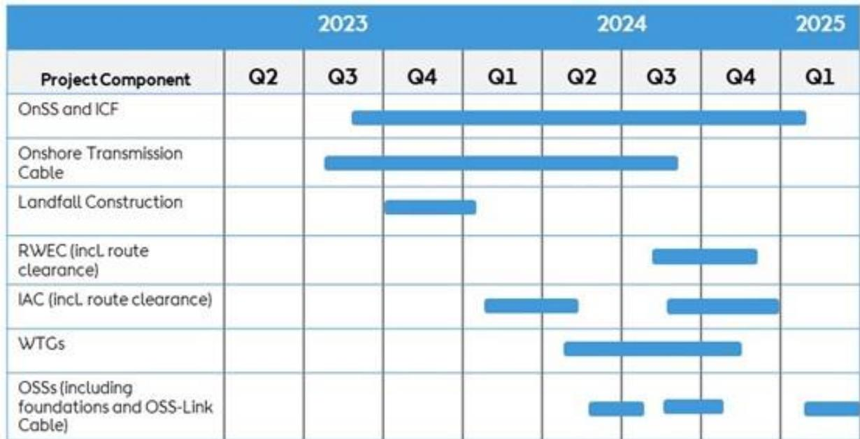
Figure 2.1-9. Revolution Wind Farm indicative construction schedule (VHB 2023).
