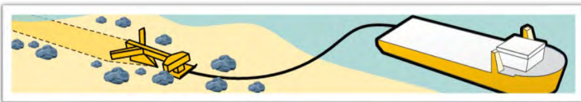
Figure 3.3.3-6 Typical Boulder Plow Configuration
