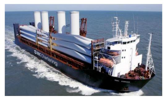
Figure 3-15. Tower Sections Onboard the BBC Chartering and Logistic Ship M/V BBC Konan¶ Source: gcaptain.com
