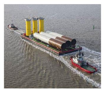
Figure 3-1. Tug and Barge Feeder System for Foundation Transportation Source: Wagenborg.com
