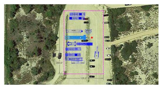
Figure 3-9. Approximate Footprint of HDD Drilling Operations at Landing Location
