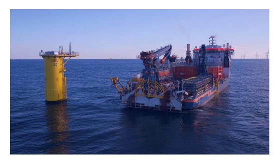
Figure 3-14. Dynamically Positioned Cable Installation Vessel¶ Source: Deutsche Bucht and Van Oord
