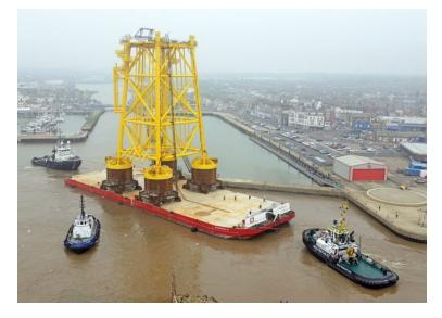
Figure 3-4. Jacket on Suction Bucket Transport¶Source: www.chpv.co.uk
